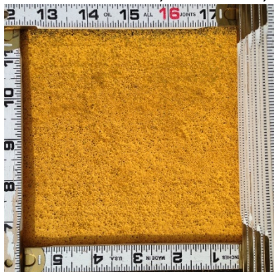
Recess Waterborne Paint, Installation, 4-0+00
