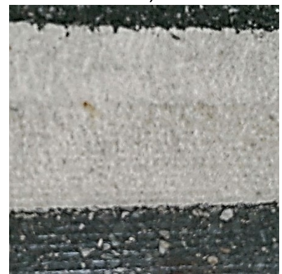
Recess Polyurea Wet Reflective, 36 months, 17-0+00
