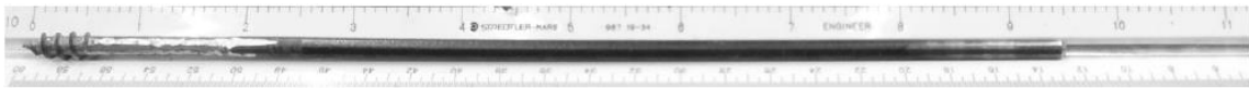
Figure 1. Drill bit used for checking decay created from a FastenMaster Headlok HLG M010 fastener. (Olszko and Bender 2015)
