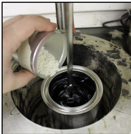
Figure 2.3. Sasobit® Being Mixed into Binder
