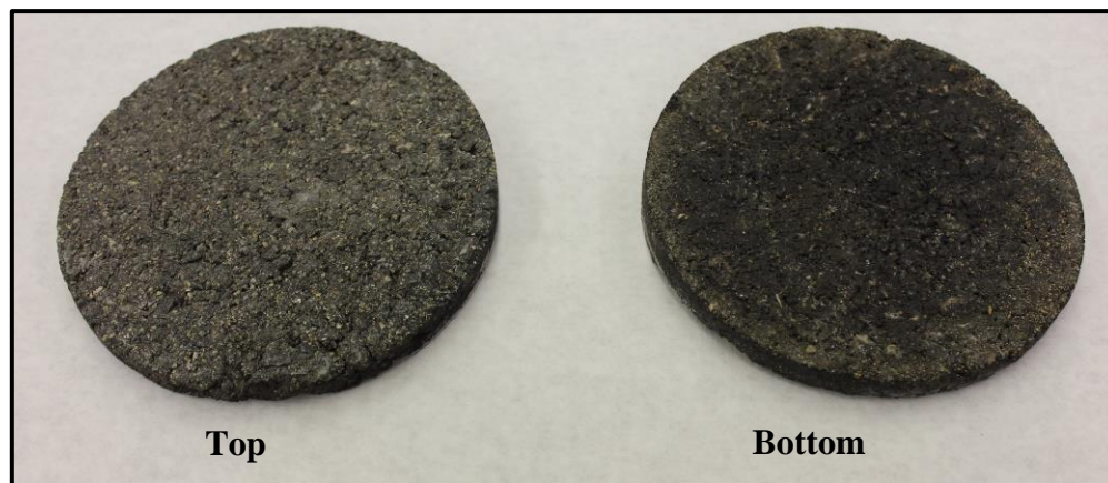
Figure 4.1. Photos of MAFB Core Slices Prior to Binder Recovery
