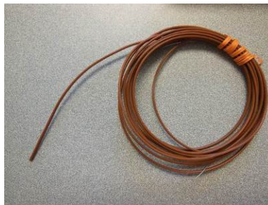
Figure 2 - Thermocouple used for concrete temperature measurement
