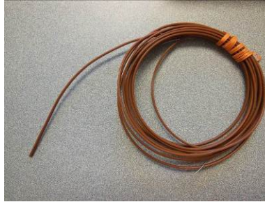
Figure 3.2. Thermocouple used for concrete temperature measurement
