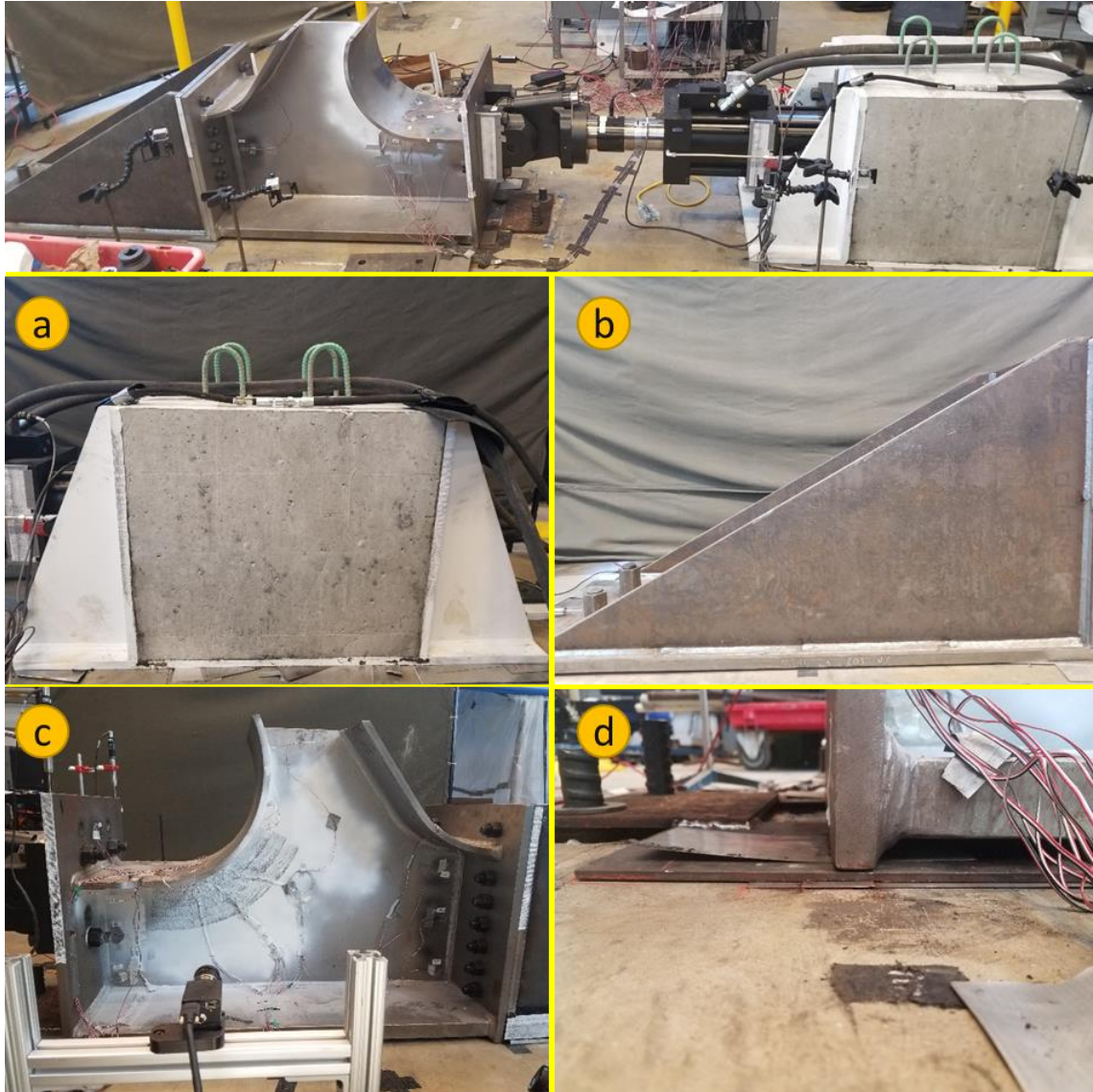
Figure 29 - System Components - Overall Test Setup, Reaction Block (a), Bracket Support (b), Specimen (c), and Shim Support (d)
