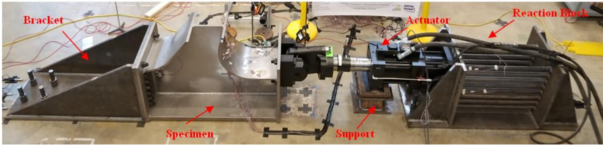
Figure 23 - Assembled Experimental Setup (without concrete poured on the reaction block)
