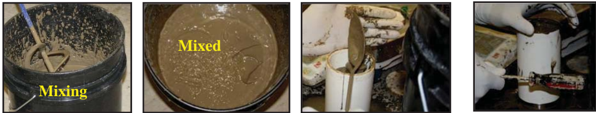
Figure 5.1. LC-VHMS Specimen Preparation-Portland vs. Slag/Portland Cement
