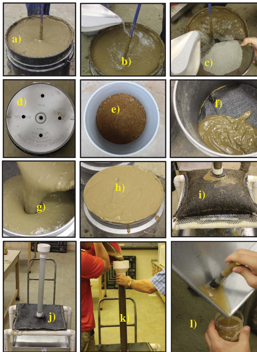
Figure 8.1. Vegetation Experiment Specimen Preparation: Buckets & Geotextile Pillows
