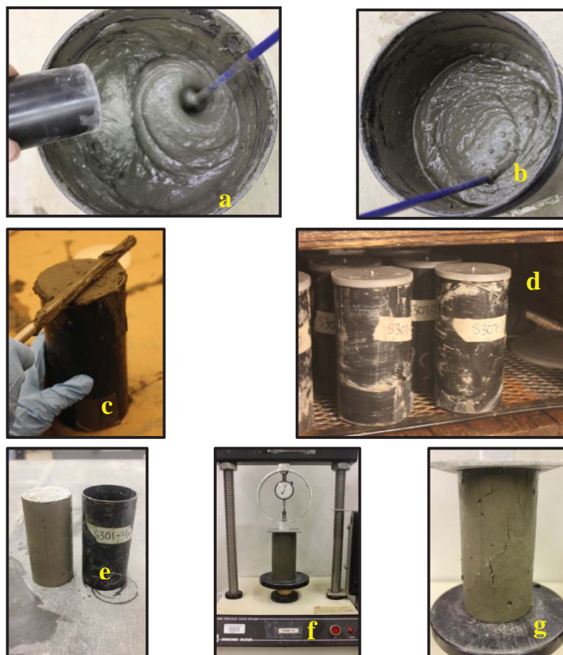
Figure 7.3. Specimen Fabrication, Curing, and Testing
