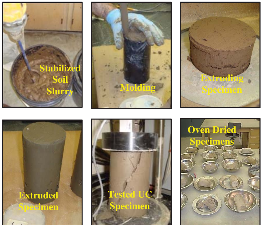
Figure 6.3. UC Specimen preparation and Testing
