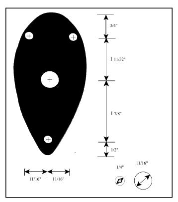
The large hole in the middle of the faceplate is for the BNC cable used to connect the antenna to the radio. The three 1/4" holes are for screws used to attach the antenna to the aircraft fuselage or skin-doubler.
