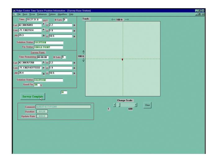
After "Survey Complete" appears on the data collection button, it is good practice to note the survey data on a log for archival purposes. The data appearing in the "Survey Point" portion of this screen at the end of the survey should be identical to that found in the appropriate 'SB' data file.
