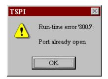
Possible Solution: Close out of TSPI software and re-invoke.
