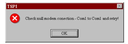
*Possible Solutions:* Check connection of null modem cable at both ends. Ensure serial port of computer is set to COM1, *not COM2*, etc.
