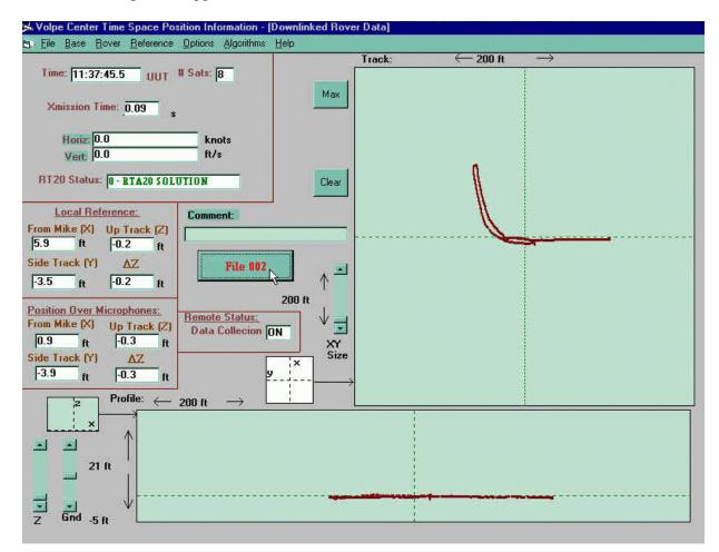
Click on "Collection Off" to begin collection of data at the remote site. The button then changes to "File xxx" where 'xxx' indicates the extension for the file currently being used for storing data.
