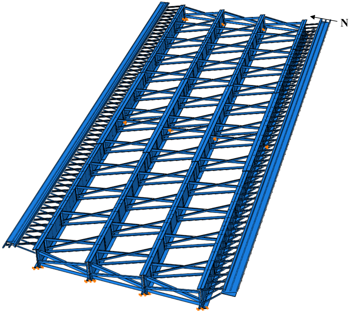
Figure 4: 3D FE Model Geometry of Skewed-Staggered Bridge Configuration
