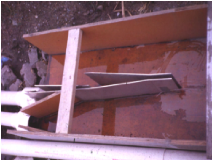
Figure 3.5 Diversion channel at downstream end of composite flow splitter
