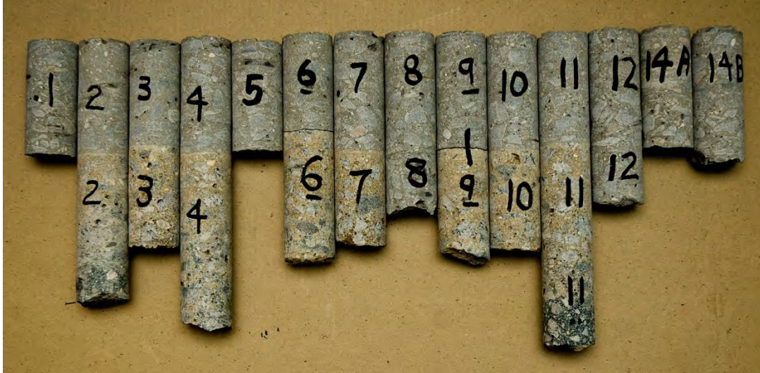
Figure 17. Cores to Verify Bond Strength and Thickness of Bonded Overlay
