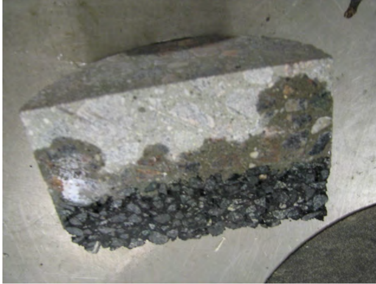
Figure 6. Slice From Mockup of a Hydraulic Cement Concrete Overlay Placed on a Porous Friction Course
