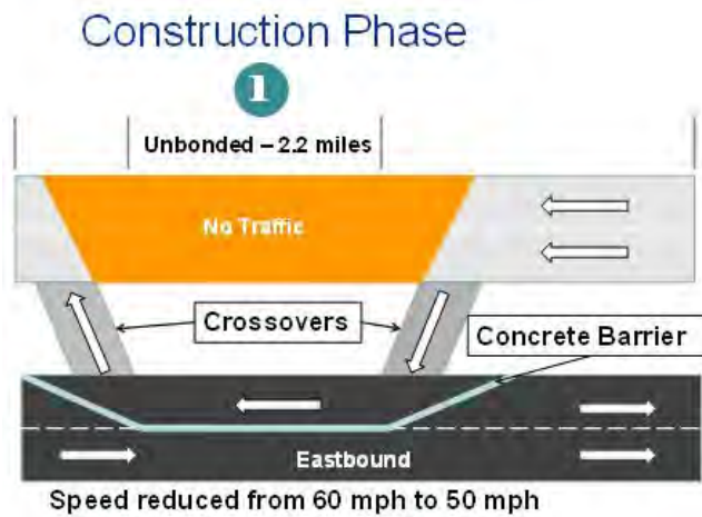
Figure 8. Phase 1 Crossovers. Unbonded = unbonded hydraulic cement concrete.
