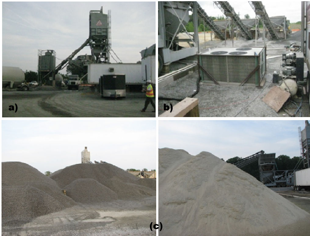
Figure 12. Concrete Plant: a) plant setup; b) chiller to cool the water; c) aggregate stockpile
