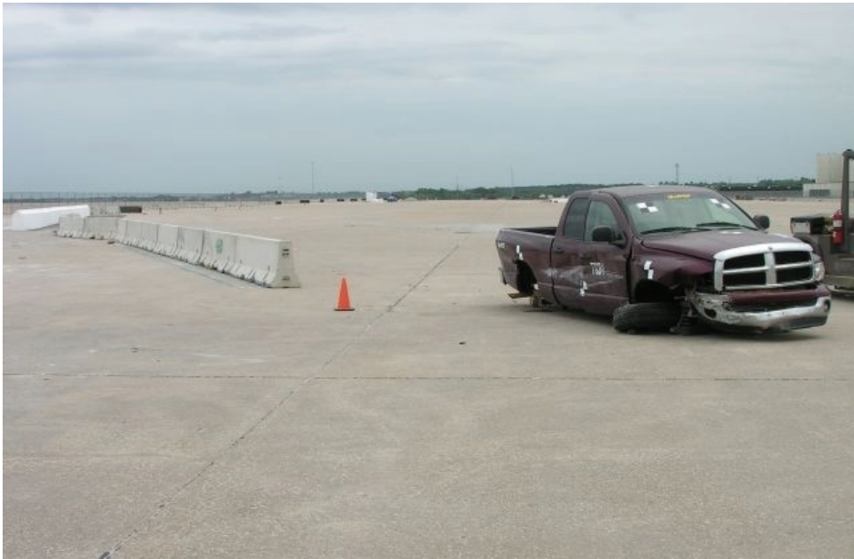
Figure 32. Vehicle Final Position and Trajectory Marks, Test No. TTCB-1
