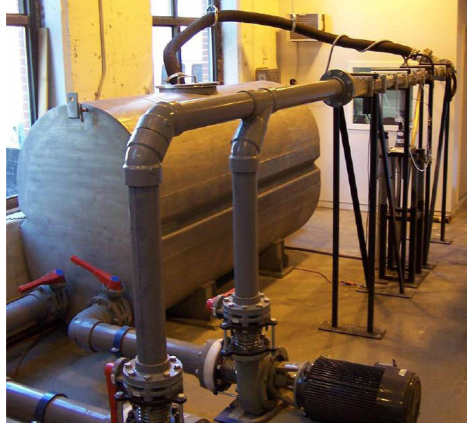
The SERF device is a unique device for testing shear-stress relationships of erodable materials.
