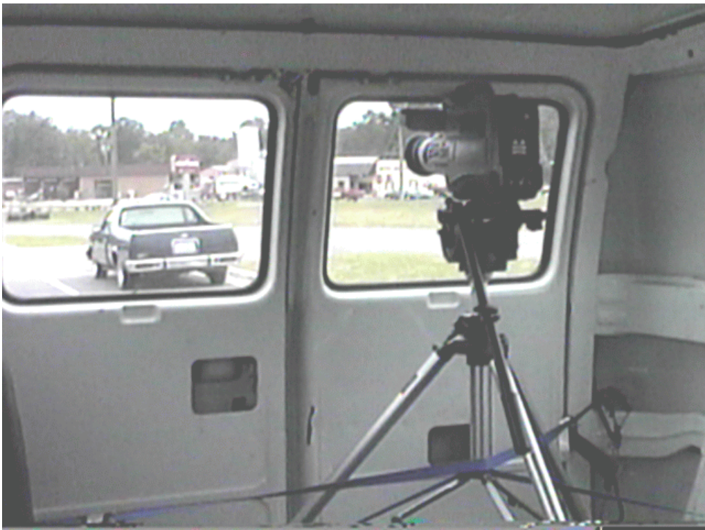
Figure 2 Setup and Positioning of the Rear Camera.
