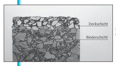
Figure 25. Twin-layer asphalt in Germany. (Photo Source: BASt, Germany)
