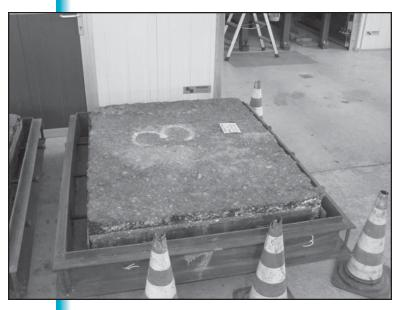
Figure 7. Block samples for accelerated loading facility testing in Denmark.
