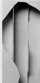
Competitor after a 2lb. weight was dropped 4 feet
