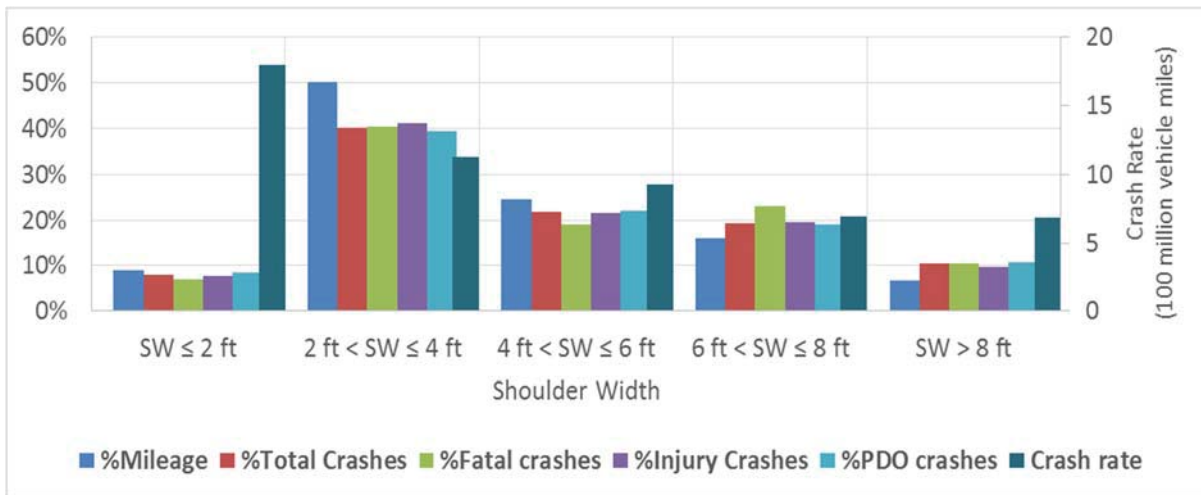
Figure 5 Mileage and crash severity distribution by shoulder width on rural 2-lane roadways
