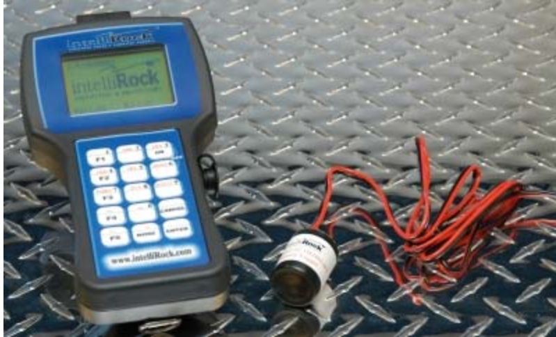
Figure 1 intelliRock II reader and logger
