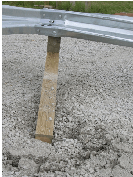
Figure 90. Post Nos. 6S through 8S Damage, Test SR-8
