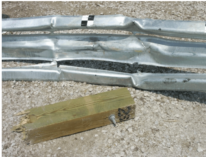
Figure 87. System Damage, Test SR-8
