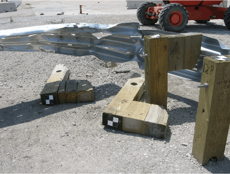
Figure 55. Post Nos. 6P through 9P Damage, Test SR-7
