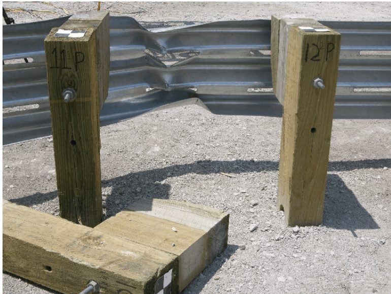
Figure 56. Post Nos. 11P through 13P Damage, Test SR-7
