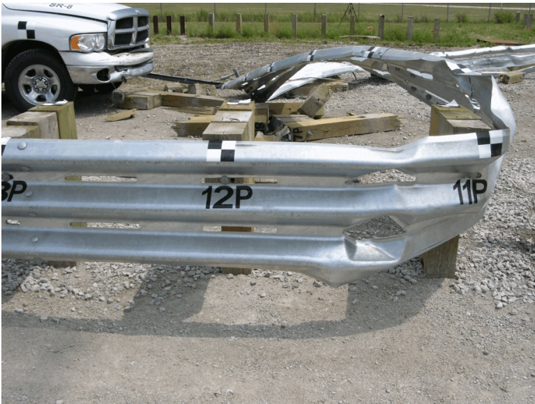
Figure 91. Post Nos. 1P through 12P Damage, Test SR-8
