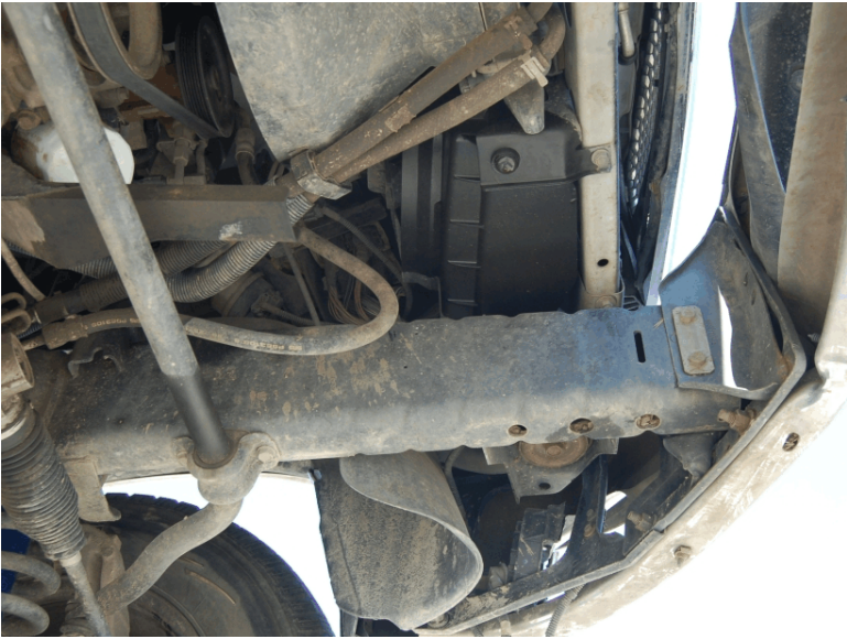
Figure 96. Undercarriage Damage, Test SR-8
