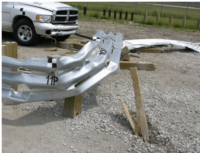
Figure 86. System Damage, Test SR-8
