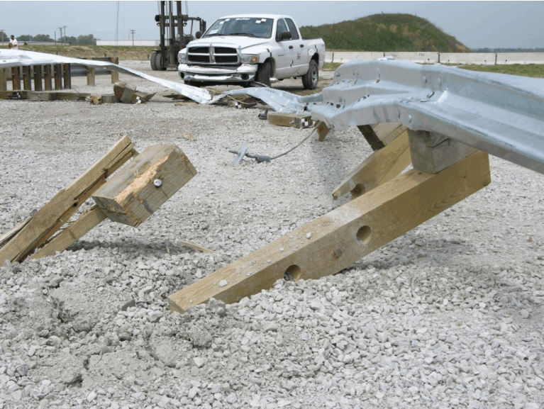
Figure 88. Secondary-Side Post Damage, Test SR-8
