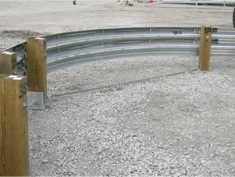
Figure 72. Nose and Plate Washer Details
