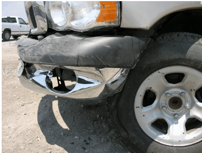
Figure 60. Vehicle Damage, Test SR-7
