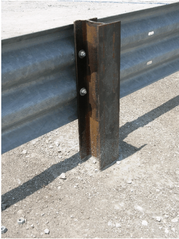
Figure 58. Post Nos. 20 and 21P Damage, Test SR-7
