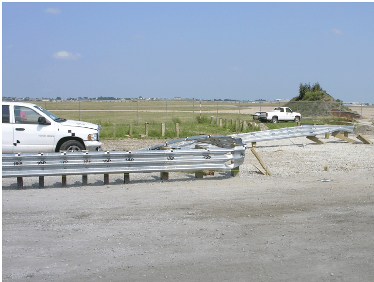
Figure 85. System Damage, Test SR-8
