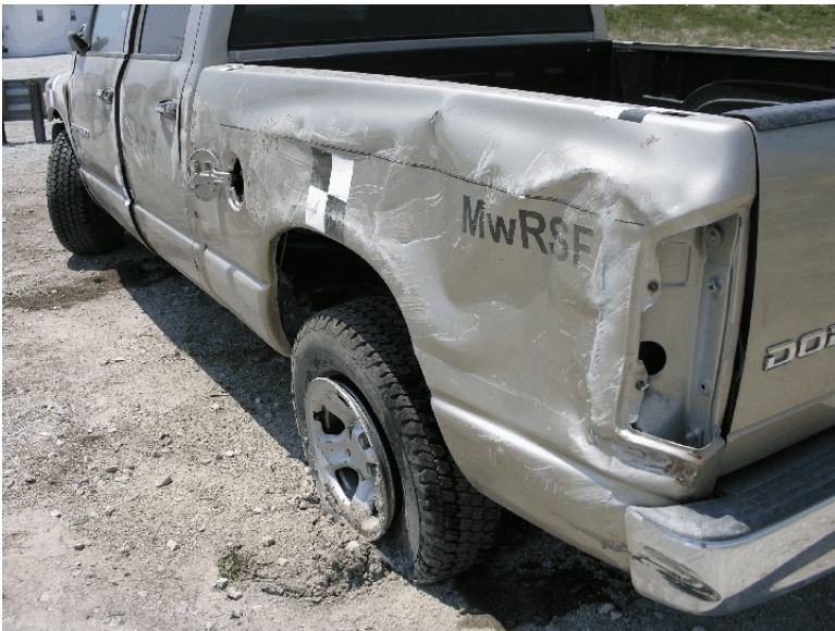
Figure 61. Vehicle Damage, Test SR-7
