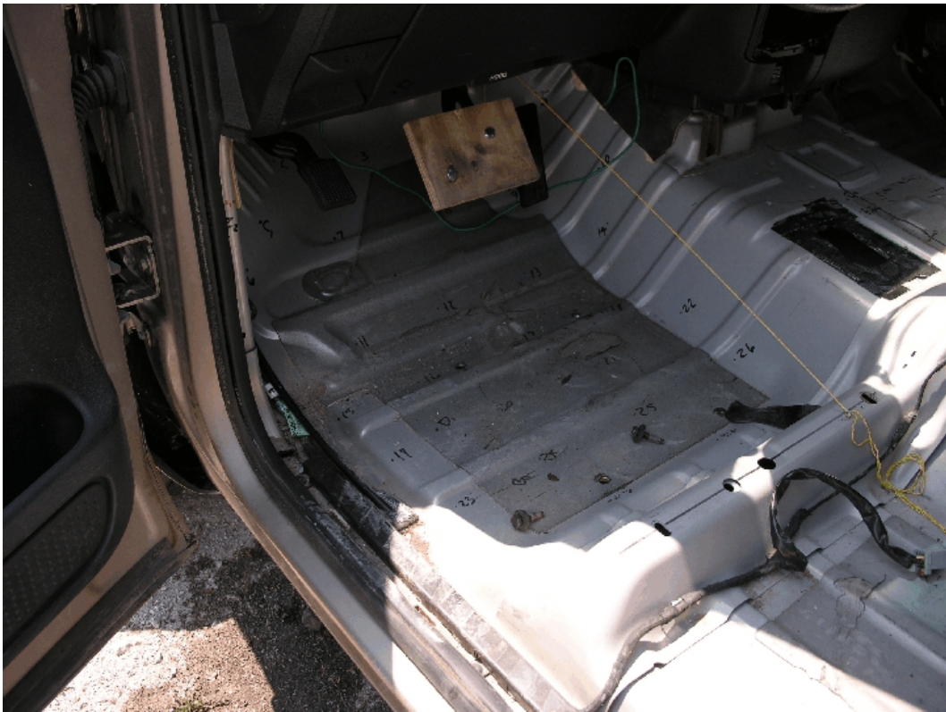
Figure 62. Occupant Compartment Deformation, Test SR-7
