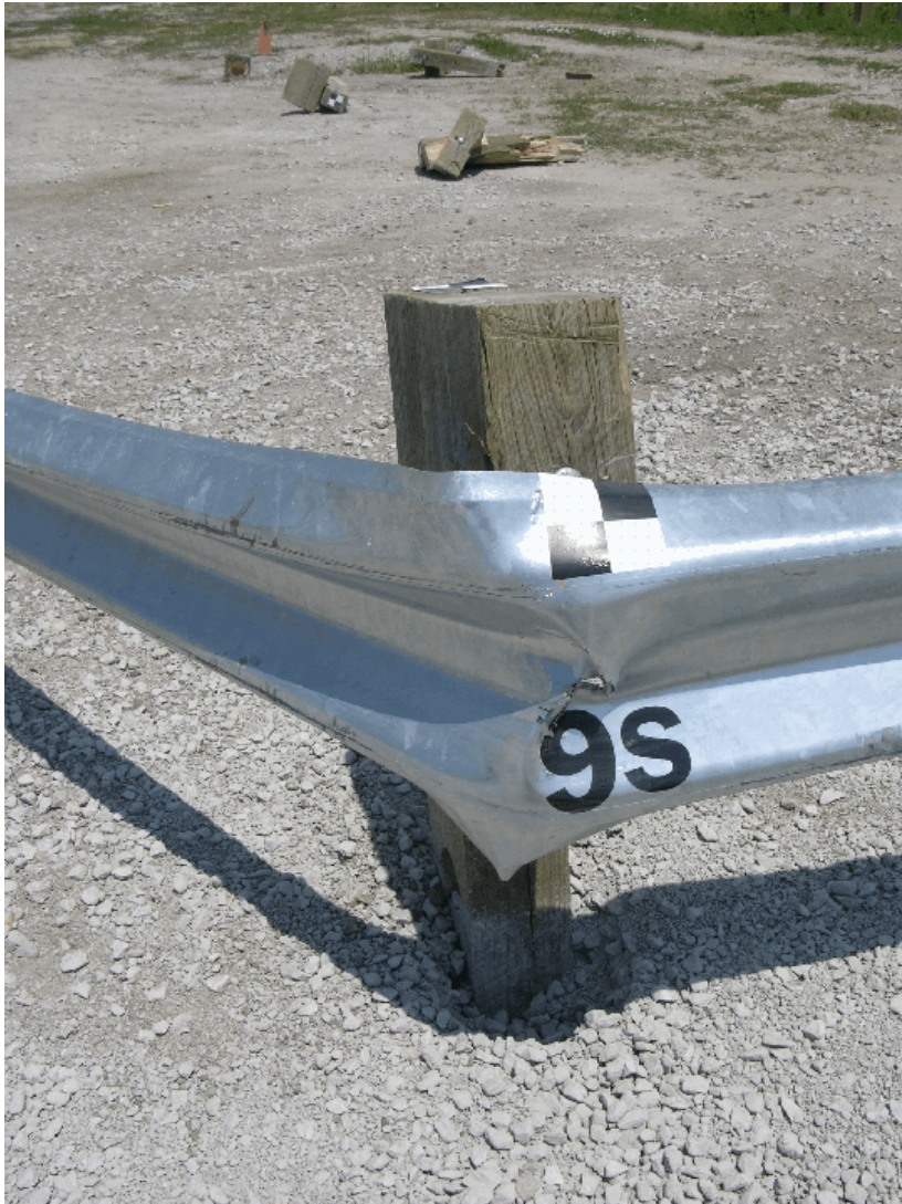
Figure 50. Post No. 9S Damage, Test SR-7
