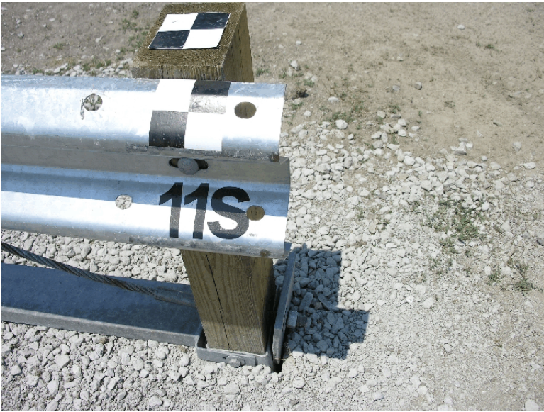
Figure 49. Post Nos. 10 and 11 Damage, Test SR-7
