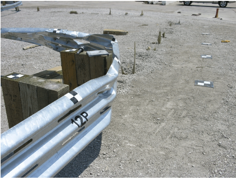
Figure 43. System Damage, Test SR-7
