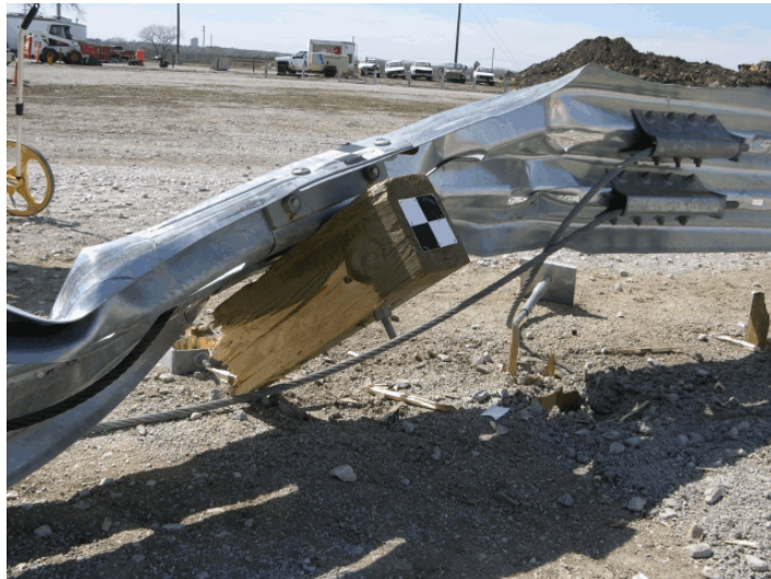
Figure 57. Post No. 1S Damage, Test SR-5
