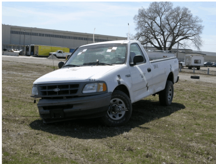
Figure 62. Vehicle Damage, Test SR-5
