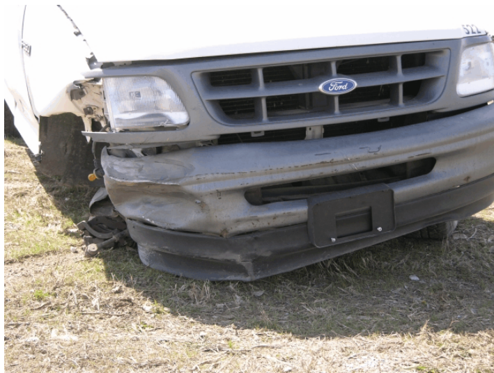
Figure 63. Vehicle Damage, Test SR-5
