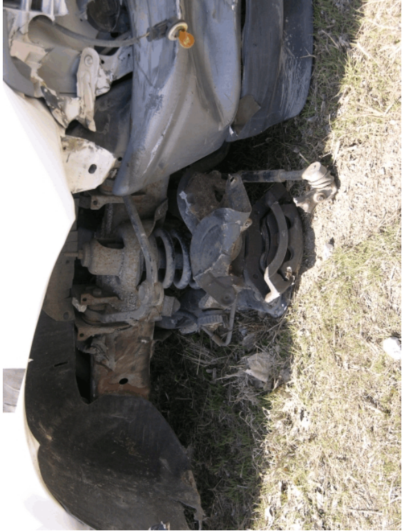
Figure 64. Vehicle Damage, Test SR-5
