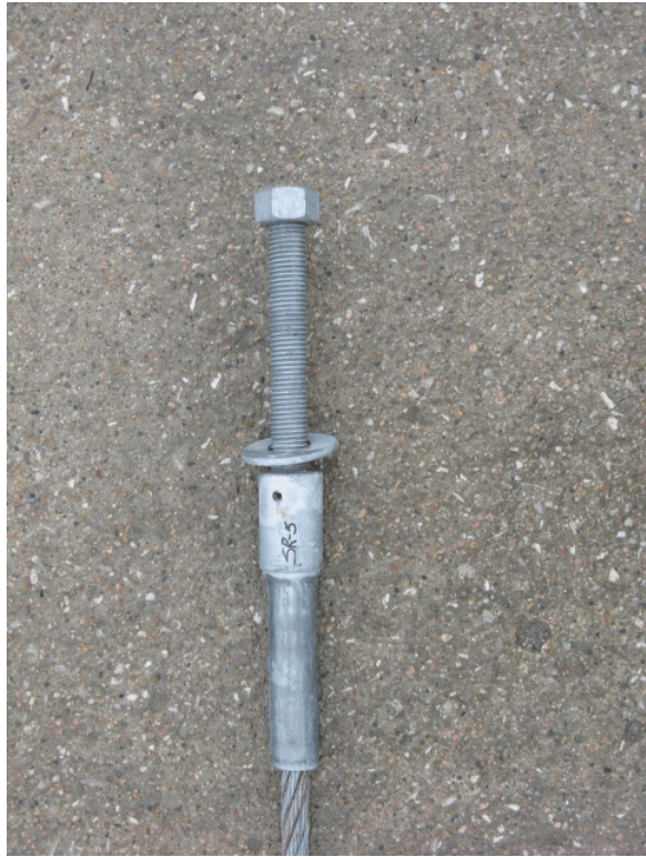
Figure 56. Nose Cable Damage, Test SR-5
