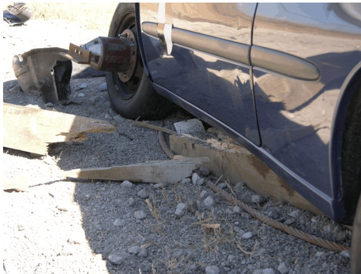
Figure 91. Post Nos. 1P through 6P Damage, Test SR-6
