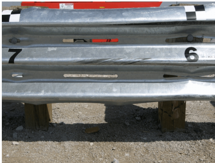
Figure 54. Rail Damage Between Post Nos. 3P through 7P, Test SR-5
