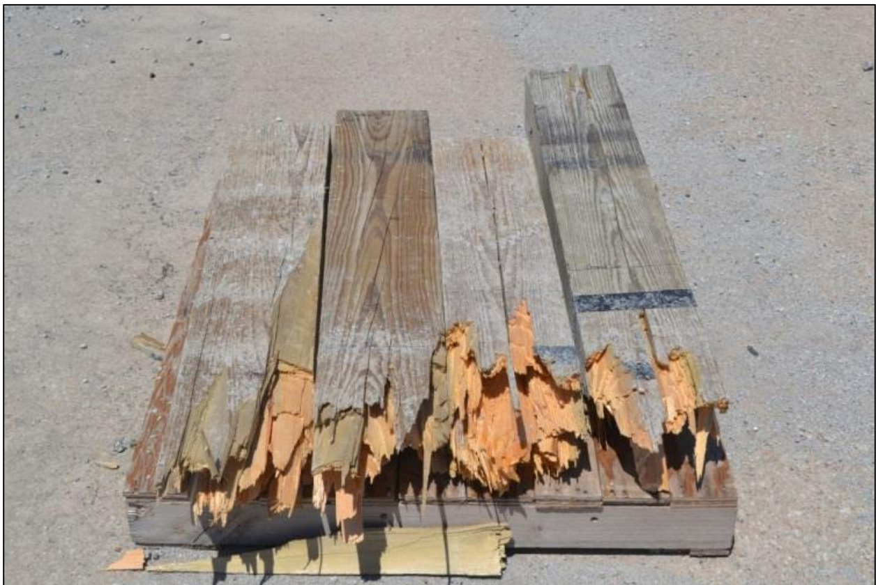
Figure 26. Comparison of Post Fractures, Test Nos. SYPW-1 (Left) and SYPW-4 (Right)
