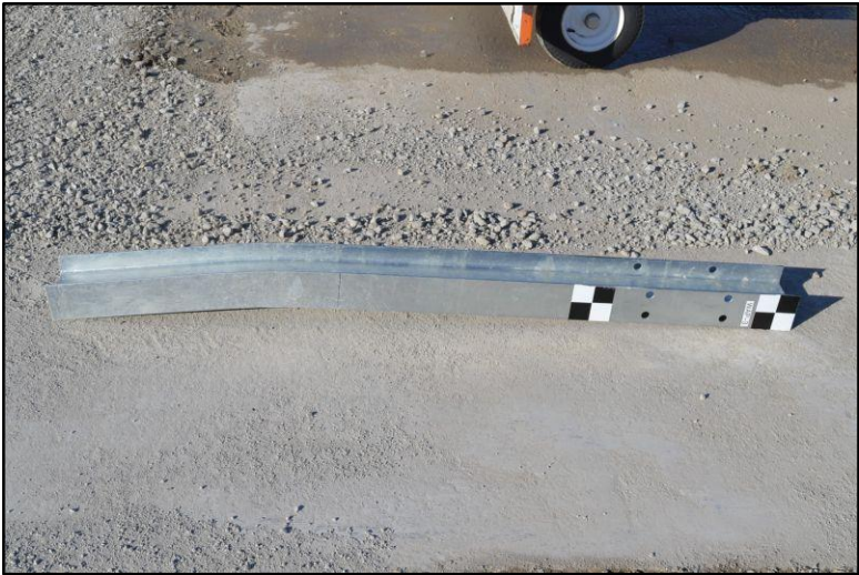
Figure 11. Time-Sequential and Post-Impact Photographs, Test No. WAP-3
