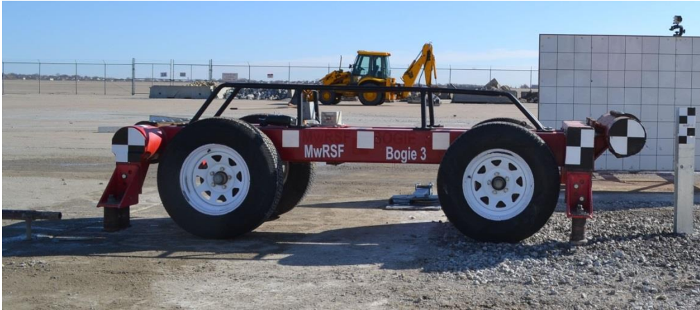
Figure 1. Rigid-Frame Bogie on Guidance Track
