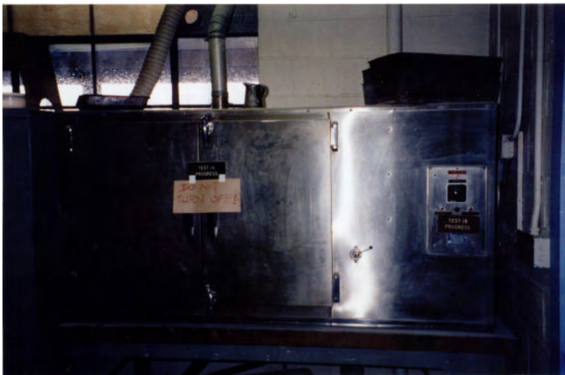
Photo 14. Modern Lab Equipment oven, model 657-SS, used to dry sample bags after test.
