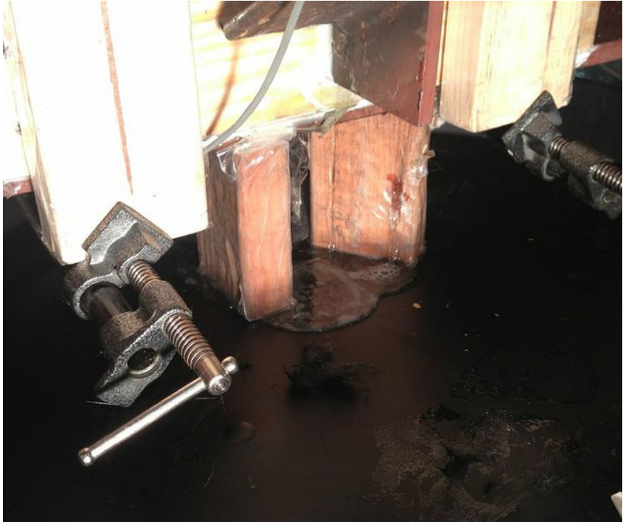
Figure B.6: Epoxy Leaking Out of Mold Insuring Air Pockets Would Not Be Present in the Block
