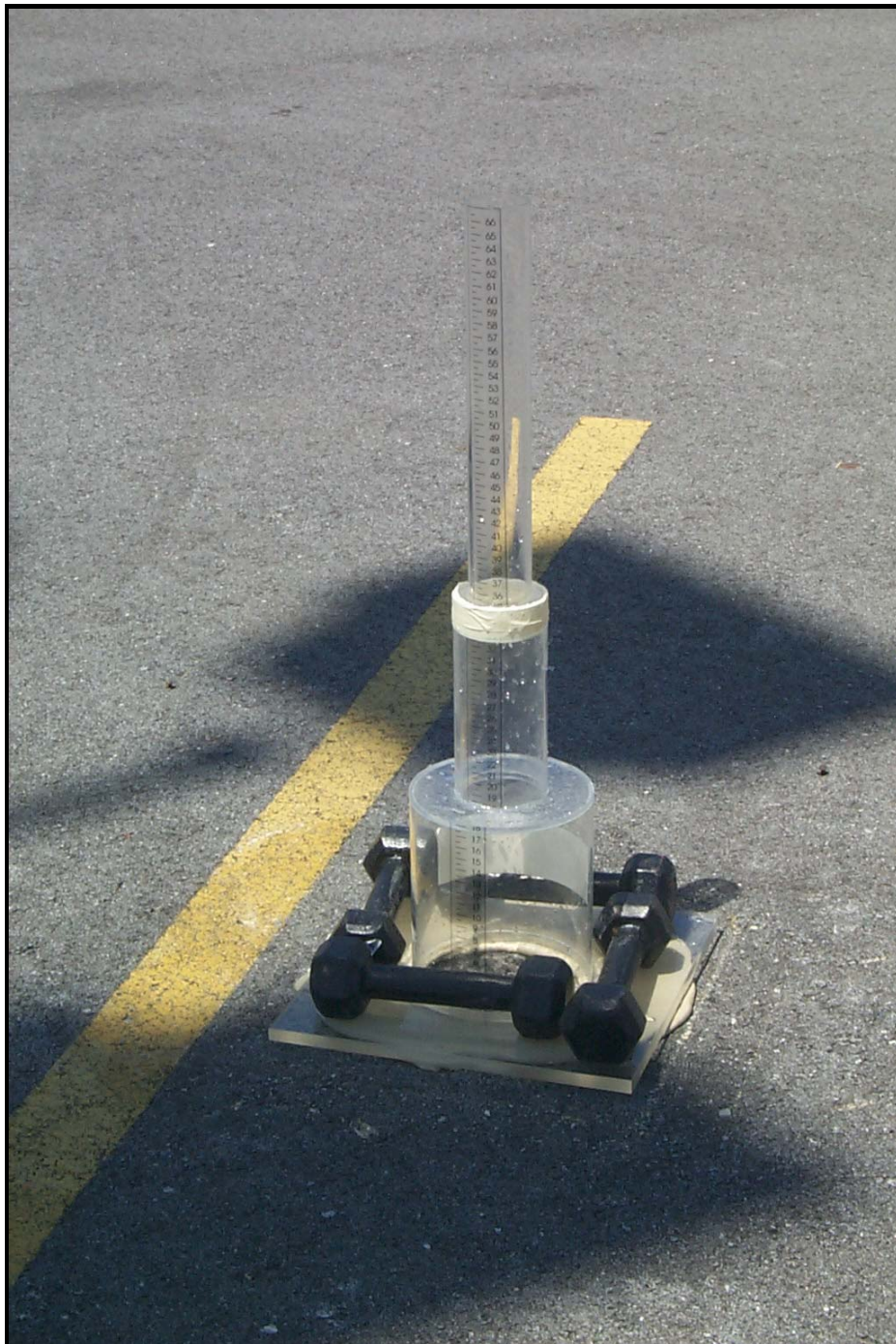
Figure 3. NCAT Field Permeameter
