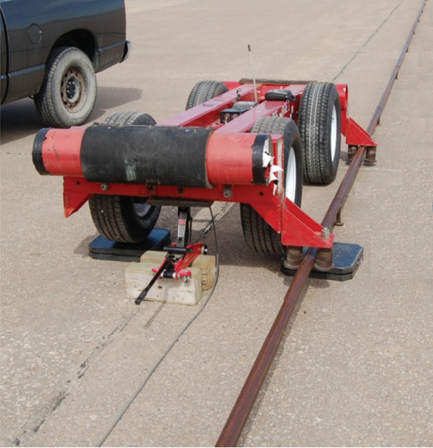
Figure 2. Rigid Frame Bogie on Guidance Track
