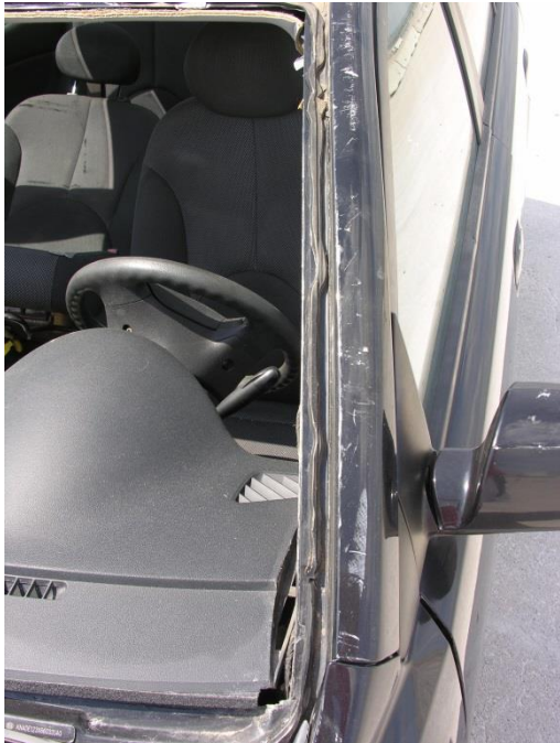
Figure 160. Vehicle Damage - Windshield, Test No. WIDA-2
