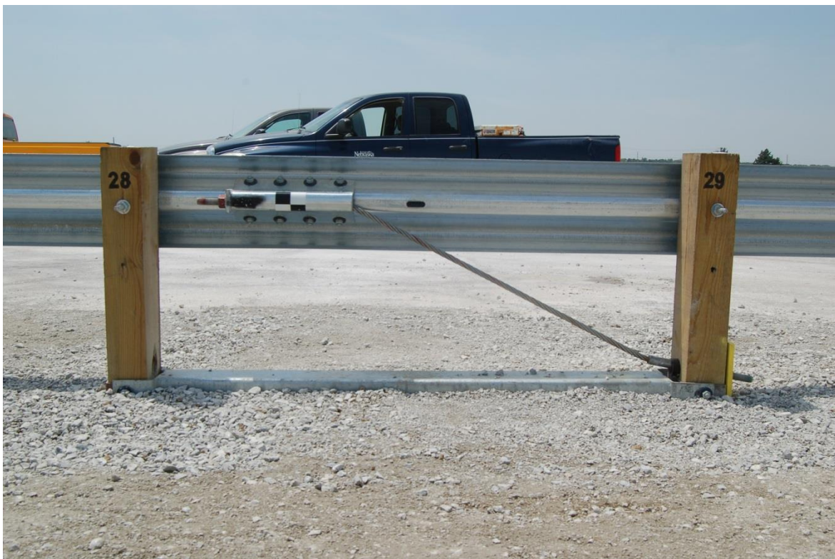
Figure 122. Test Installation Photographs, Test No. WIDA-1
