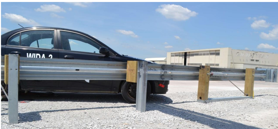
Figure 150. Impact Location, Test No. WIDA-2
