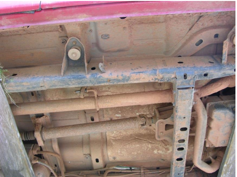
Figure 144. Undercarriage and Suspension Damage, Test No. WIDA-1
