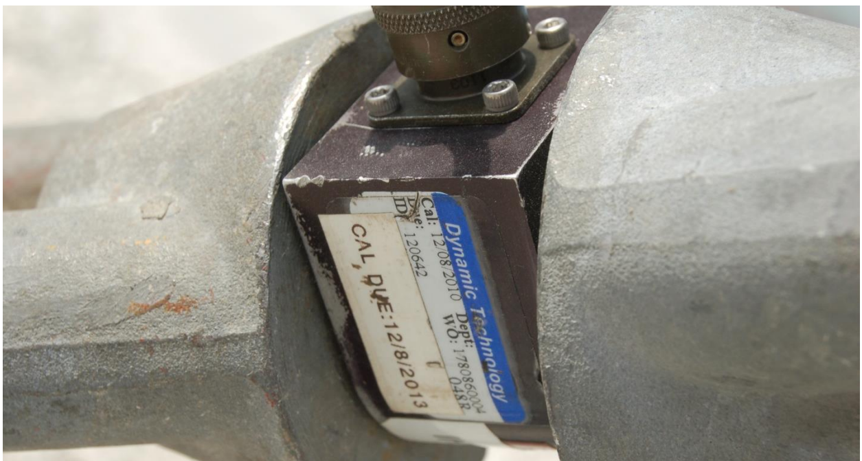
Figure 101. Load Cell Setup, Test No. WIDA-1
