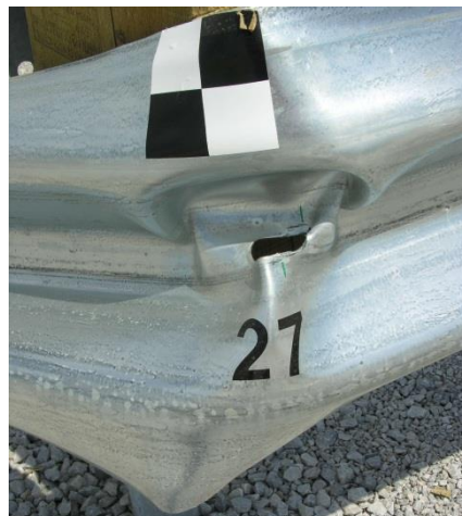
Figure 154. Rail Damage, Test No. WIDA-2
