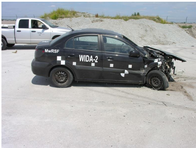
Figure 157. Vehicle Damage, Test No. WIDA-2
