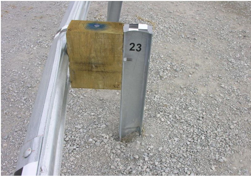
Figure 139. System Damage at Post Nos. 21 through 24, Test No. WIDA-1
