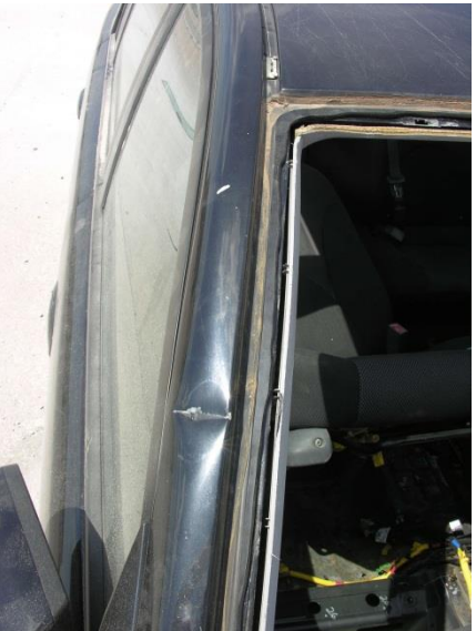
Figure 159. Vehicle Damage - Windshield Glue Strip, Test No. WIDA-2
