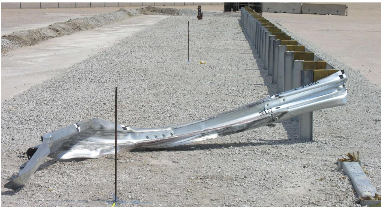
Figure 152. System Damage, Test No. WIDA-2
