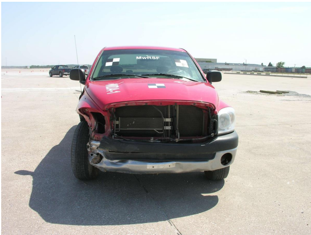
Figure 142. Vehicle Damage, Test No. WIDA-1
