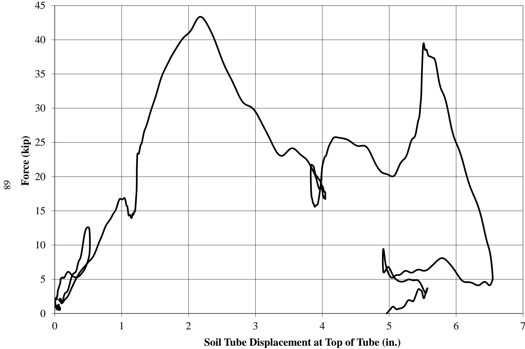
Figure 39. Bogie Force vs. Soil Tube Displacement Measured by String Pot, Test No. MGSEA-1
