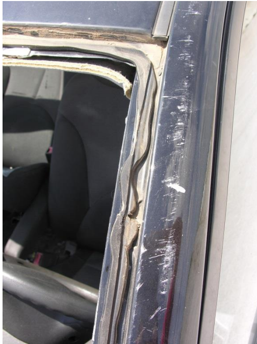
Figure 160. Vehicle Damage - Windshield, Test No. WIDA-2
