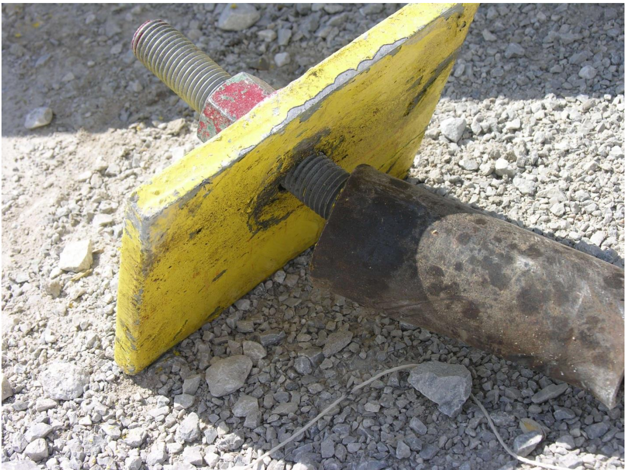
Figure 156. Anchor Cable Damage, Test No. WIDA-2
