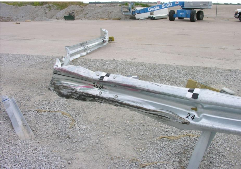
Figure 138. Details of Rail Damage, Test No. WIDA-1
