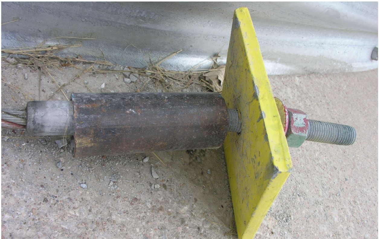
Figure 141. Anchor Cable Damage, Test No. WIDA-1
