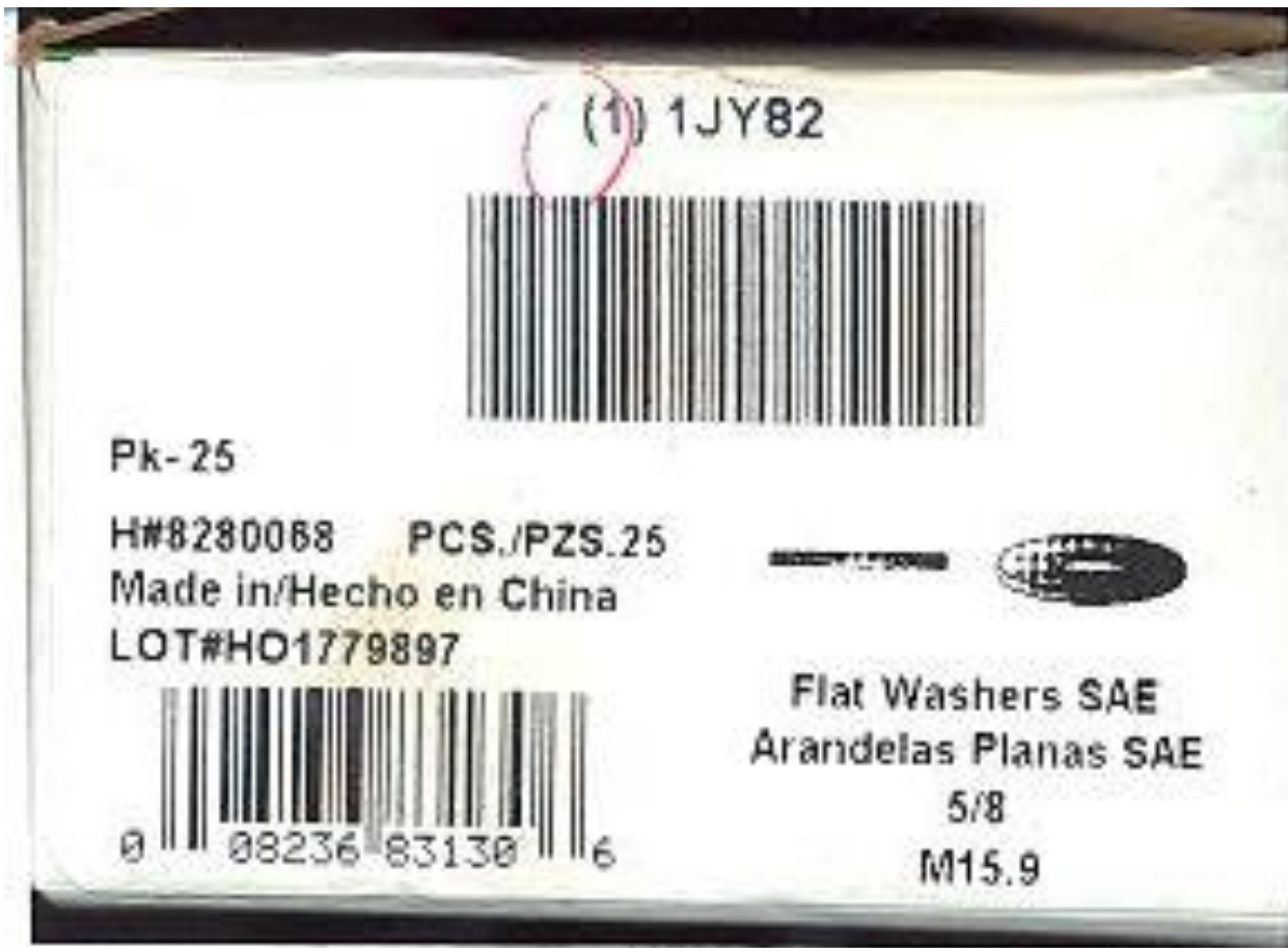
Figure B-47. 5/8 in. (16 mm) Diameter Flat Washer, Part b5, Test Nos. WIDA-1 and WIDA-2
