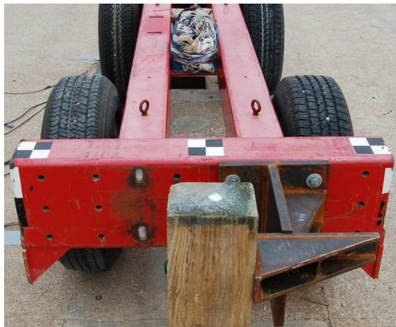
Figure 4. Rigid-Frame Bogie used for Test Nos. BCTRS-1 and BCTRS-2
