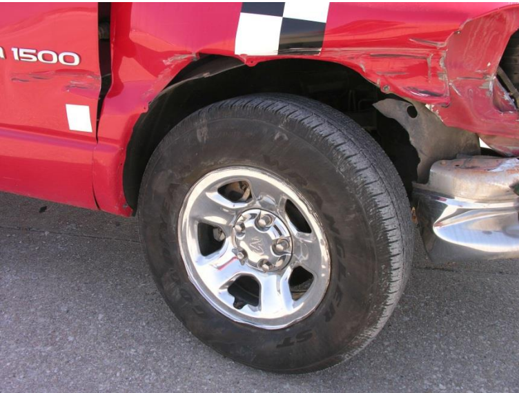
Figure 143. Vehicle Damage, Test No. WIDA-1
