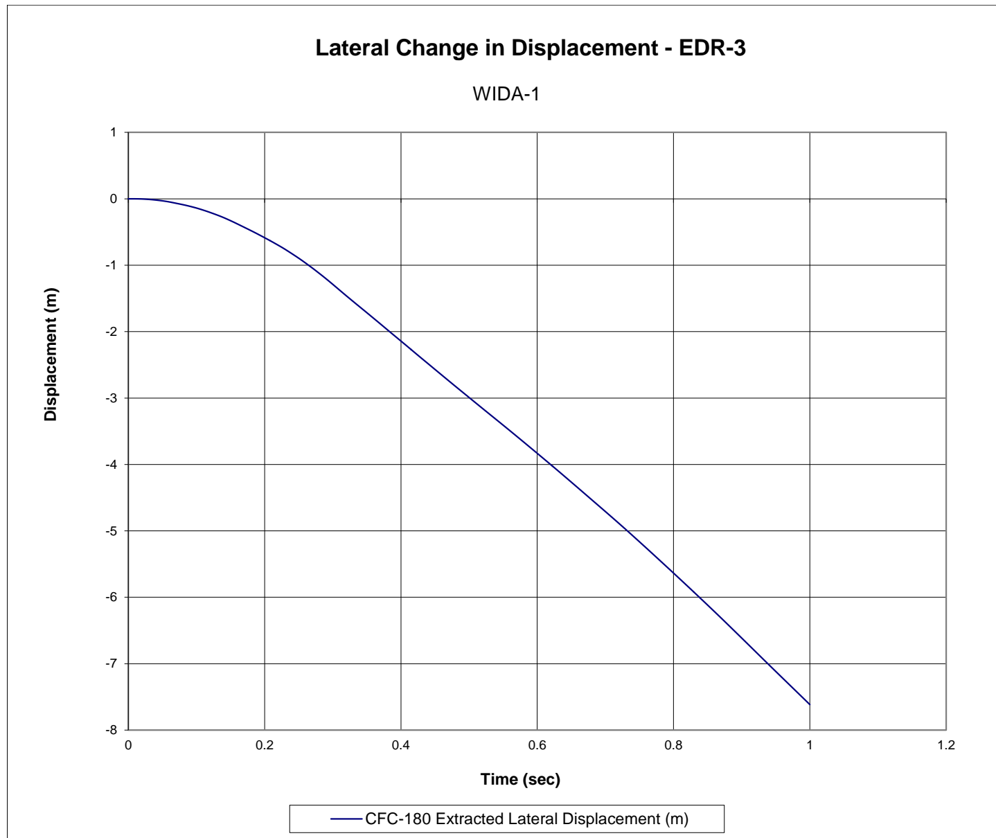
Figure I-22. Lateral Occupant Displacement (EDR-3), Test No. WIDA-1
