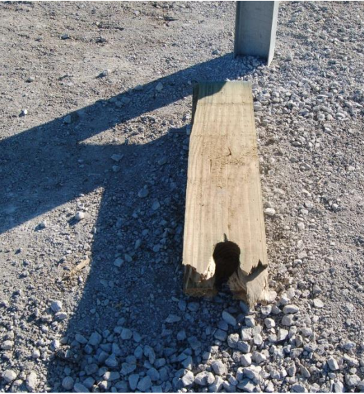
Figure 59. Post-Impact Photographs, Test No. DSAP-2
