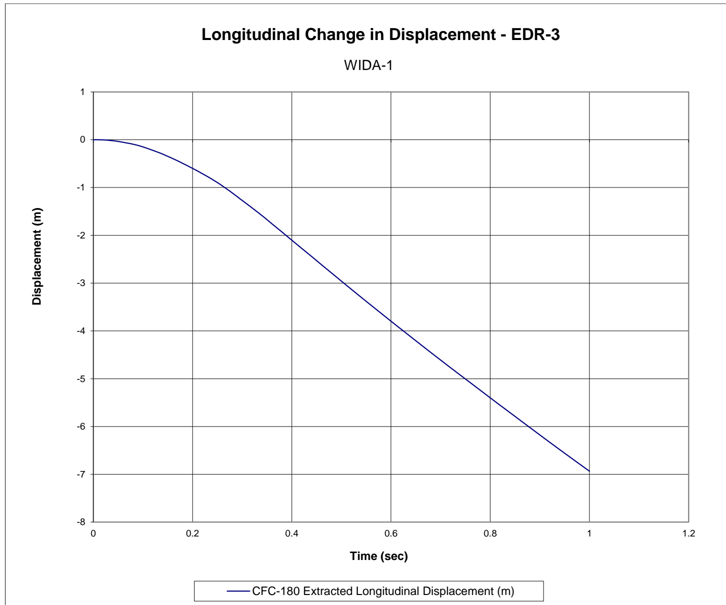
Figure I-19. Longitudinal Occupant Displacement (EDR-3), Test No. WIDA-1
