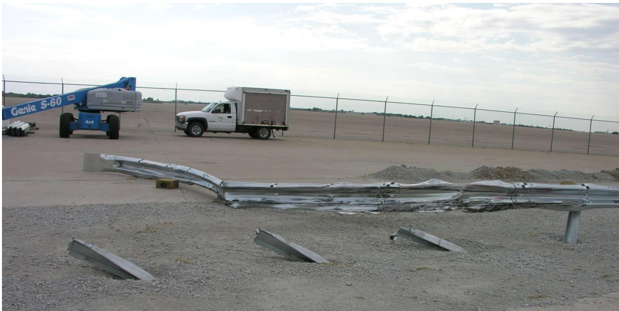
Figure 136. System Damage, Test No. WIDA-1
