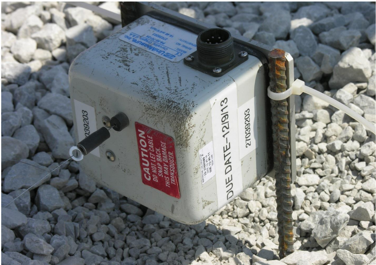
Figure 102. String Pot Setup, Test No. WIDA-1
