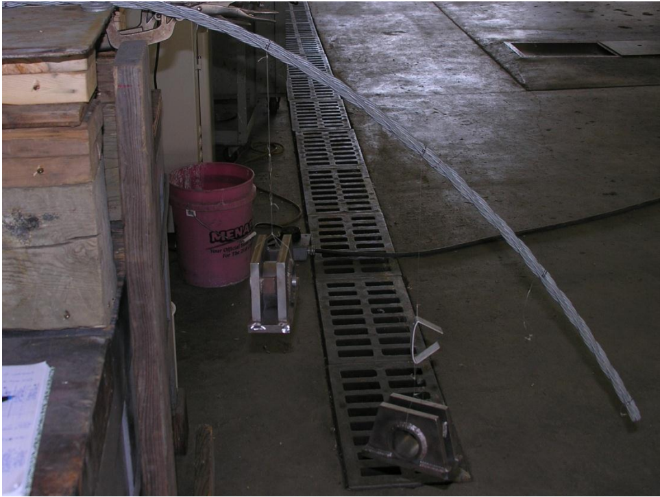
Figure 87. Loading Configuration and Method of Applying Discrete Weights
