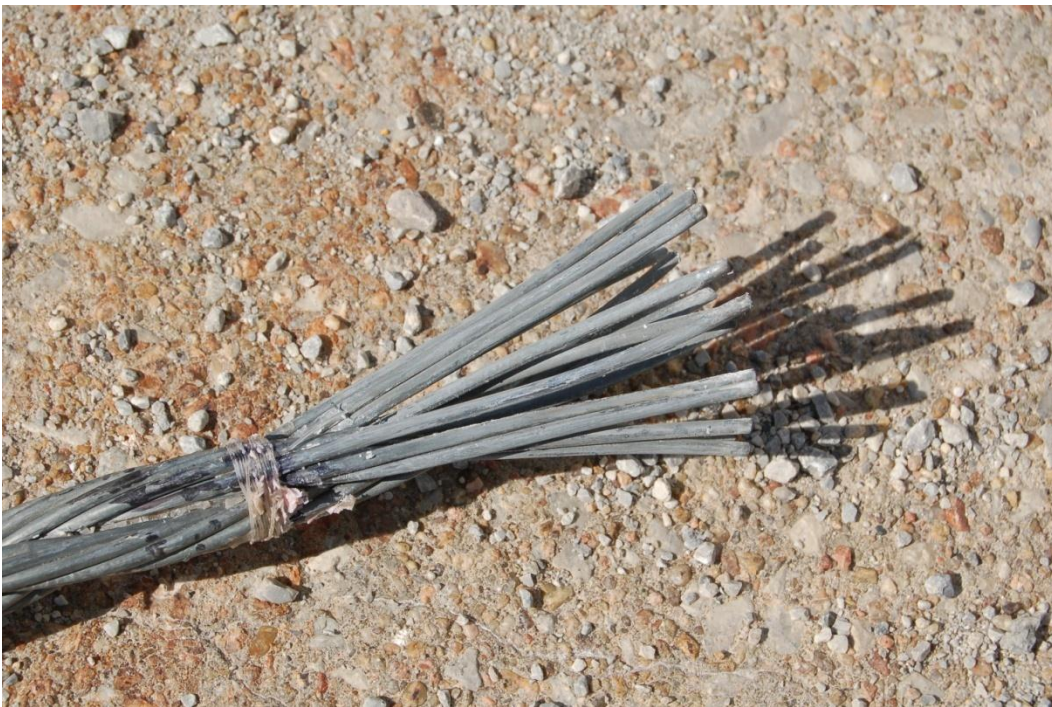
Figure 128. Wire Rope Pullout, Test No. DBC-3
