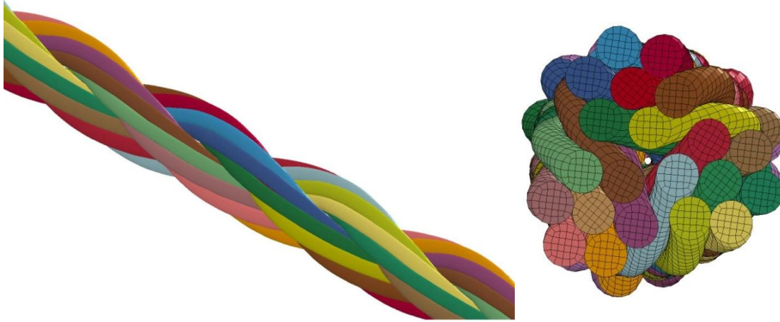
Figure 2. Solid Element Model of \frac{3}{4} -in. (19-mm) Wire Rope
