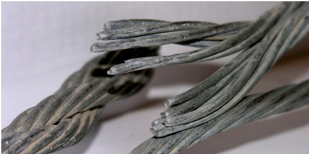
Figure 15. Fracture Location at String Pot U-bolt, Non-Prestretched Wire Rope Test
