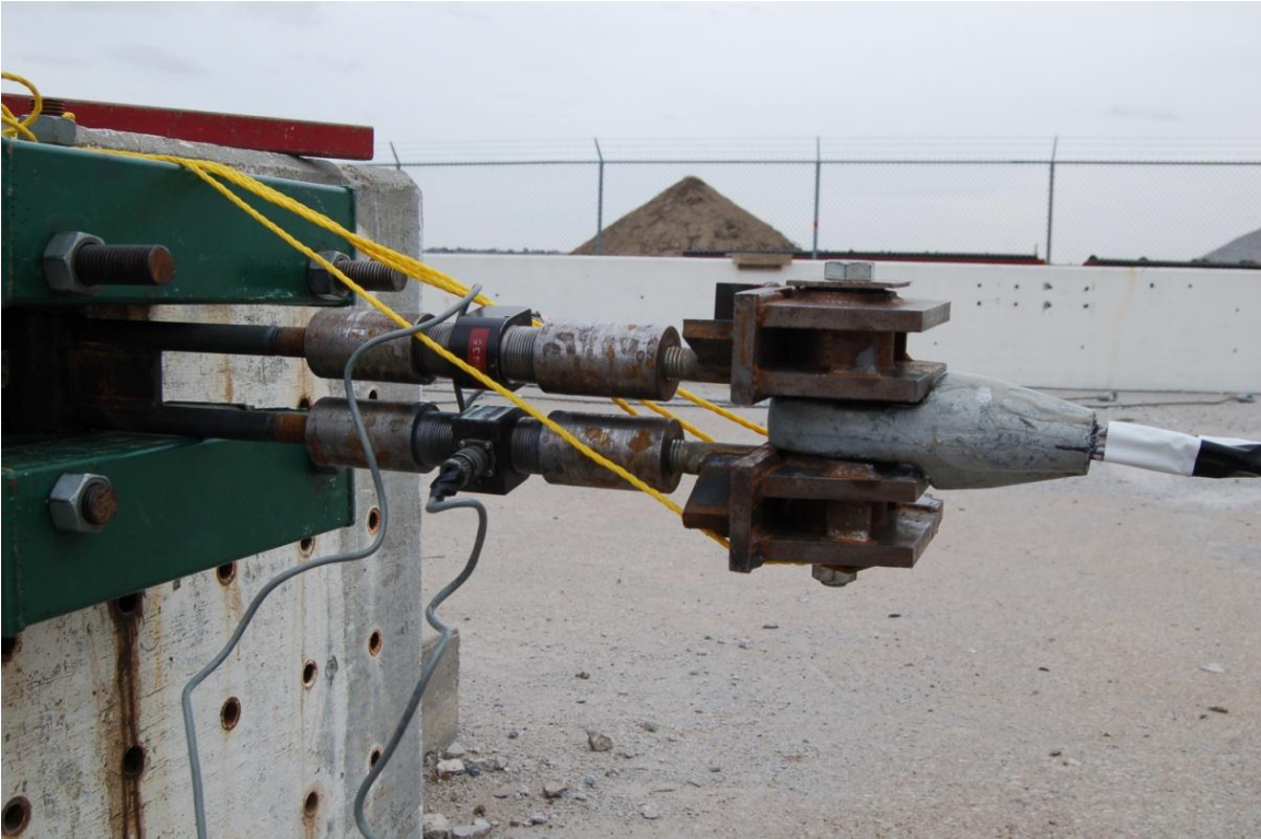
Figure 52. Load Frame, Test Nos. DTC 1-3
