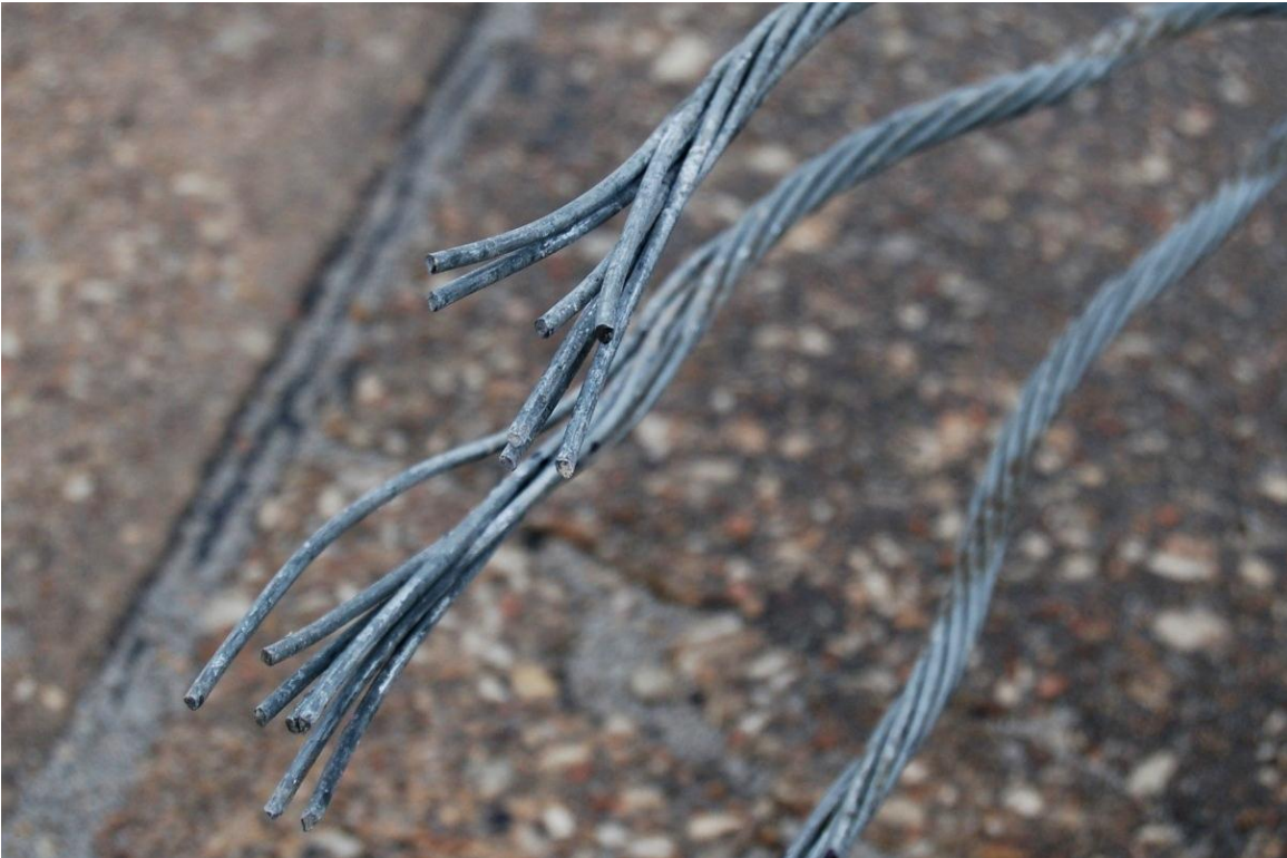
Figure 147. Wire Rope Damage, Test No. DBC-6
