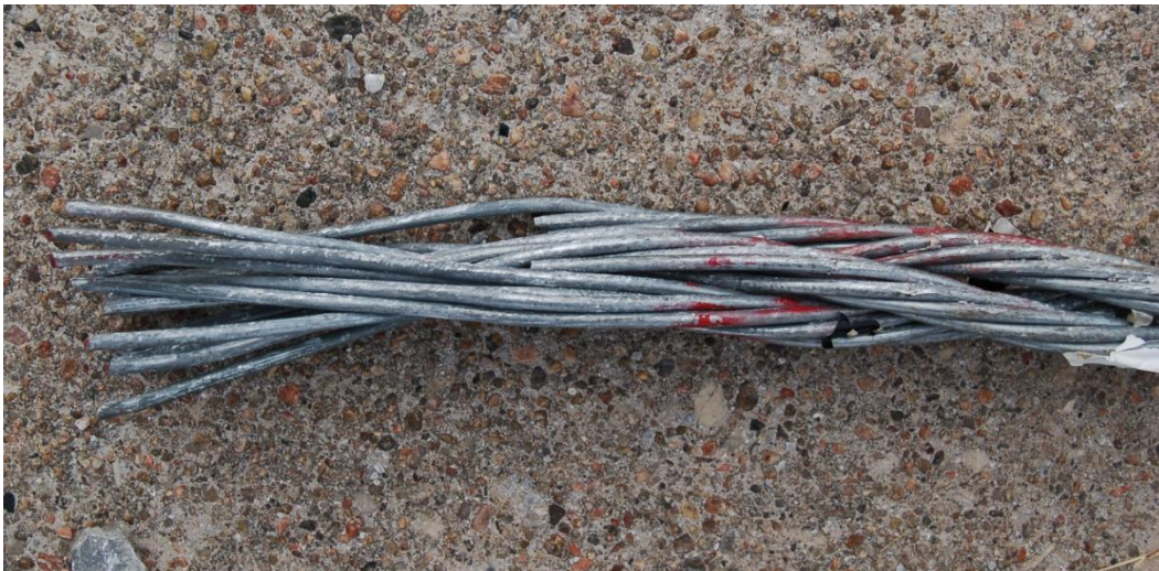
Figure 72. Wire Rope Pullout of Downstream Socket, Test No. DTC-3
