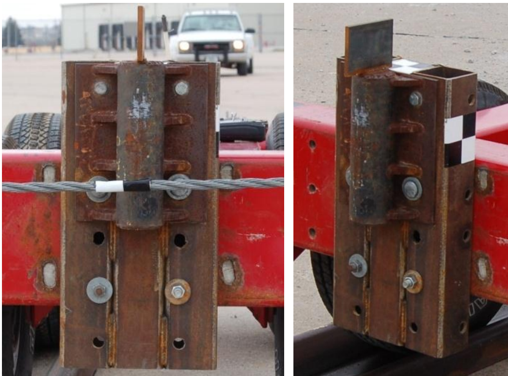
Figure 112. Impact Head and Mounting Post, Component Test Nos. DBC 1-6
