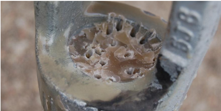
Figure 69. Pullout of Downstream Wire Rope Socket, Test No. DTC-2
