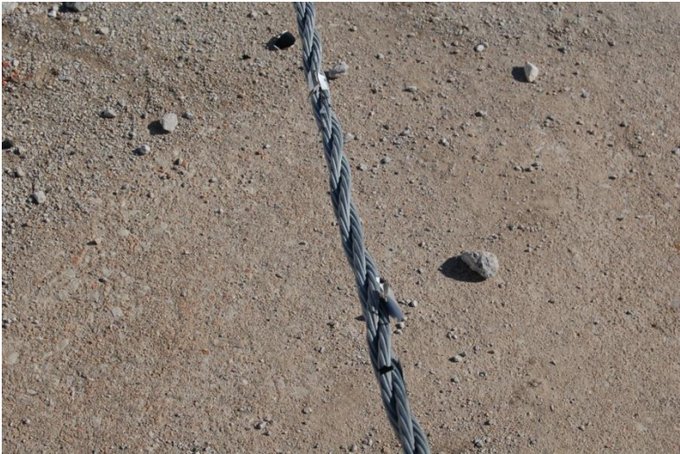
Figure 133. Wire Rope Damage, Test No. DBC-4
