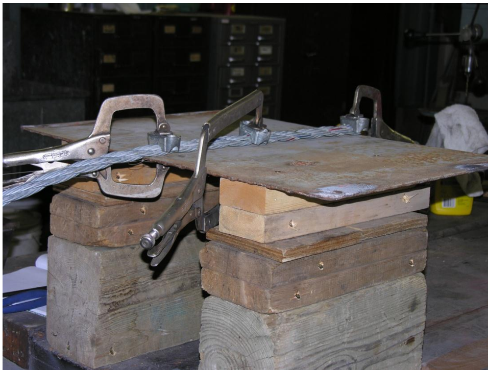
Figure 85. Clamped Configuration of Long Wire Rope Quasi-Static Bending Test
