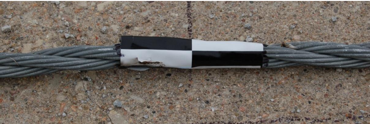
Figure 143. Wire Rope Damage, Test No. DBC-5
