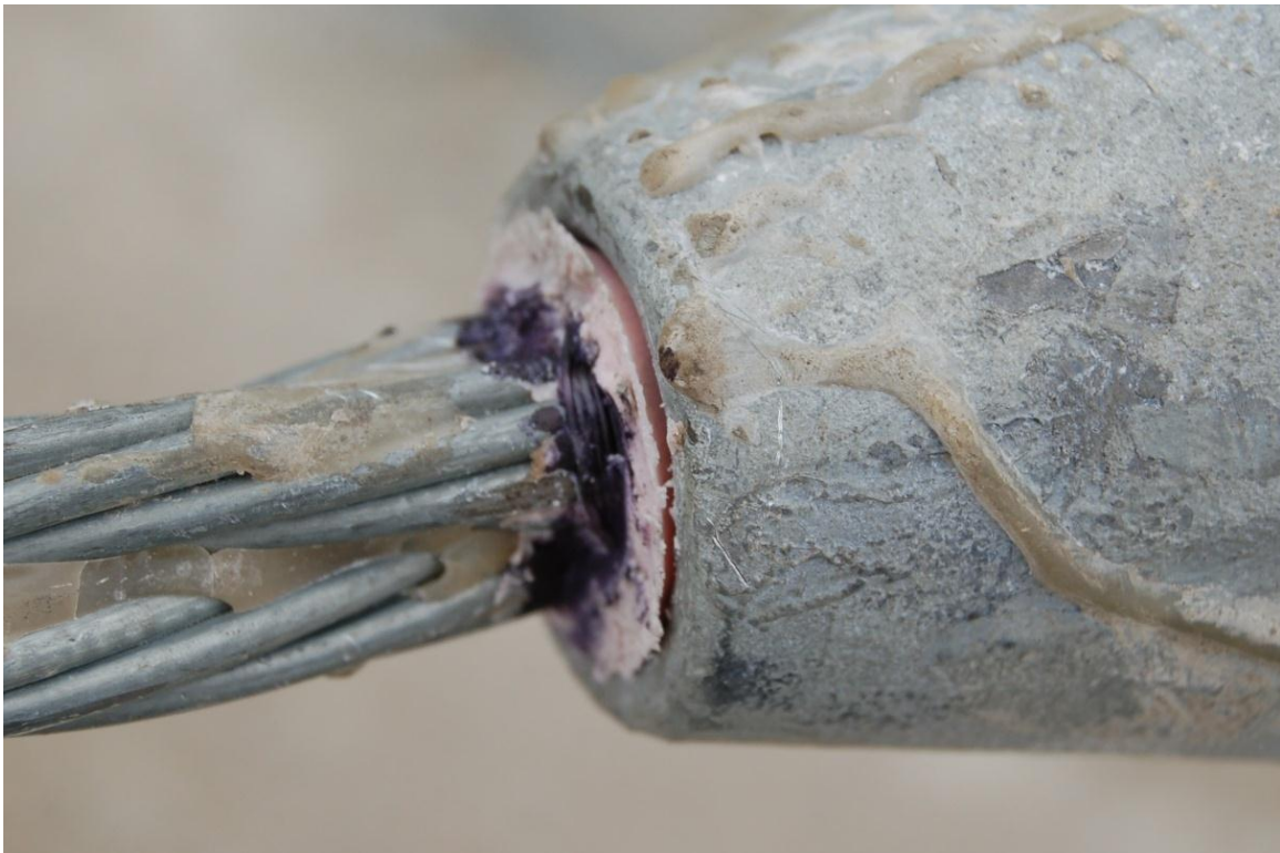
Figure 144. Wire Rope End Fitter Damage, Test No. DBC-5
