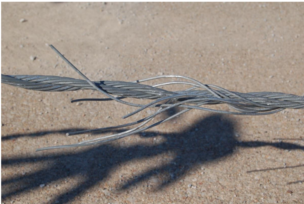
Figure 134. Wire Rope Damage, Test No. DBC-4
