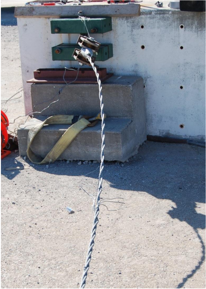
Figure 132. Wire Rope Damage, Test No. DBC-4
