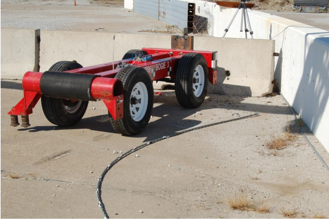
Figure 127. Final Position of Bogie Vehicle and Wire Rope, Test No. DBC-3
