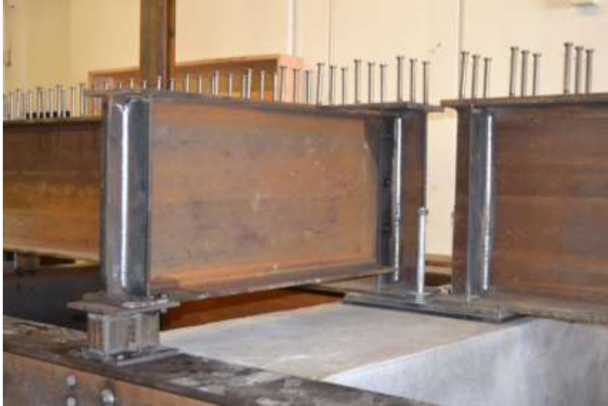
Figure 5.5 Steel Diaphragm Beam
