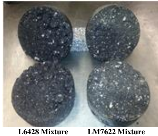
Figure 31. Picture of no tack coat specimens after testing in the LISST jig.
