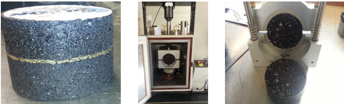
Figure 12. LISST test setup with a Specimen before and after Testing.
