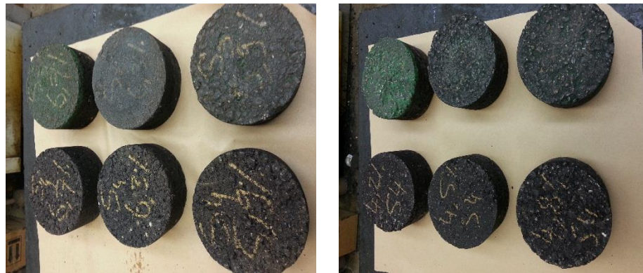
Figure 16. Pictures of moisture-conditioned samples before and after the raveling testing.
