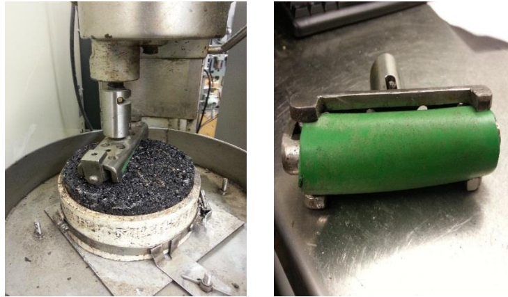
Figure 8. Installed raveling test adapter with a specimen ready for testing.
