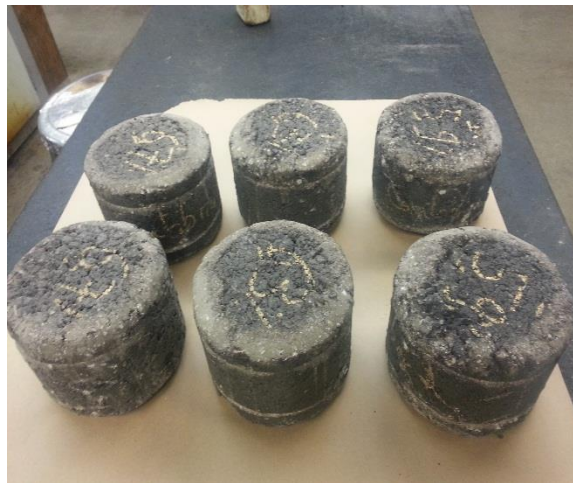
Figure 18. Picture of L6428 samples after testing for surface abrasion.
