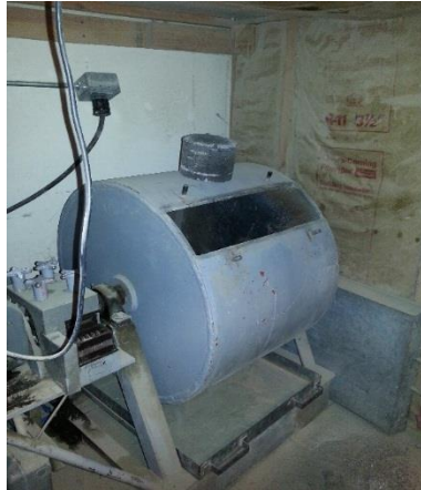
Figure 9. Los Angeles abrasion machine with a thin AC overlay specimen after testing.
