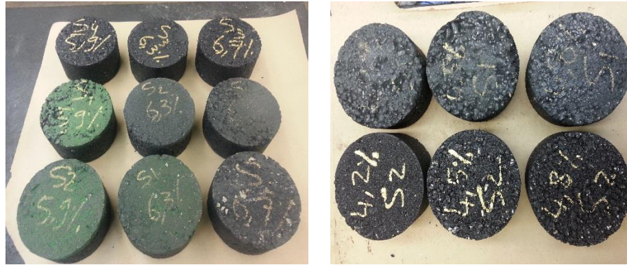
Figure 15. Pictures of unconditioned samples before and after the raveling testing.
