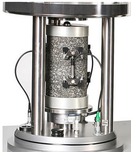
Figure 10. Dynamic modulus testing setup.
