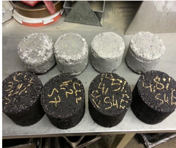
Figure 19. Picture of LM7622 samples before and after testing for surface abrasion.
