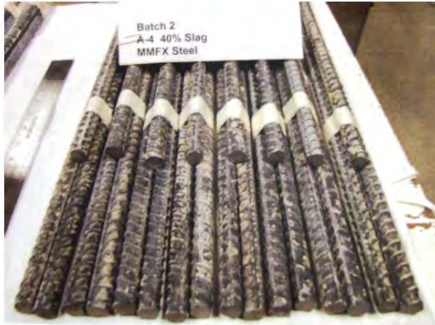
Figure 6. 60% PC + 40% Slag Ready-Mixed Batch
