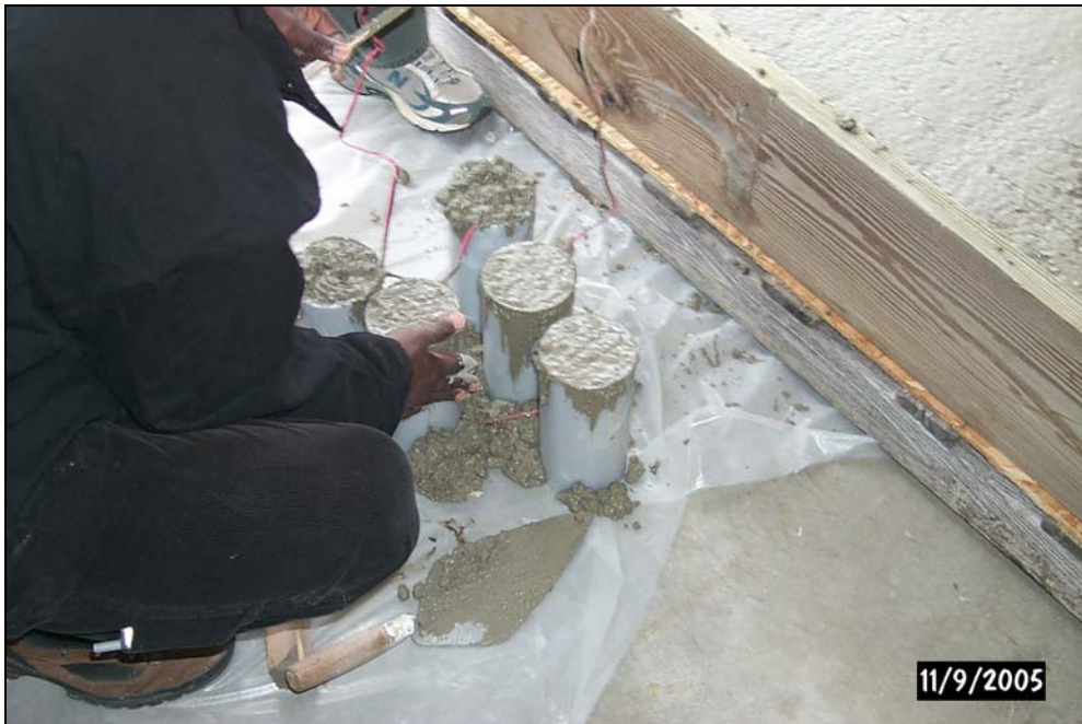
FIGURE B10 Placement of maturity meter in cylinders.
