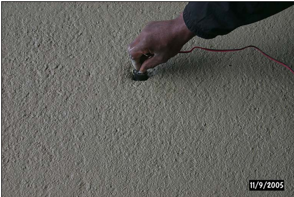
FIGURE B12 Placement of maturity meter in center of test slab.
