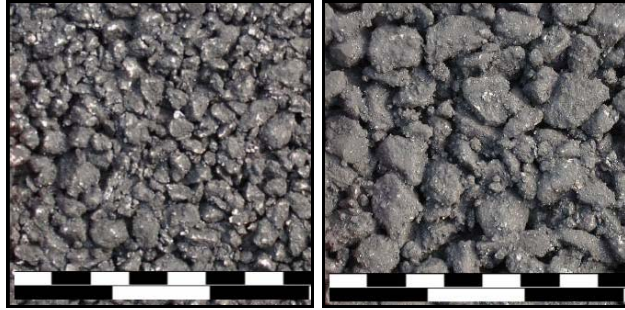
Figure 7. Surface Texture of PFC/OGFCs (left) and PA-coarse (right) Mixtures (17).
