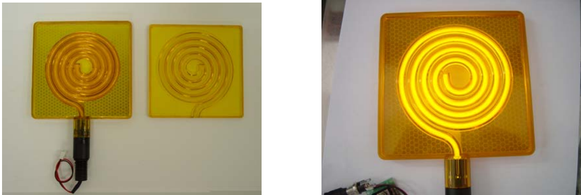
Fig. 5 EL Fiber Housing with Passive Reflector around Spiral Lamp
