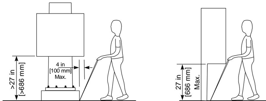
When an obstruction of a height greater than 27 in [686 mm] from the surface would create a protrusion of more than 4 in [100 mm] into the pedestrian circulation area, construct additional curb or foundation at the bottom to provide a maximum 4 in [100 mm] overhang.
