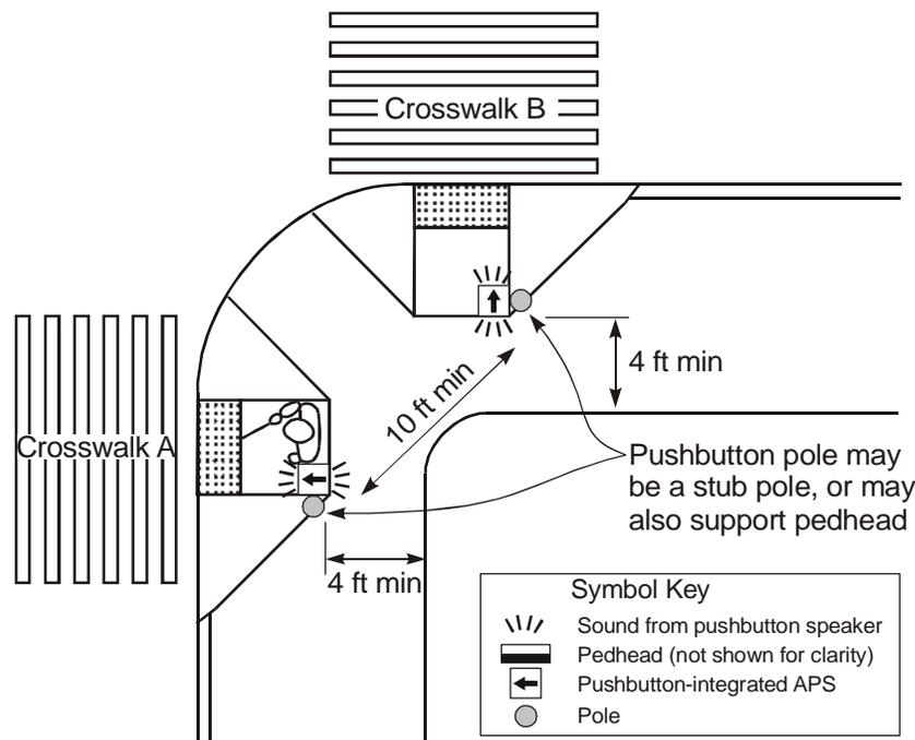
Figure 8-13. Recommended Placement for Pedestrian Push Buttons — Integrated APS in New Construction.<sup>14</sup>
