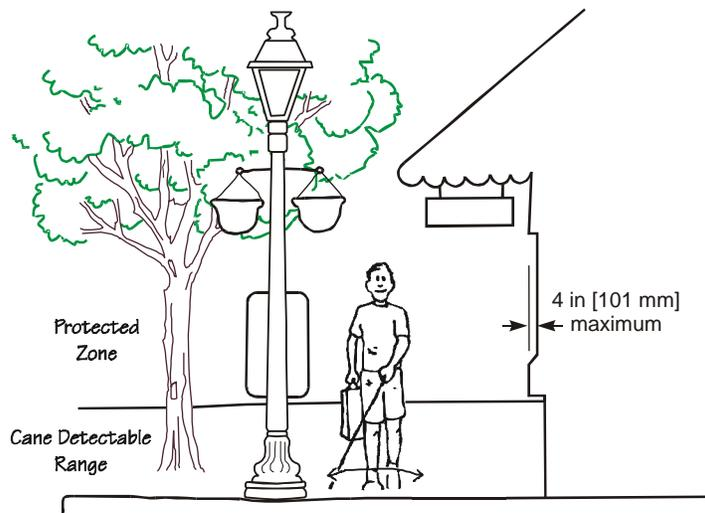
Figure 5-6. Post-Mounted Objects (Post-Mounted Objects Seen in Elevation, Dimensioned to Indicate 4 inch [101 mm] Maximum Protrusion).<sup>10</sup>
