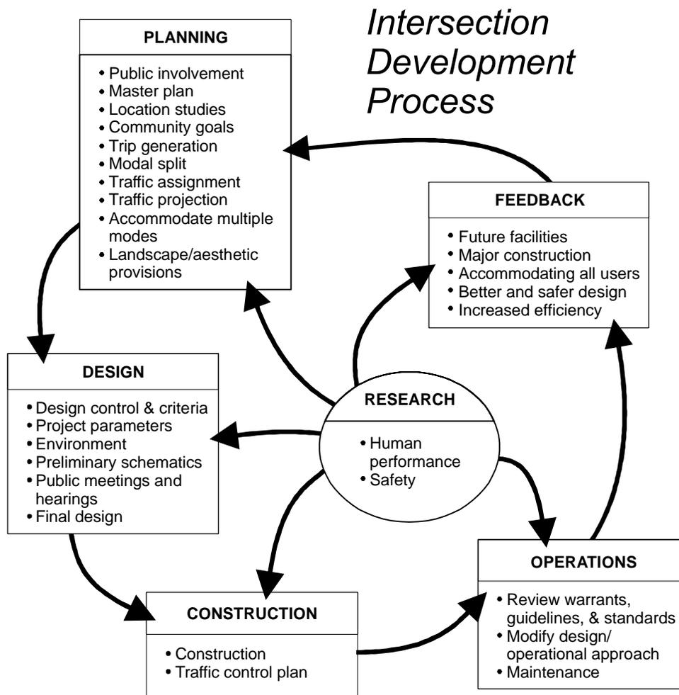
Figure 1-1. The Intersection Development Process.
