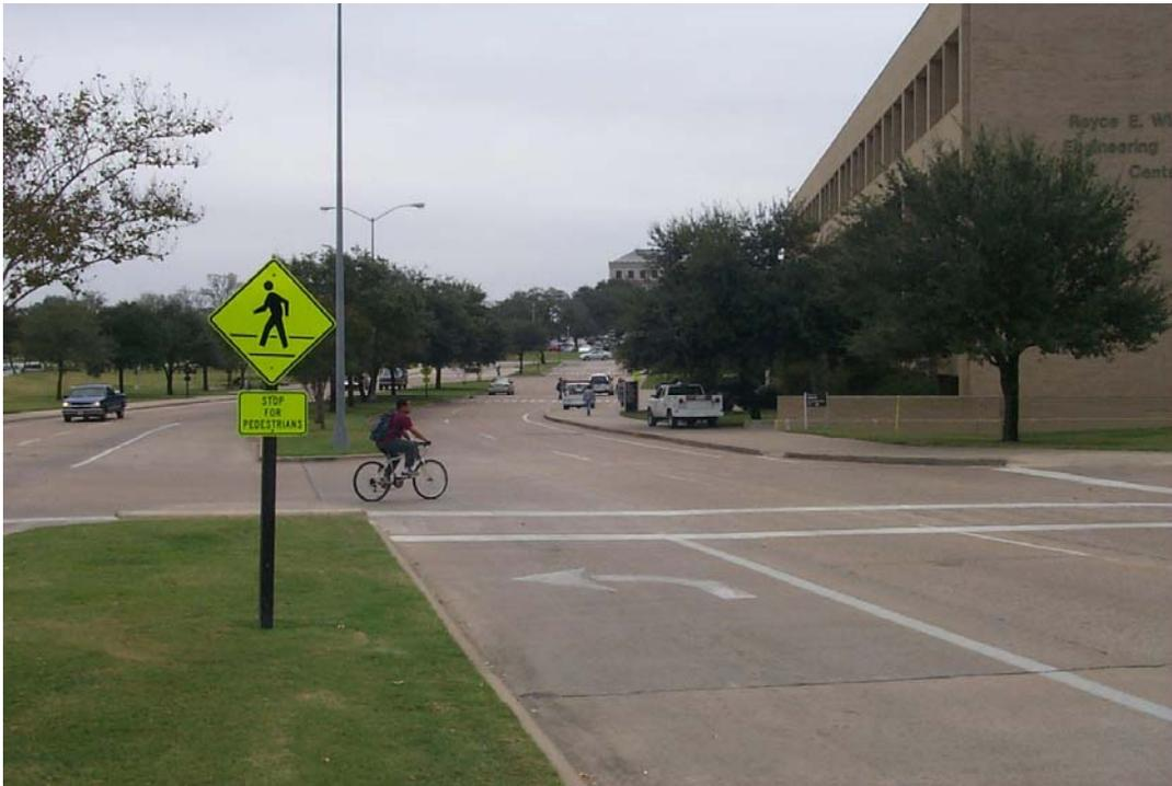
Figure 9-2. Example of Transverse Pavement Markings (Arrow and Crosswalk).
