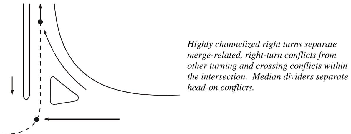
Figure 4-11. Channelized Right Turns.<sup>8</sup>
