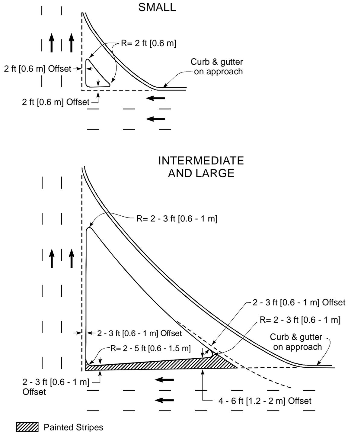
Figure 4-17. Details of Corner Island Designs for Turning Roadways (Urban Locations).
