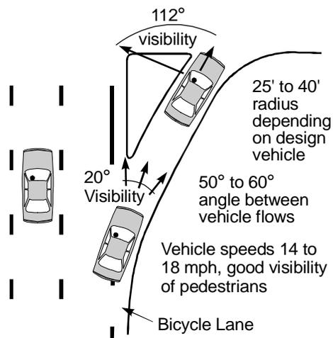
Figure 4-18. Suggested Design for Right-Turn Lane with Island.<sup>11</sup>
