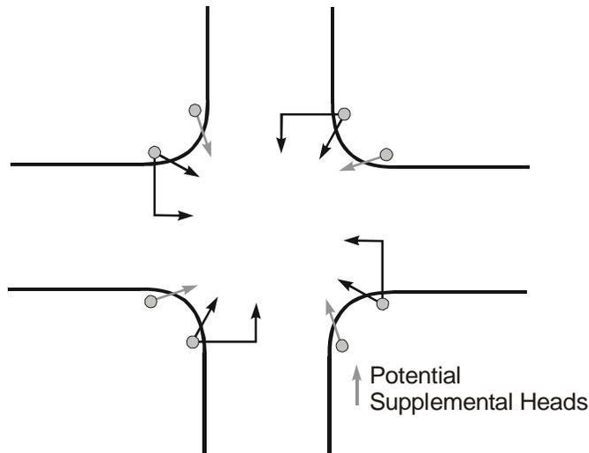
Figure 8-10. Mast Arm Mounting with Post-Mounted Signals.<sup>7</sup>
