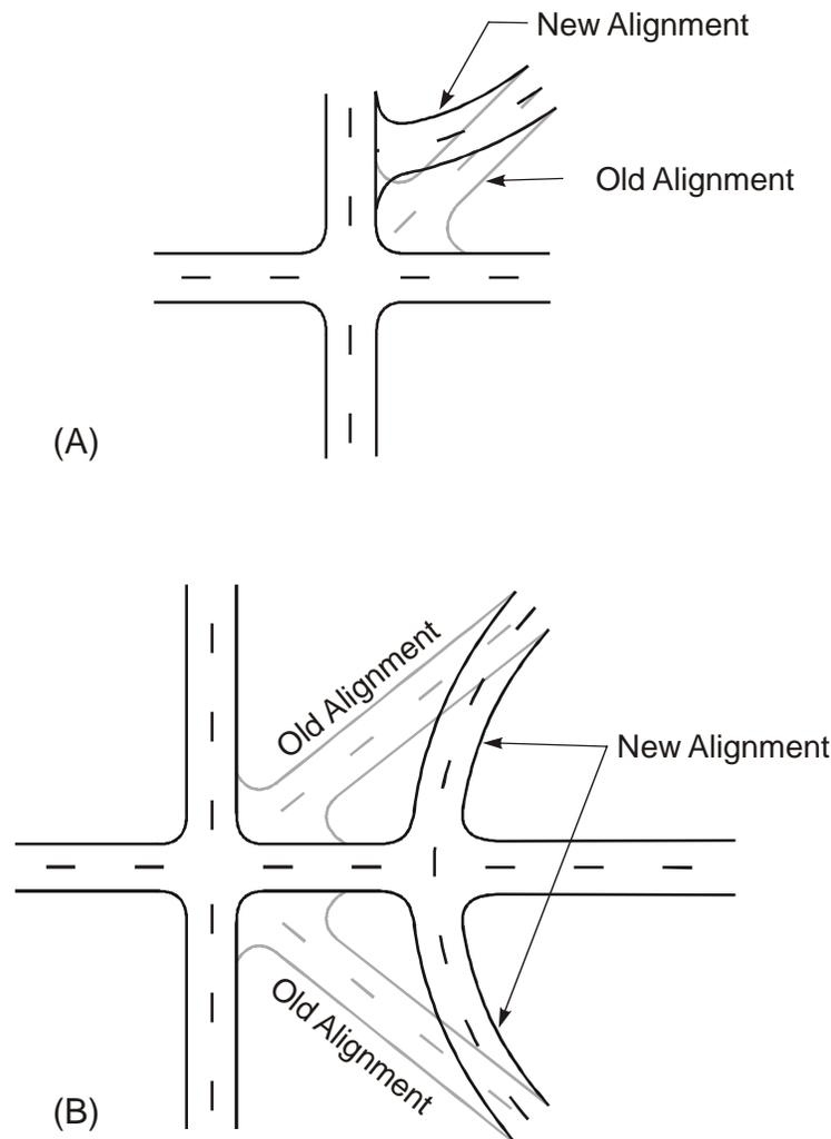
Figure 3-5. Realigning Multileg Intersections.<sup>3</sup>
