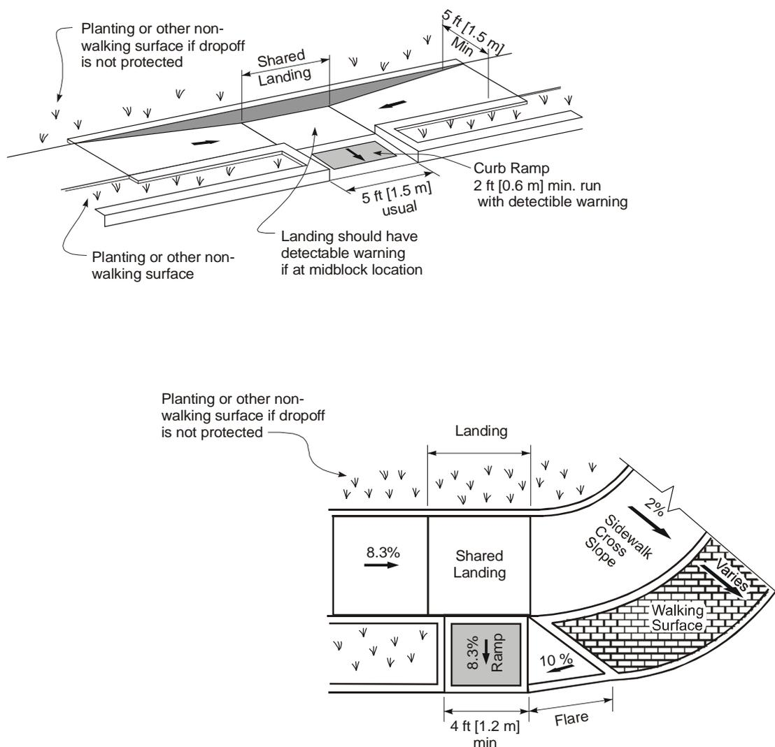
Figure 7-6. Examples of Combination Curb Ramps.
