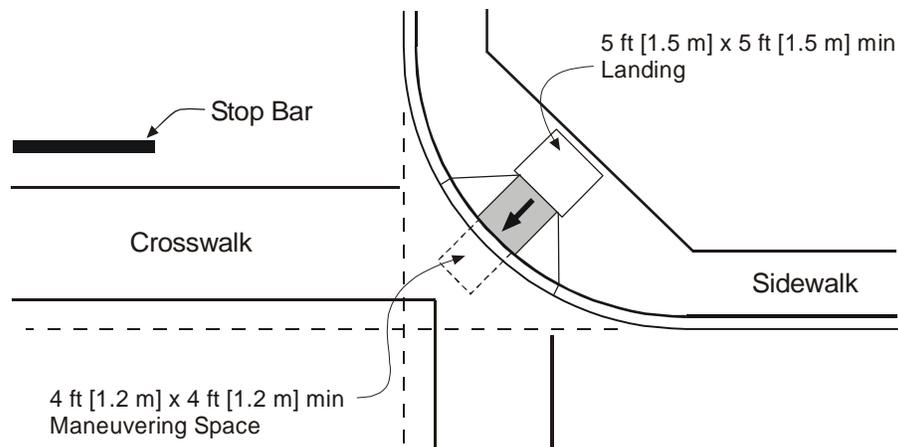
Figure 7-7. Diagonal Curb Ramp.
