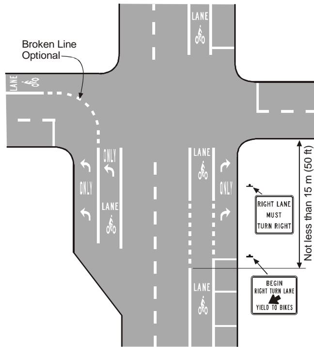
*Figure 9-13. Typical Intersection Pavement Markings with Designated Bicycle Lane with Left-Turn Area, Heavy Turn Volumes, Parking, One-Way Traffic, or Divided Highway.<sup>1</sup>*
