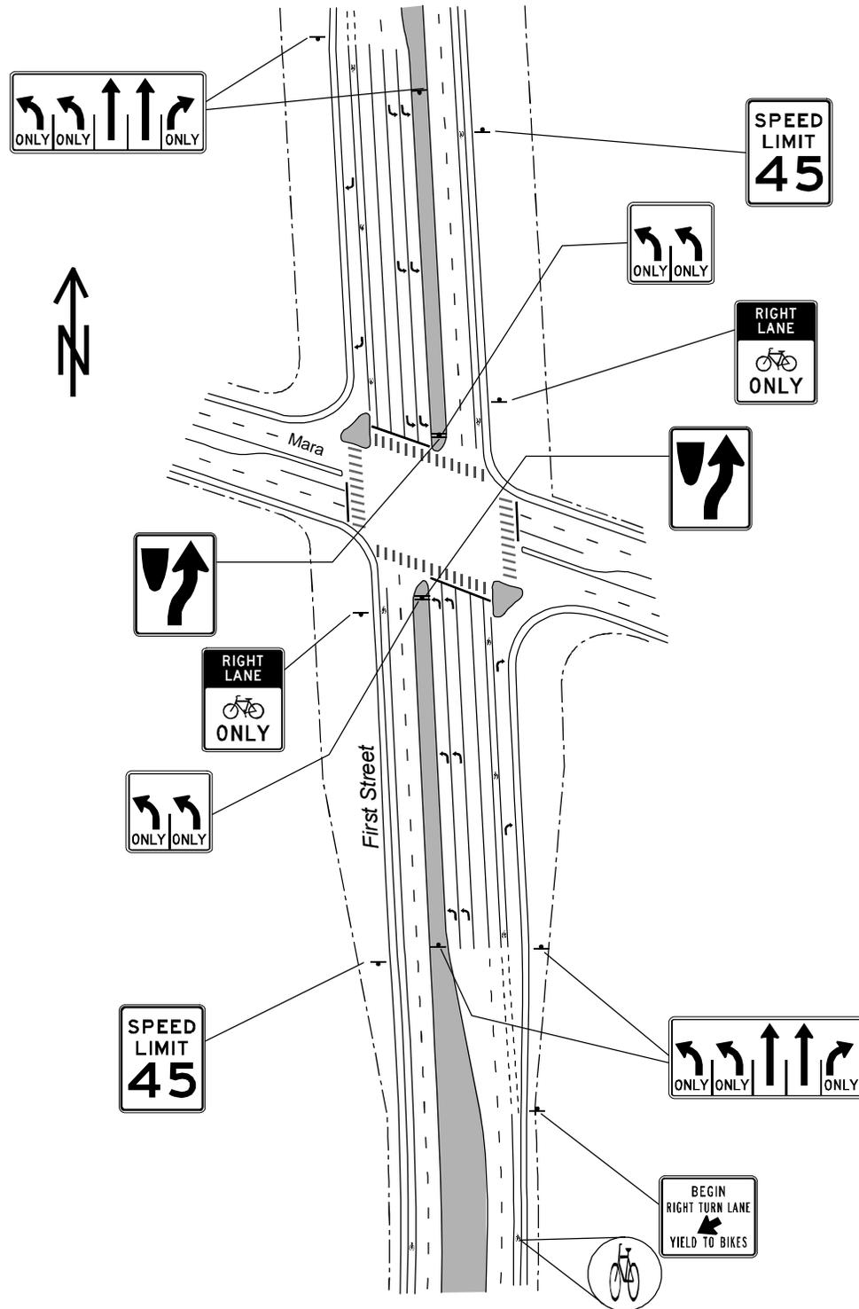
Figure 9-1. Sketch of Intersection with Bicycle Lane Carried through Right-Turn Lane
