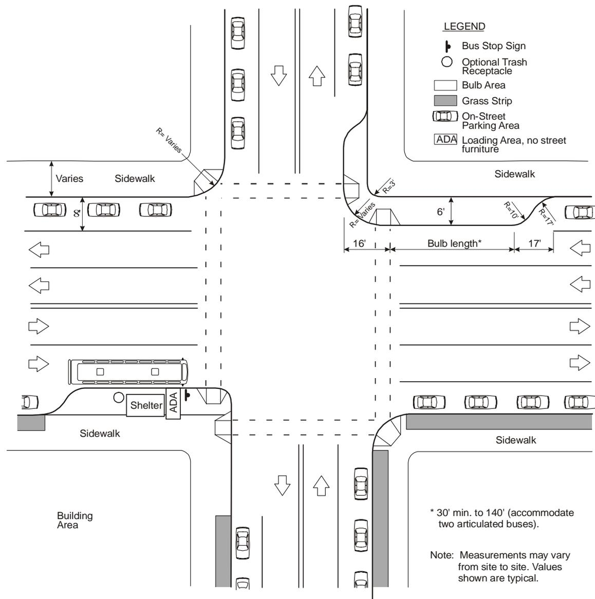
Figure 5-24. Typical Bus Bulb Dimensions.<sup>15</sup>
