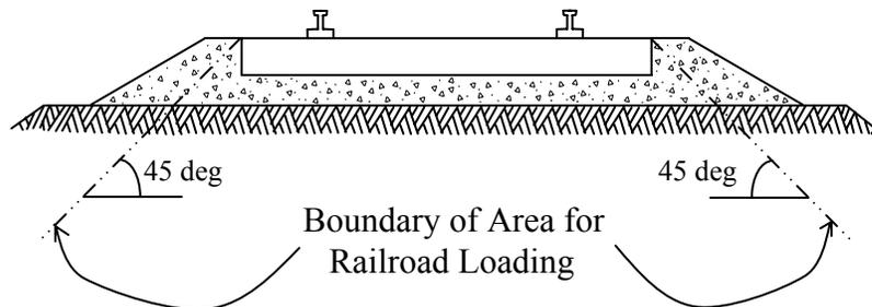
Figure 6-15. Diagram Showing Area Requiring Consideration for Railroad Loading.
