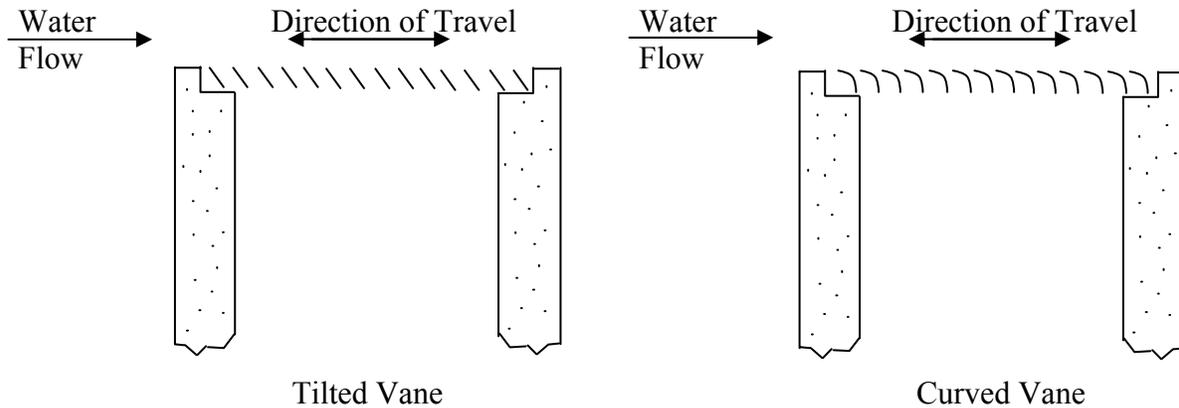
Figure 6-12. Tilted Vane (or “Bar”) and Curved Vane Grate Inlets.
