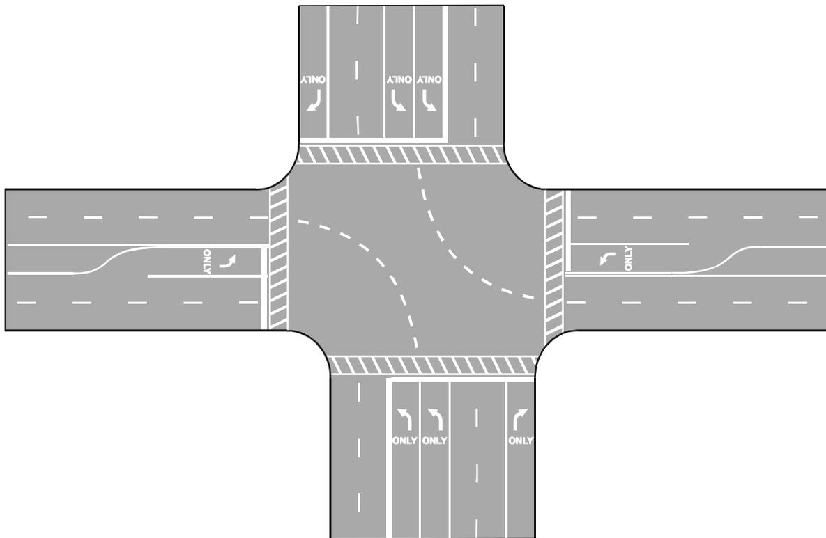
Figure 9-5. Typical Dotted Line Markings to Extend Longitudinal Lane Line Markings.
