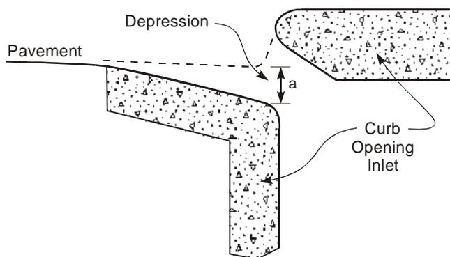
Figure 6-9. Depression at Curb Opening Inlet.
