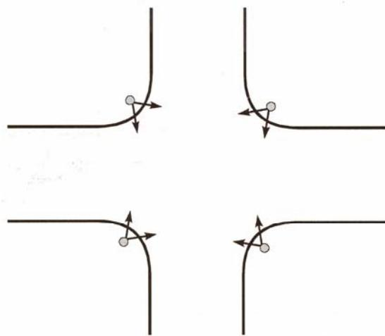
Figure 8-4. Post-Mounted Signals.<sup>7</sup>
