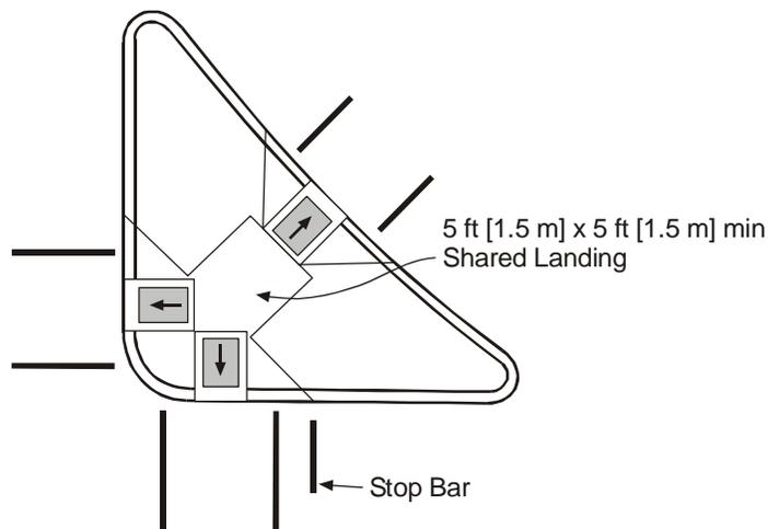
Figure 4-24. Typical Layout of Curb Ramps at a Channelizing Island.<sup>15</sup>
