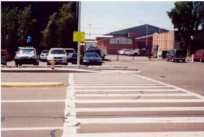
*Figure 7-21. Example of High-Visibility Markings.*
