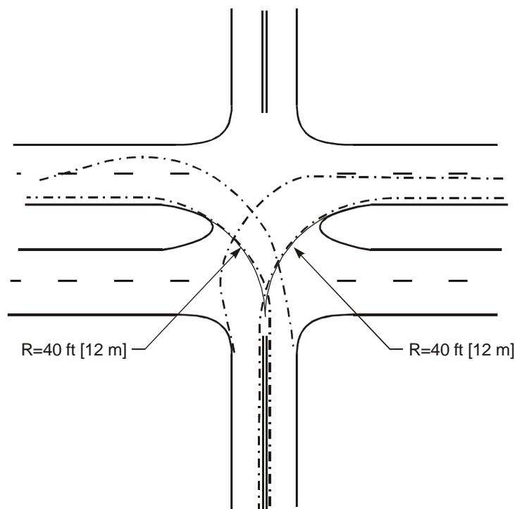
Figure 4-23. Minimum Design of Median Openings (WB-50 [WB-15], Control Radius of 40 ft [12 m]).<sup>2</sup>
