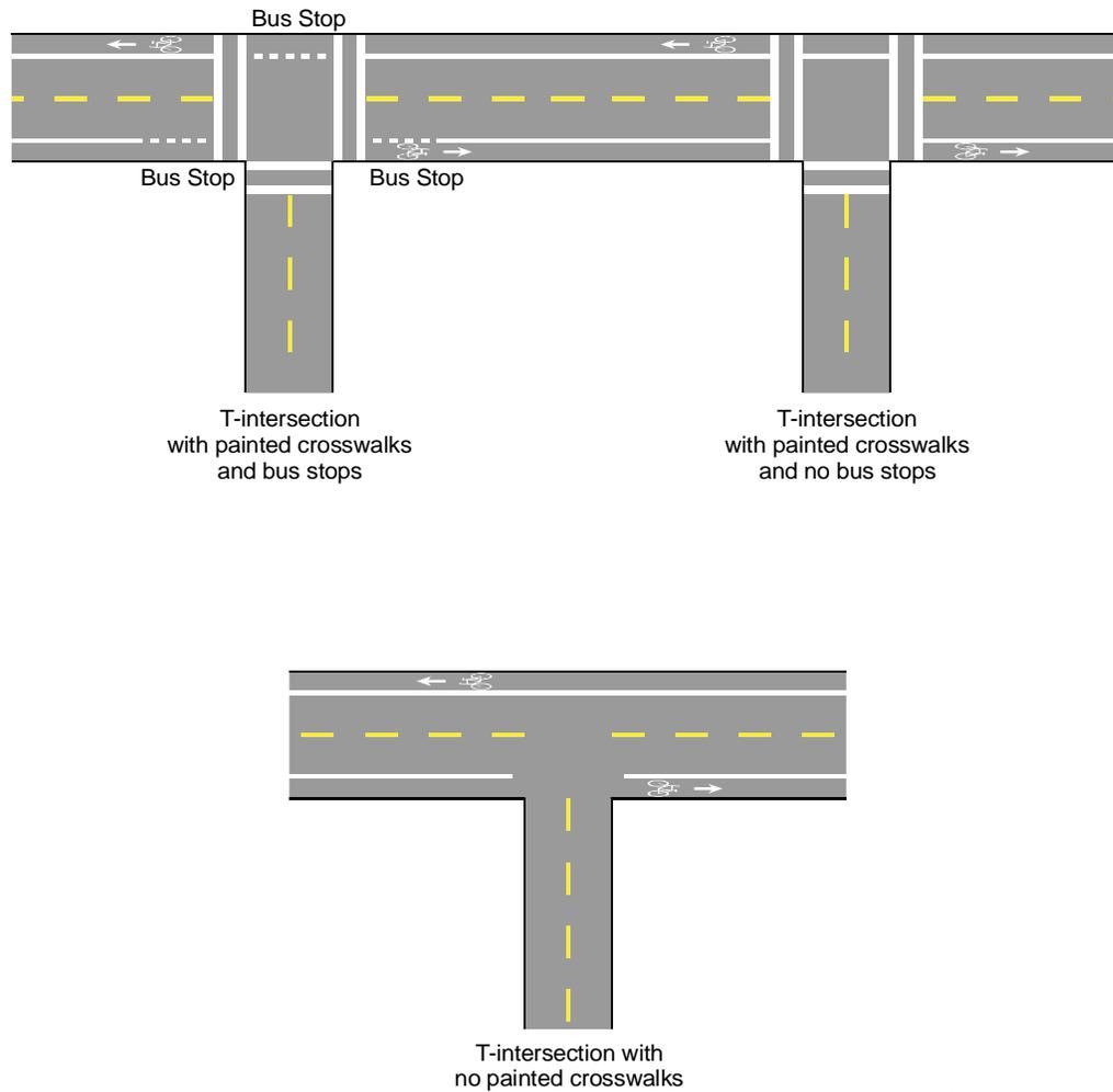
Figure 4-28. Example of Bicycle Lane Marking at T-Intersections.<sup>9</sup>
