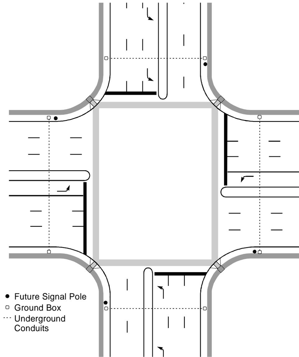
Figure 8-5. Intersection Design to Accommodate Traffic Signal Installation.
