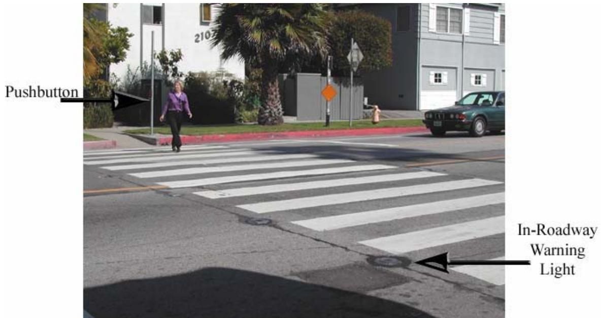
Figure 7-28. Example of In-Roadway Warning Lights.
