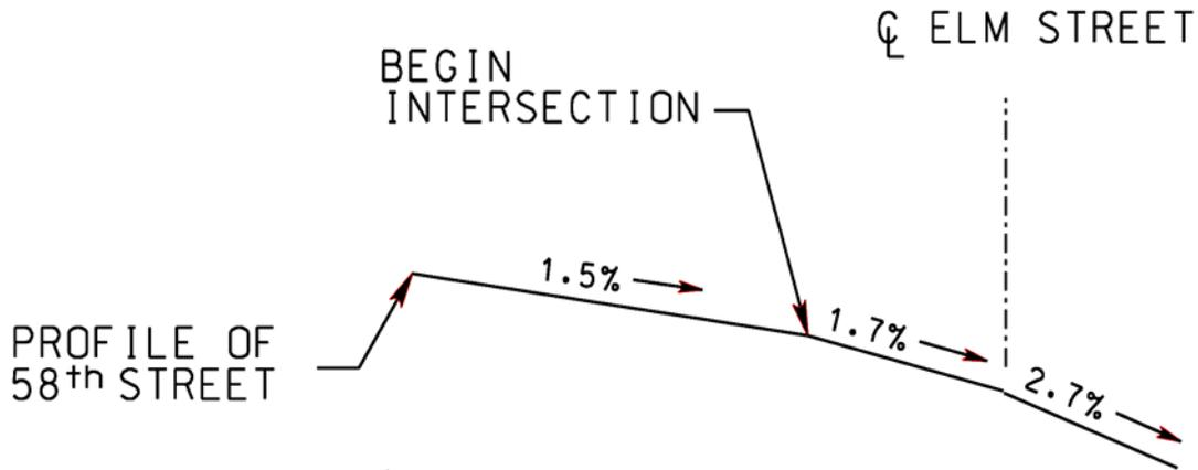
Figure 3-29. Profile of 58<sup>th</sup> Street as It Meets Elm Street's Cross Slope.
