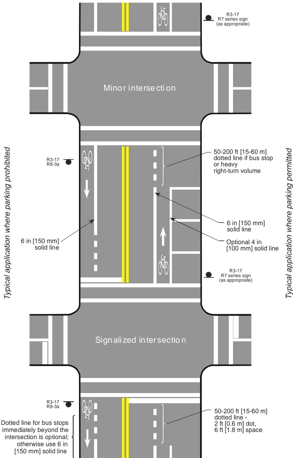
Figure 4-27. Bicycle Lane Marking Examples.<sup>9</sup>
