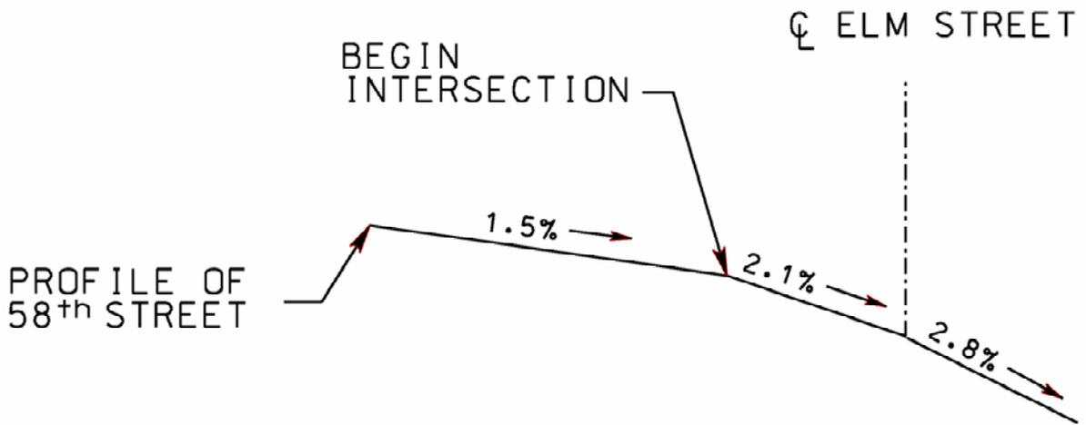
Figure 3-31. Revised Profile of 58<sup>th</sup> Street as It Meets Elm Street's Cross Slope.
