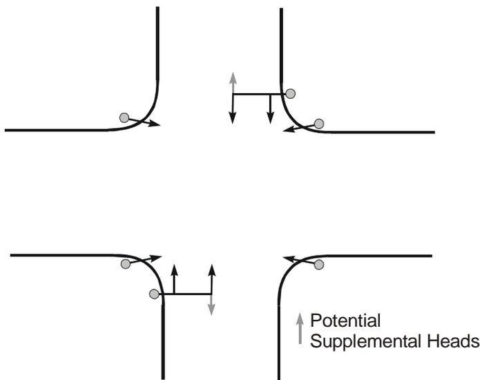
Figure 8-9. Typical Mast Arm Mounting.<sup>7</sup>
