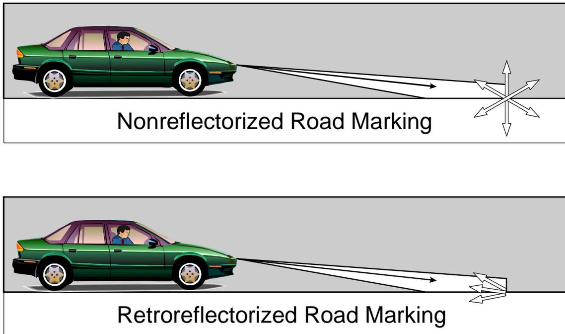
Figure 9-3. Light Reflection Characteristics.<sup>3</sup>
