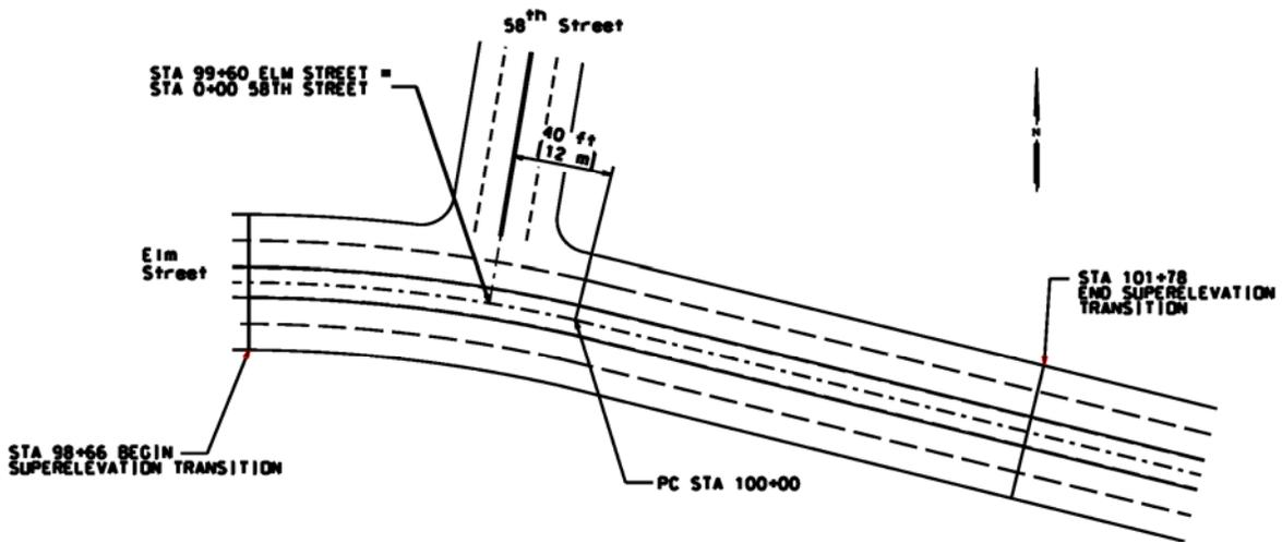
Figure 3-30. Revised Layout of Superelevation Transition.
