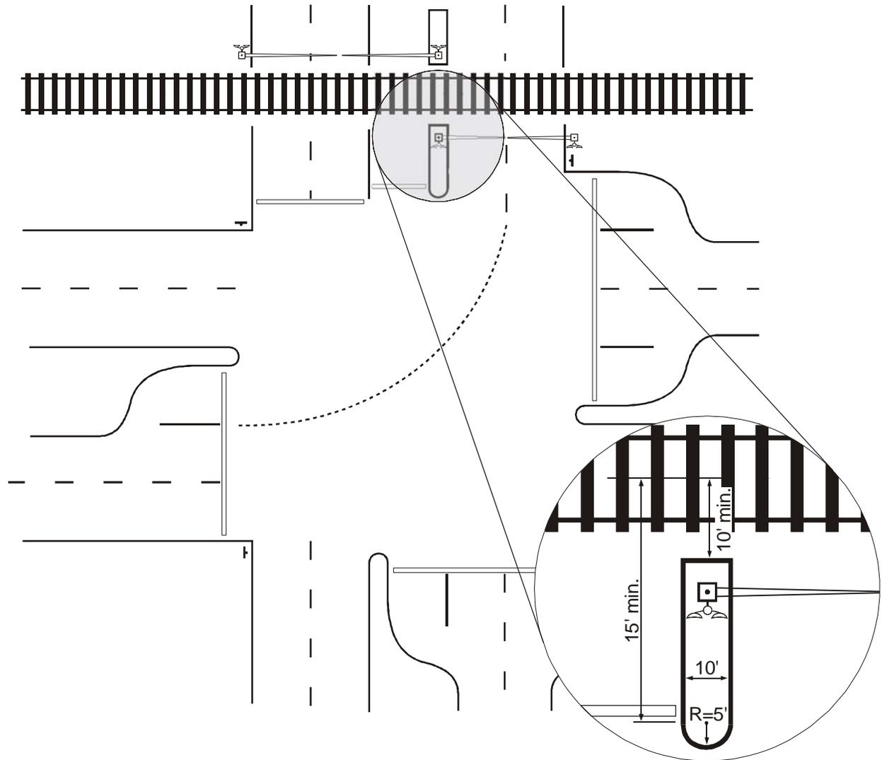
Figure 11-8. Channelizing Island at Railroad Grade Crossing.<sup>8</sup>
