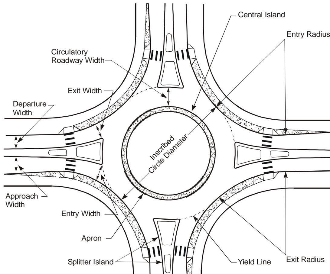
Figure 1-3. Example of Roundabout.<sup>1</sup>
