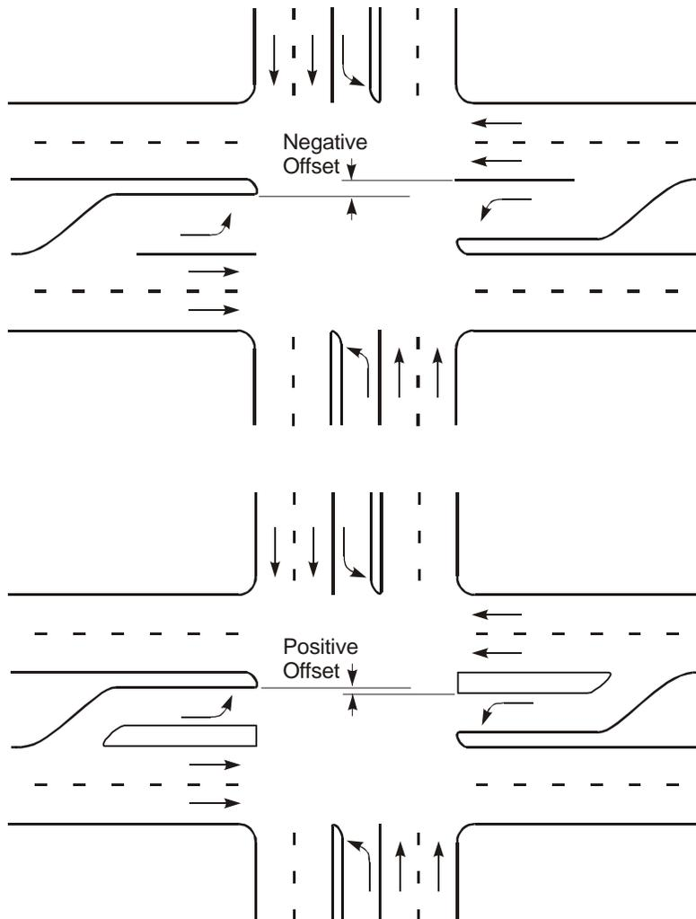
Figure 4-4. Negative and Positive Offsets of Left-Turn Lanes.<sup>4</sup>
