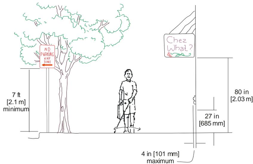
Figure 10-1. Sidewalk Free of Protruding Objects.<sup>5</sup>
