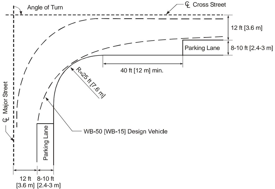
Figure 3-8. Effective Radius with Parking Restriction.<sup>4</sup>
