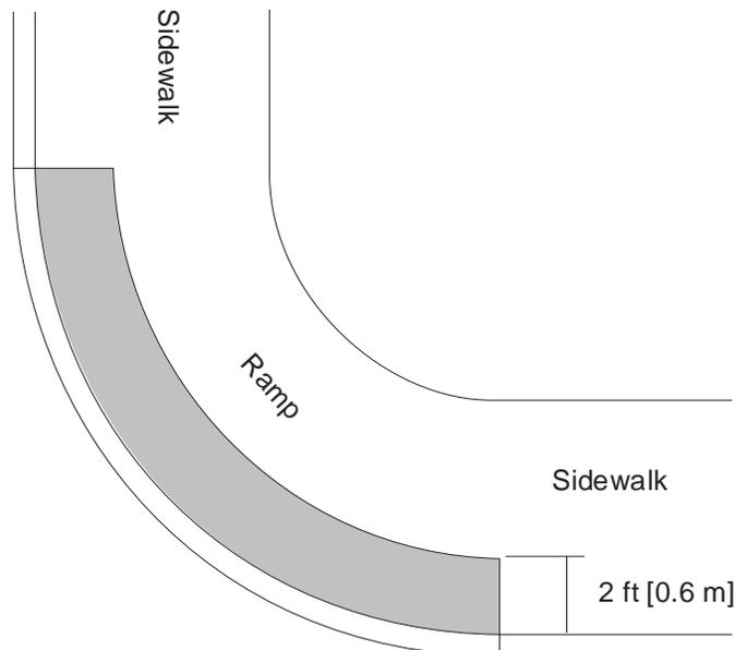
Figure 7-8. Example of a Blended Transition.
