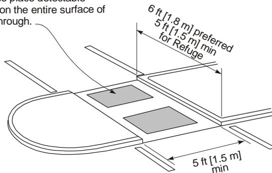
Figure 4-26. Cut through at Raised Median.<sup>15</sup>
