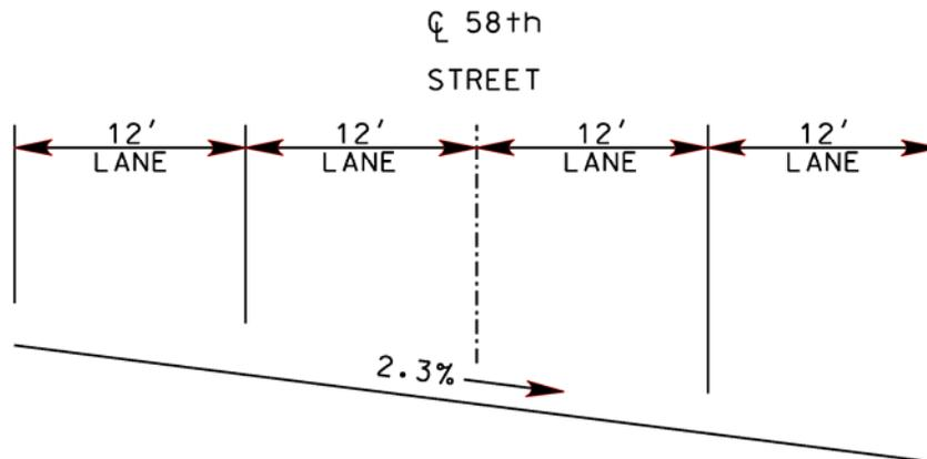
Figure 3-33. Cross Section of 58<sup>th</sup> Street Entering Intersection (STA 0+31).
