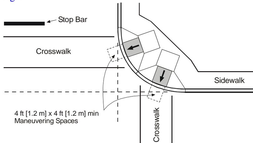
Figure 7-2. Perpendicular Curb Ramp.
