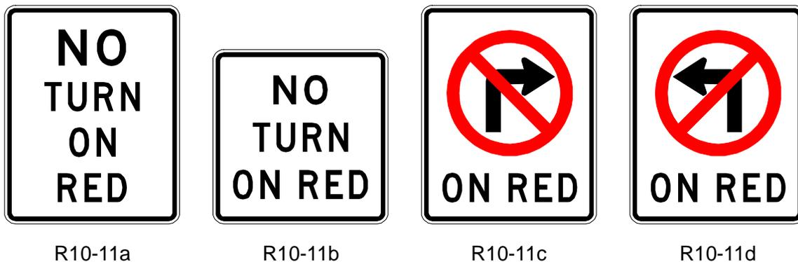
Figure 10-16. Signing for Prohibited Right Turn on Red (*TMUTCD*).
