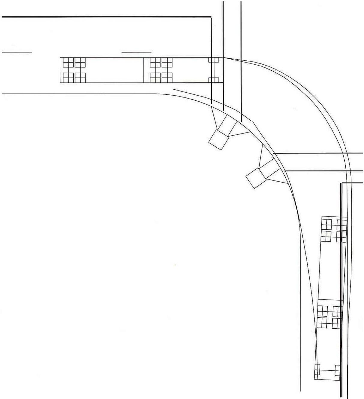
Figure 3-38. WB-50 [WB-15] on 50-ft [15 m] Radius.
