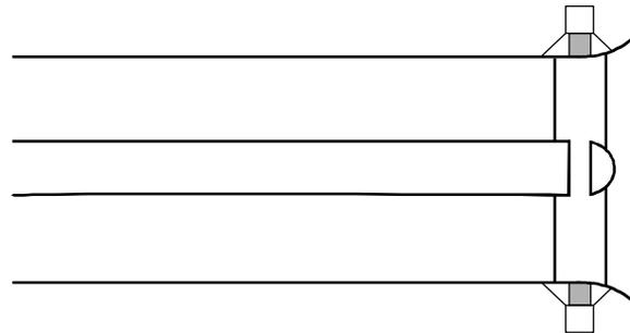
*Figure 4-13. Raised Median Channelization.<sup>8</sup>*
