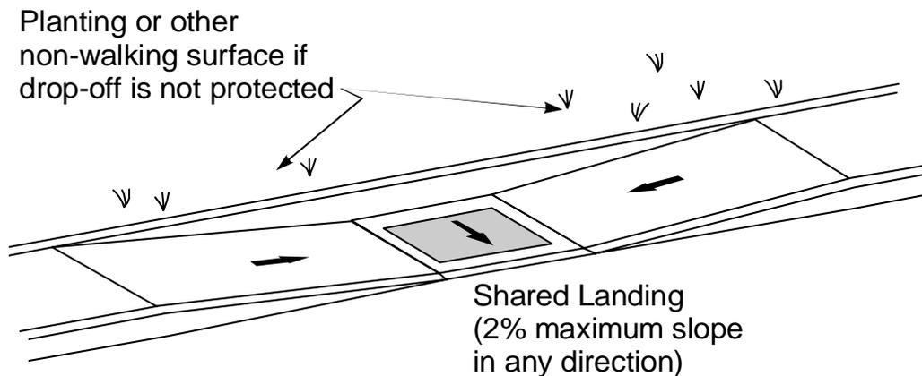
Figure 7-4. Parallel Curb Ramps.
