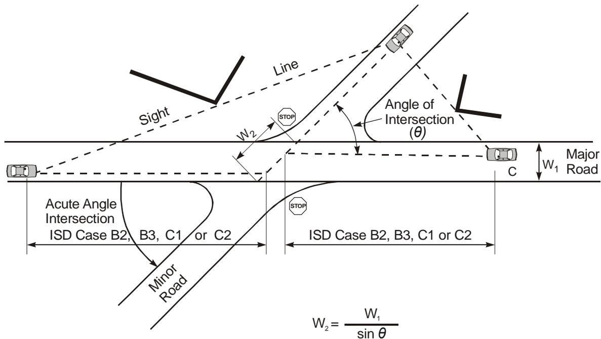
Figure 3-3. Sight Triangles at Skewed Intersections.<sup>3</sup>
