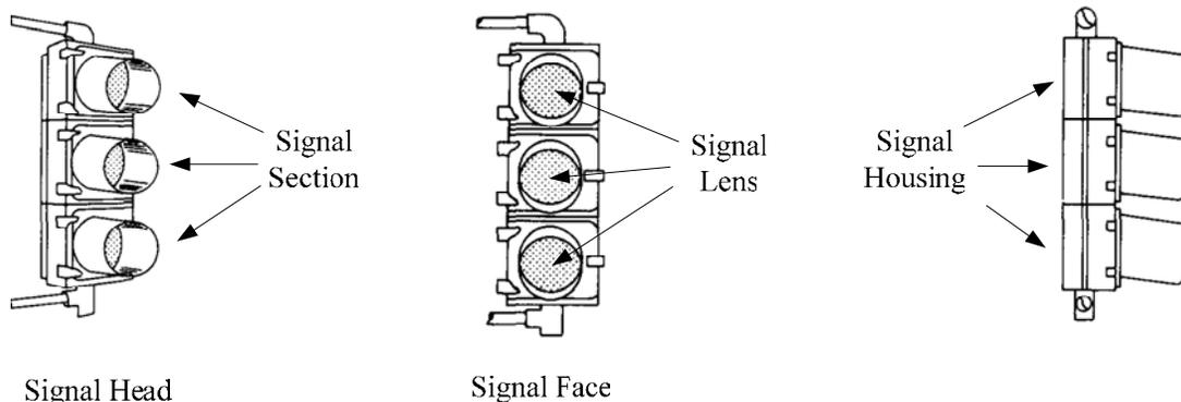
Figure 8-1. Components of a Three-Section Traffic Signal Head.
