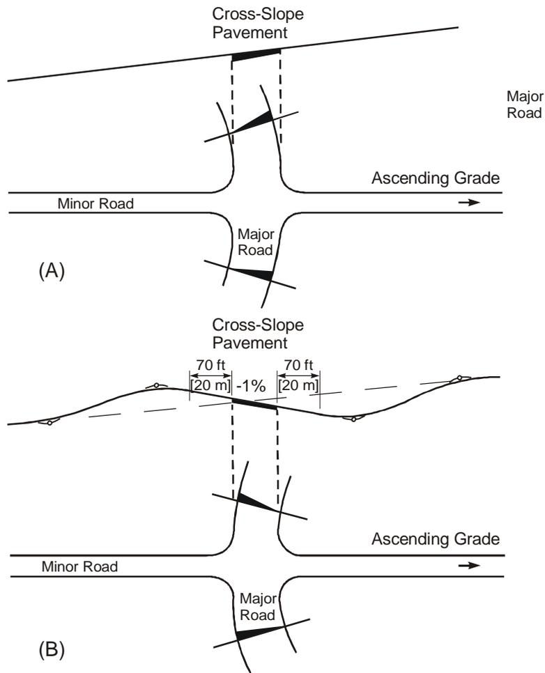
Figure 3-12. Coordination of Vertical Alignments on Horizontal Curves.<sup>10</sup>
