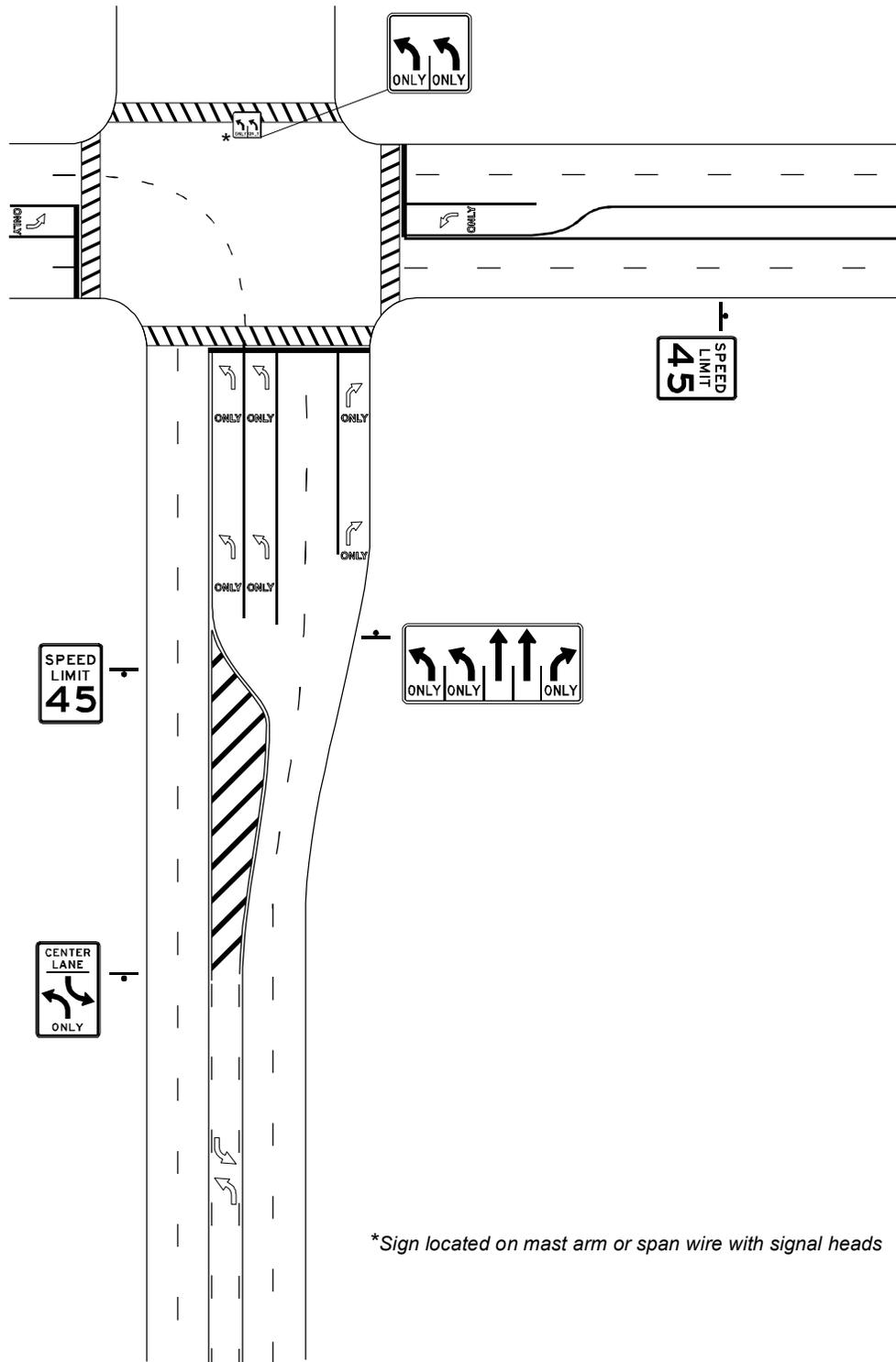
Figure 10-1. Example of Signs and Pavement Markings for Intersection with Dual Left-Turn Lanes and Single Right-Turn Lanes.
