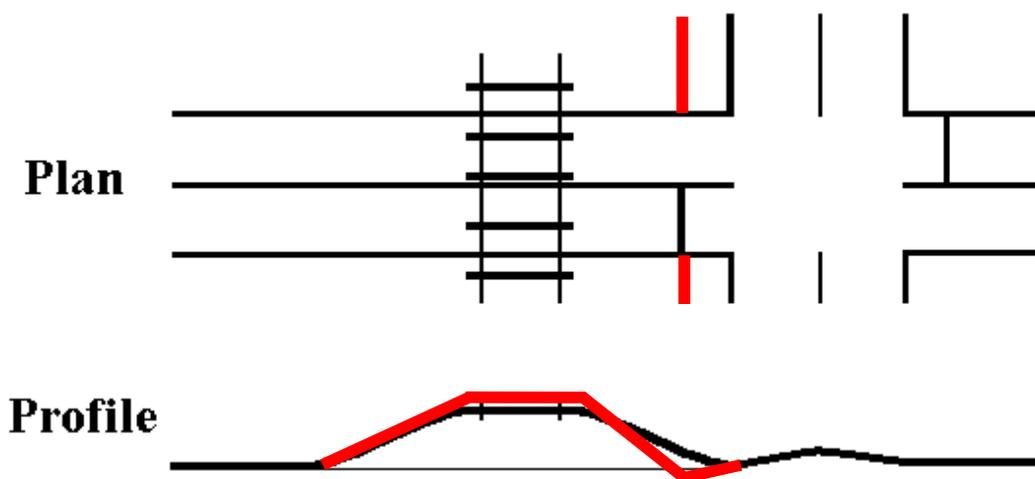
Figure 11-2. Effect of Widening Roadway and Raising Railroad on Grades.
