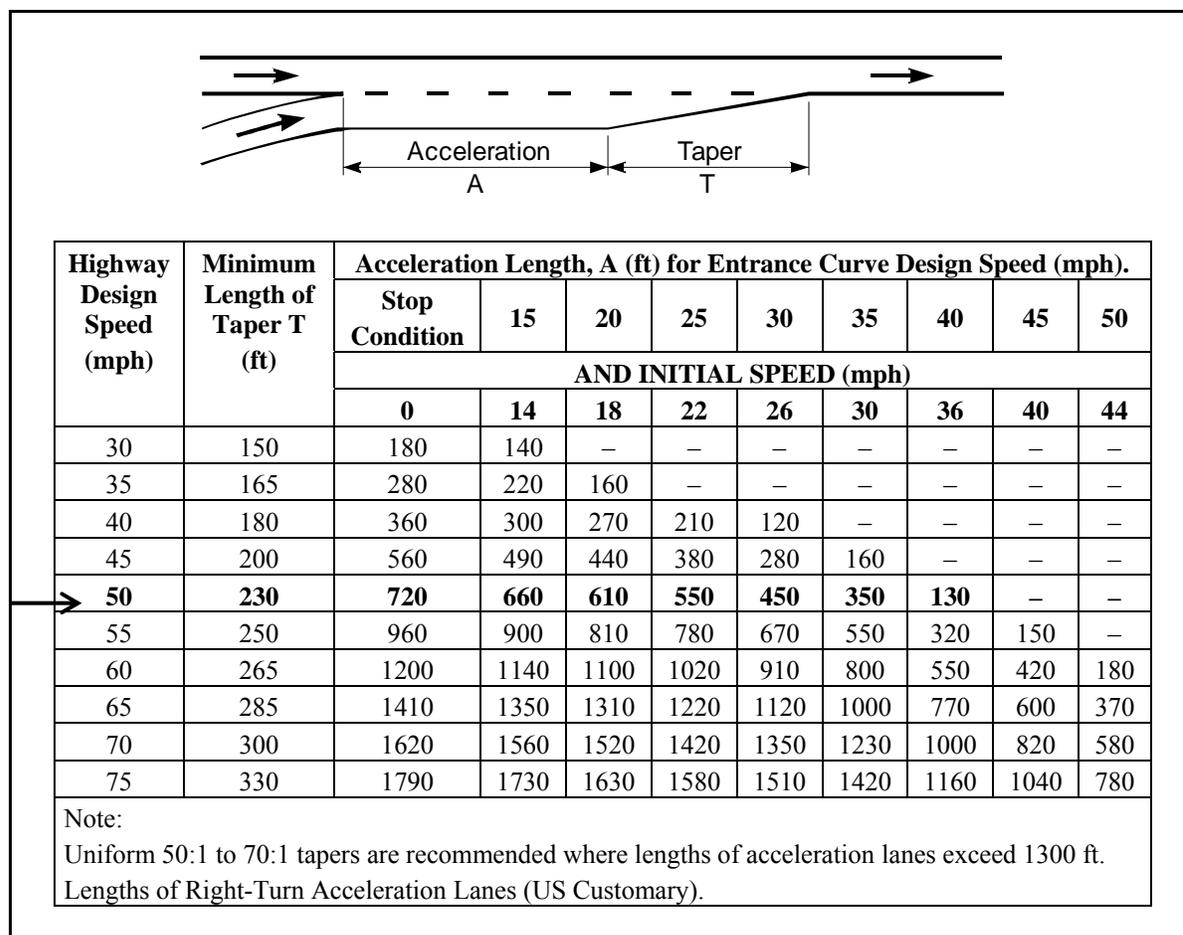
Figure 4-2. Length of Right-Turn Acceleration Lanes<sup>1</sup> (Reproduced from *Roadway Design Manual* Figure 3-10 <link>).
