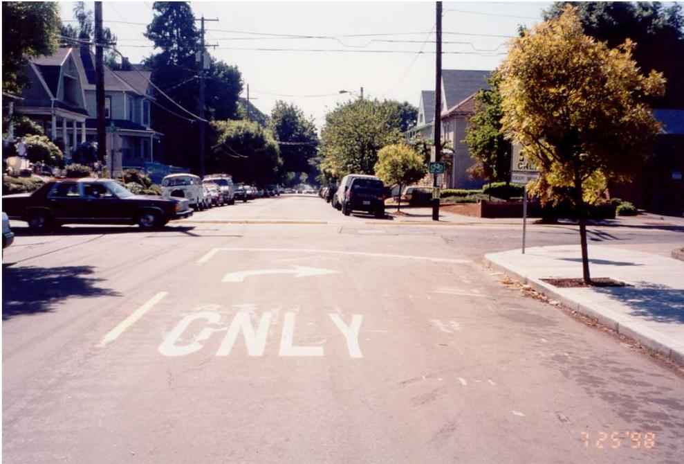
Figure 9-11. Example of Right Turn Only Word Pavement Markings.
