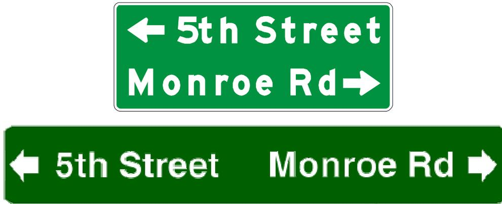
Figure 10-7. Signing for Different Street Names for Different Directions of Travel, Two Examples.
