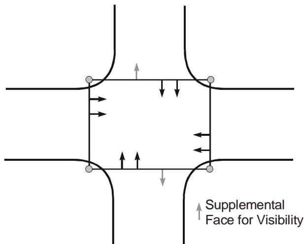
Figure 8-7. Span Wire Mounting: Box Span.<sup>7</sup>
