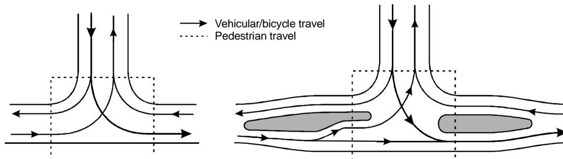
Figure 1-3. Typical Three-Leg Intersection.
