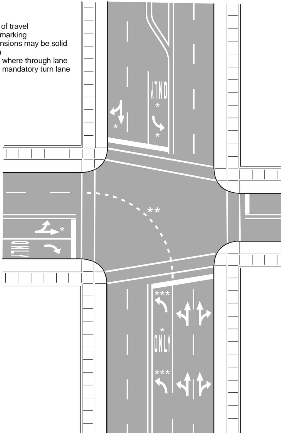
Figure 9-10. Typical Lane Use Control Word and Symbol Markings.
