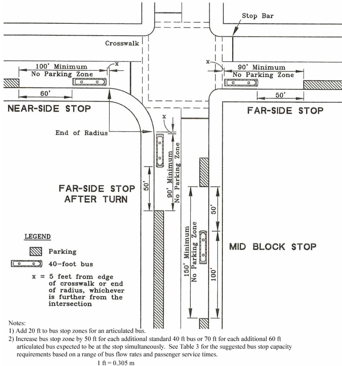
Figure 5-25. Typical Types of and Dimensions for On-Street Bus Stops.<sup>16</sup>
