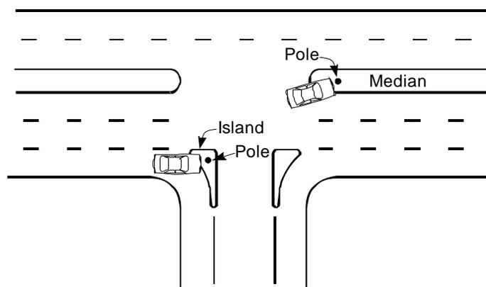
Figure 5-9. Inappropriate Location of Poles within a Traffic Island or Median.<sup>11</sup>
