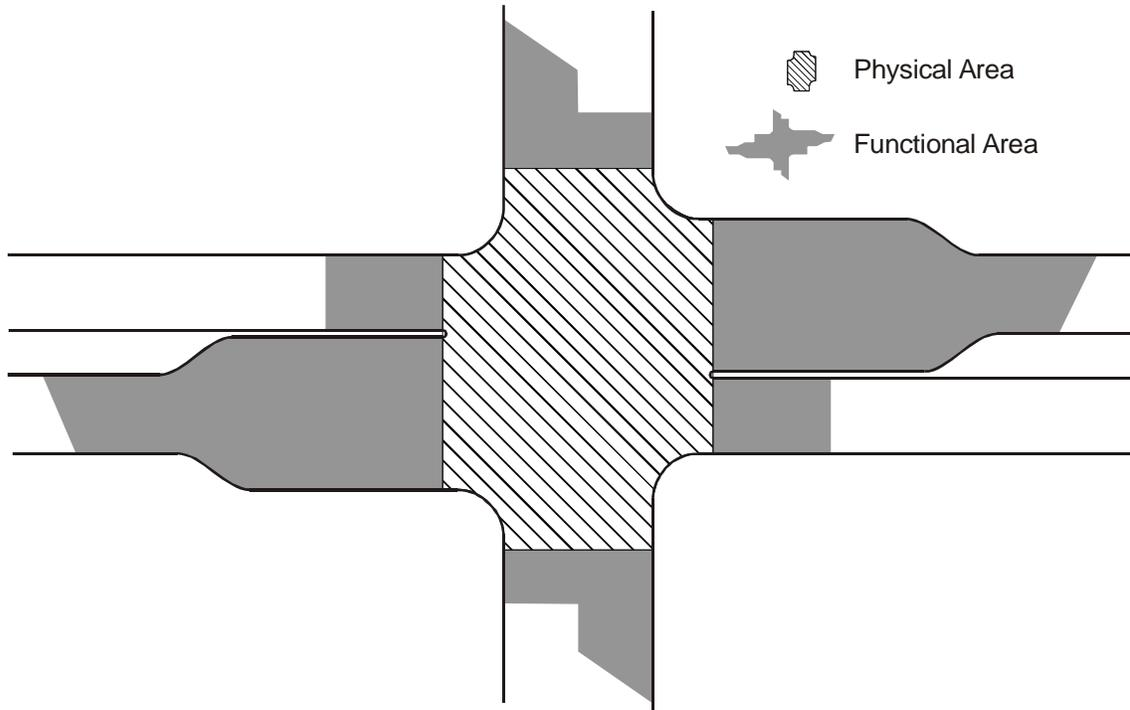
Figure 1-7. Functional Area of an Intersection.<sup>18</sup>
