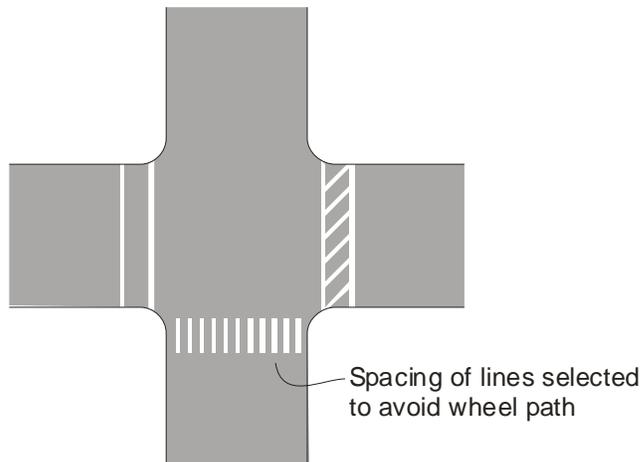
Figure 9-7. Crosswalk Marking Options.<sup>1</sup>
