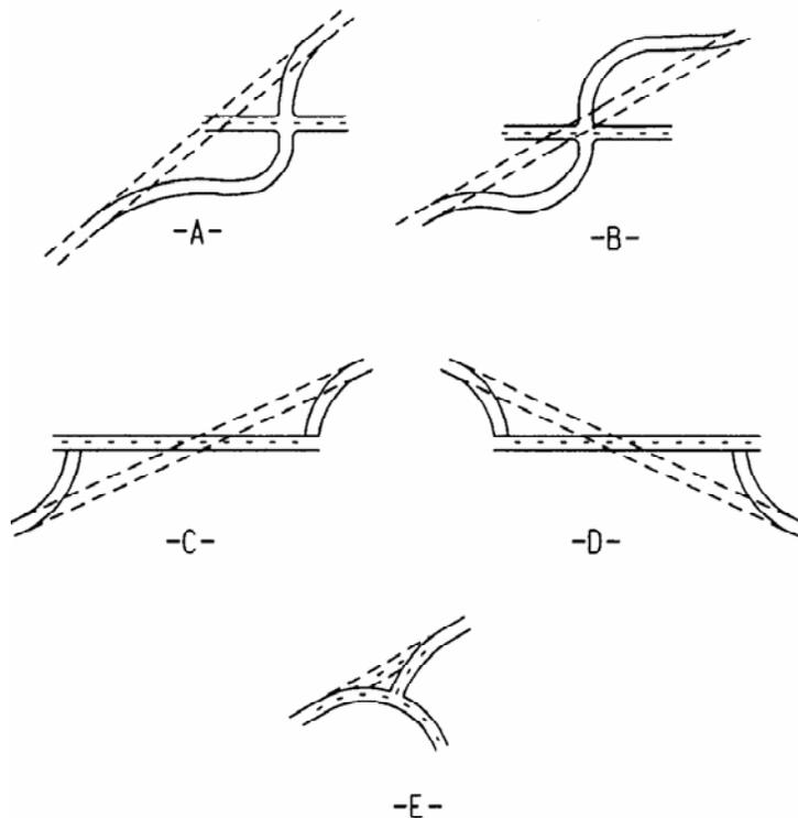
Figure 3-10. Realignment Options at Intersections.<sup>3</sup>
