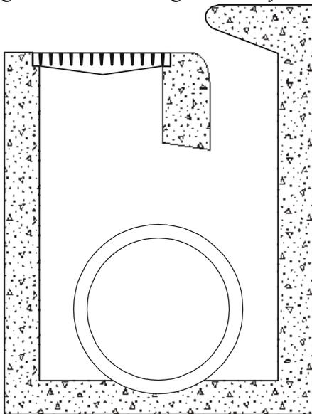
Figure 6-13. Example of Combination Inlet.
