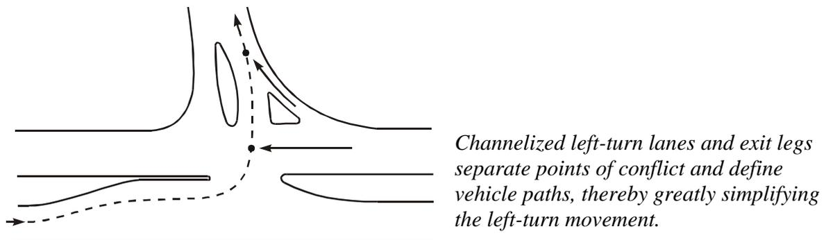
Figure 4-10. Channelized Left-Turn Lanes and Exit Legs.<sup>8</sup>
