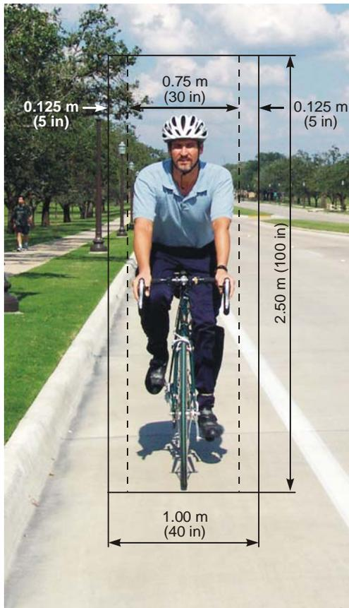
Figure 2-3. *Bicyclist Operating Space (Based on Data in the AASHTO Guide for the Development of Bicycle Facilities*<sup>9</sup>).
