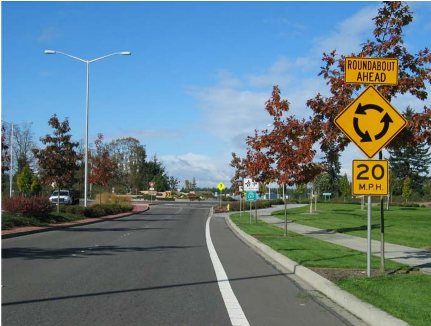
Figure 1-6. Roundabout Advance Warning Sign Example.
