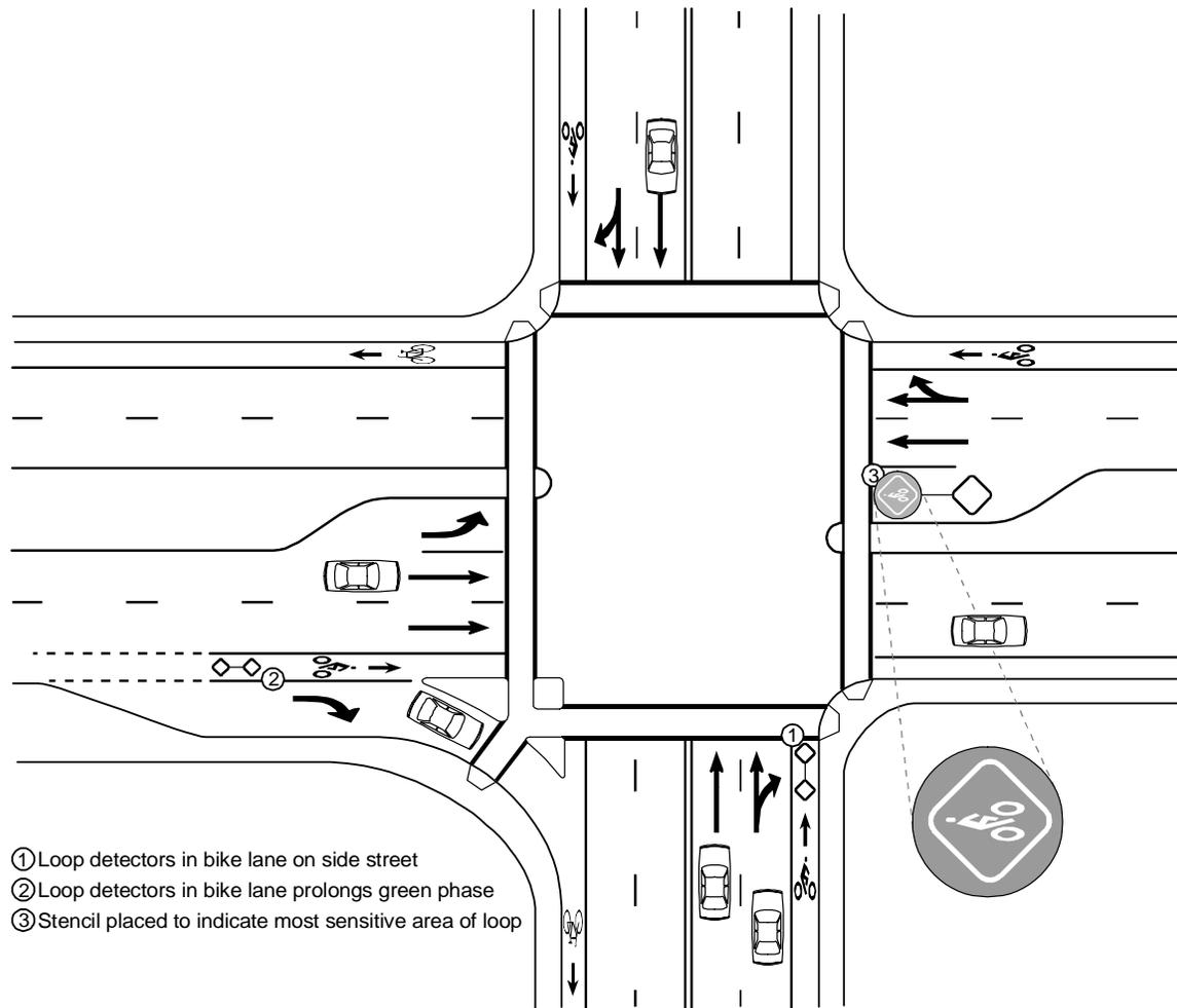
Figure 8-14. Signalized Intersection Sensitive to Bicycles (Based on Oregon Bicycle and Pedestrian Plan).<sup>19</sup>
