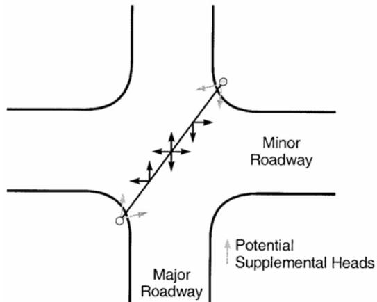
Figure 8-6. Span Wire Mounting: Two-Pole Simple Span.<sup>7</sup>
