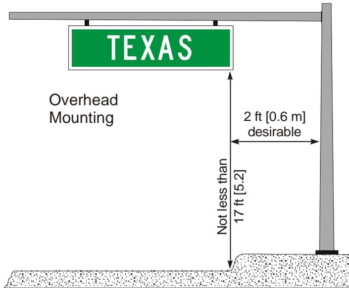
Figure 10-4. Overhead Street Name Sign on Mast Arm Post.
