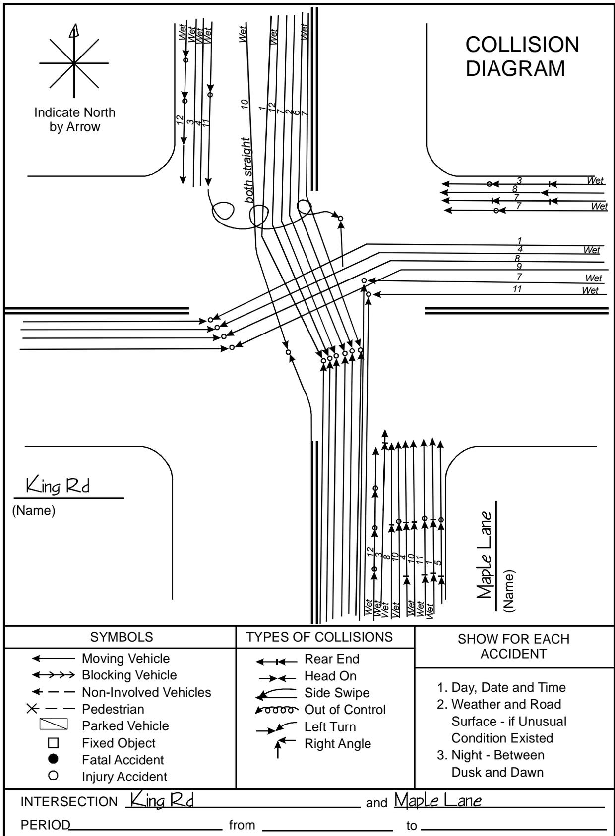
Figure 2-2. Collision Diagram.
