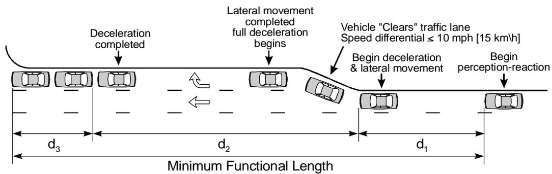
Figure 1-8. Elements of the Functional Area of an Intersection.<sup>18</sup>
