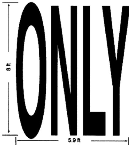
Figure 9-12. Typical Elongated Letters for Word Pavement Markings.
