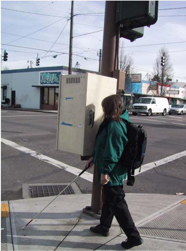
Figure 5-5. Protruding Controller Equipment.
