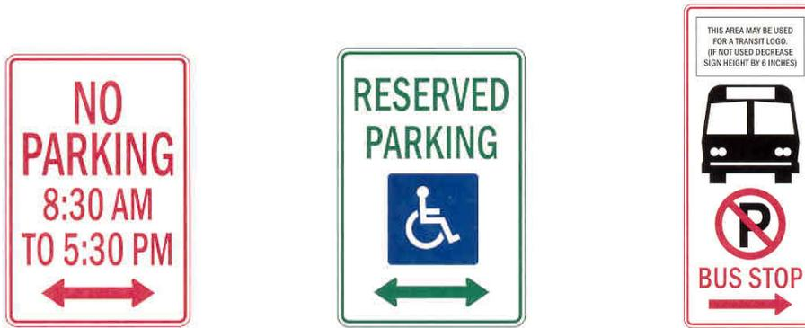
Figure 10-15. Parking and Bus Sign Examples from TMUTCD.
