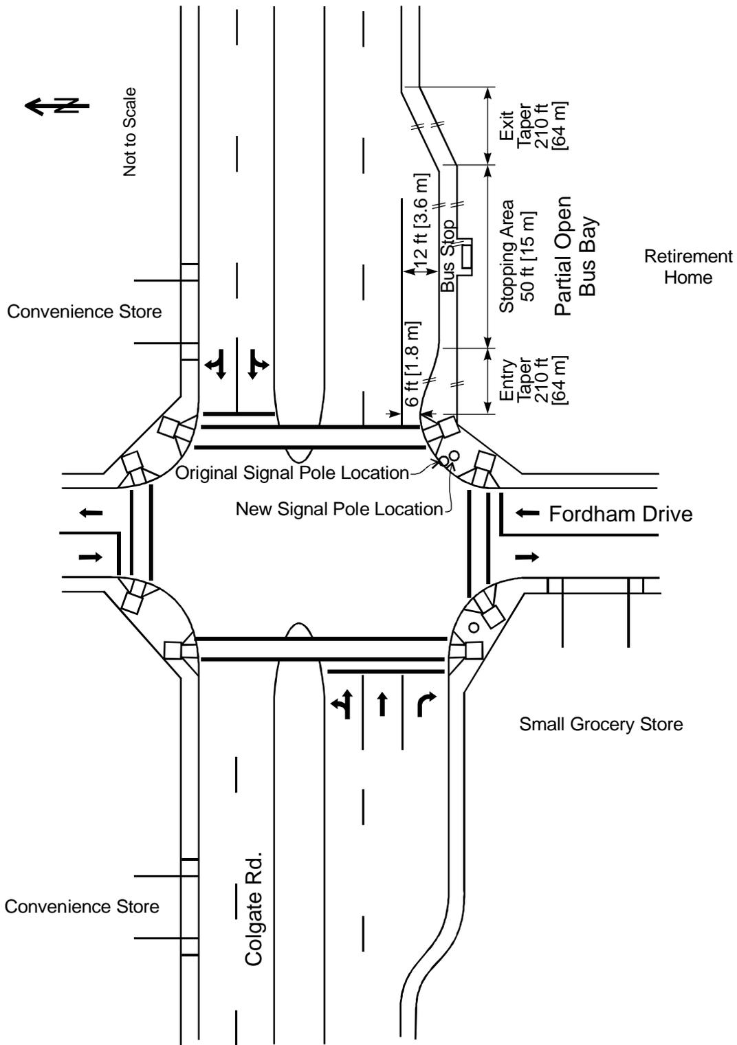
Figure 5-4. Design of Bus Stop and Adjoining Sidewalk.
