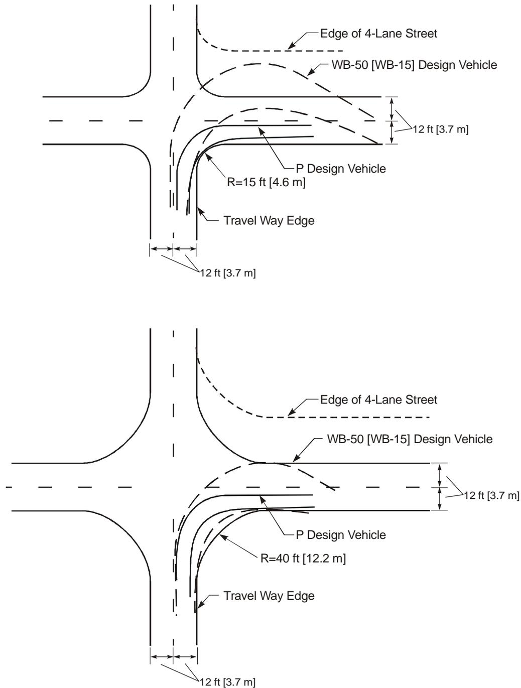
Figure 3-6. Effect of Curb Return Radius on Right Turning Paths ( $R=15\text{ ft [4.6 m]}$  and  $R=40\text{ ft [12.2 m]}$ ).<sup>3</sup>
