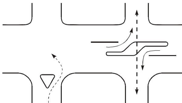
*Raised traffic islands can block through movements or undesirable turning movements without hindering other intersection movements.*
