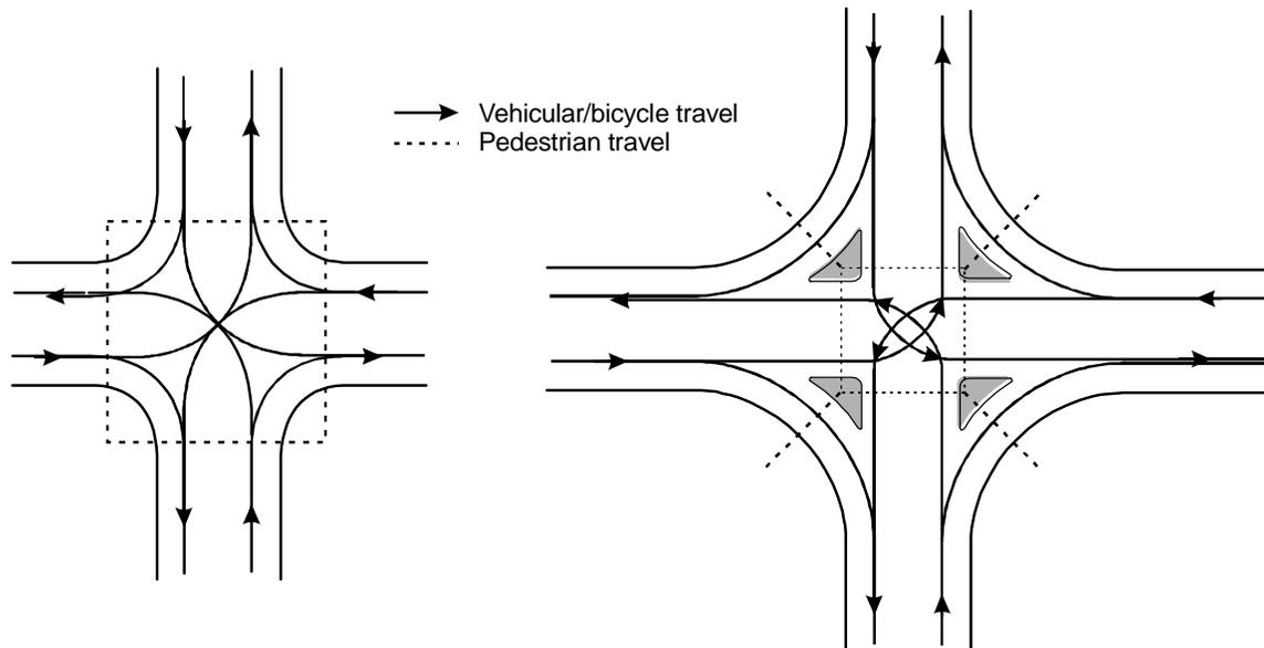
Figure 1-5. Typical Four-Leg Intersections.
