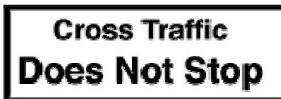
*Figure 10-17. Supplemental Panel to Mount below Stop Sign.*
