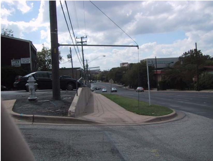
*Figure 5-28. Guy Wire to Accommodate Pedestrian Movement.*
