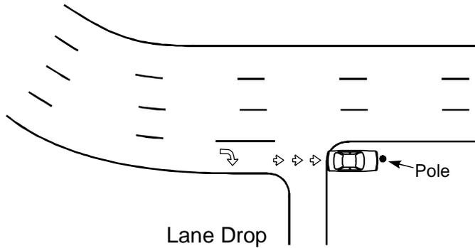
Figure 5-7. Exposure of Vehicle to Utility Pole Downstream of Lane Drop.<sup>11</sup>
