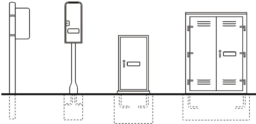
Figure 8-11. Types of Controller Cabinet Mountings.<sup>7</sup>
