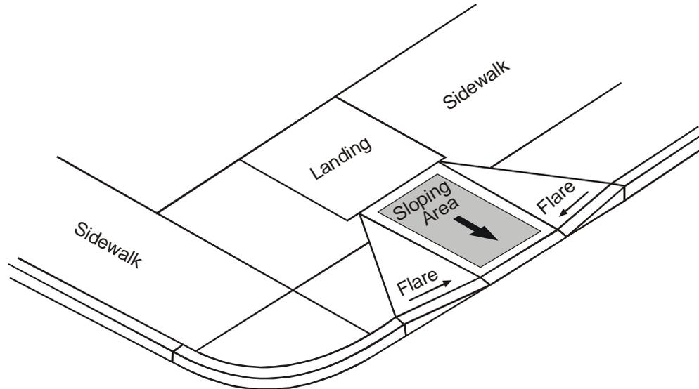
Figure 7-1. Components of a Curb Ramp.
