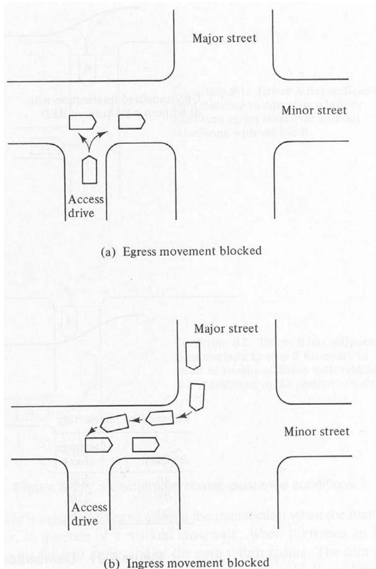
Figure 11-10. Driveways Blocked by Intersection Queue.<sup>2</sup>
