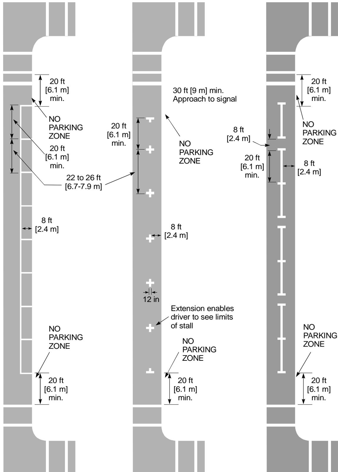
Figure 9-9. Typical Parking Space Markings.<sup>1</sup>
