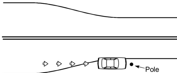
Figure 5-8. Placement of Pole Downstream of Roadway Narrowing.<sup>11</sup>
