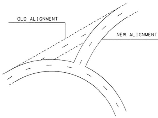
*Figure 3-4. Realignment of Tangent Roadway at Intersection.<sup>3</sup>*
