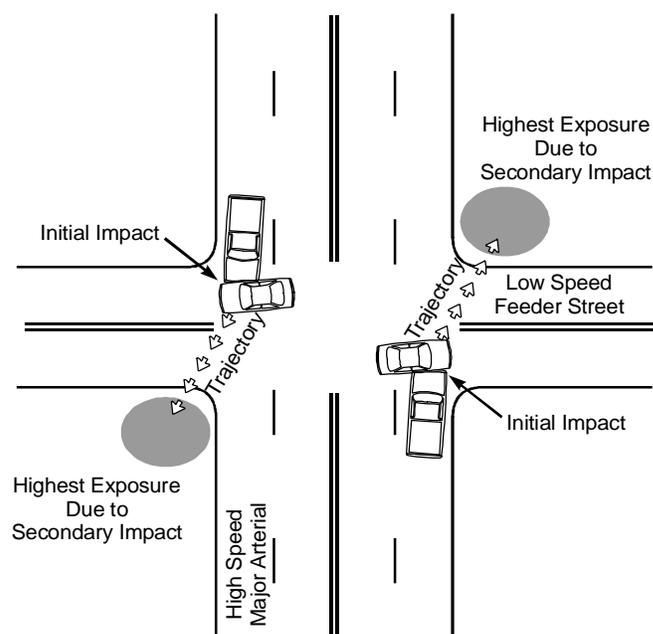
Figure 5-10. Intersection Zones Having Highest Exposure to Secondary Collisions.<sup>11</sup>
