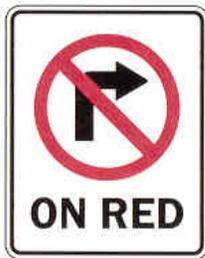
*Figure 10-11. Turn Prohibition Example from TMUTCD.<sup>1</sup>*
