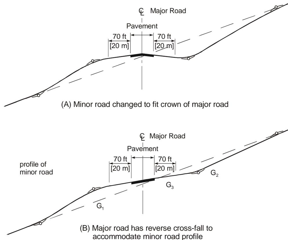
Figure 3-11. Coordination of Vertical Alignments on Horizontal Tangent.<sup>10</sup>
