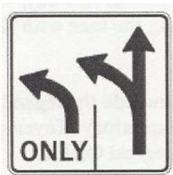
Figure 10-12. Intersection Lane Control Sign Example from the *TMUTCD*.<sup>1</sup>
