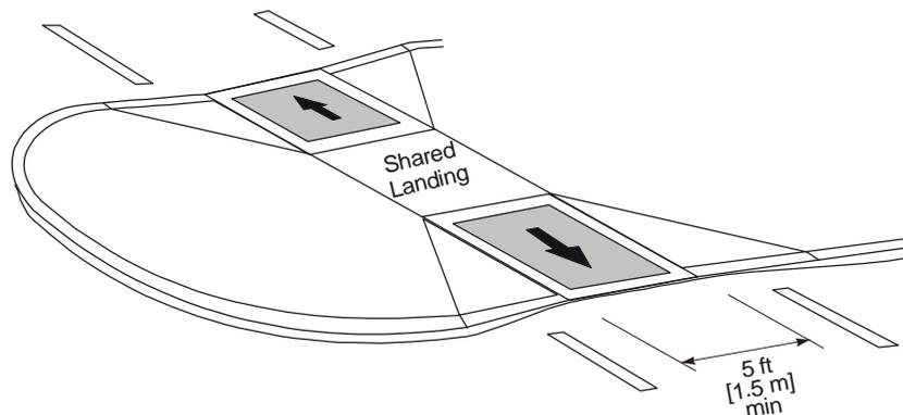
Figure 4-25. Curb Ramp at Median Islands.<sup>15</sup>
