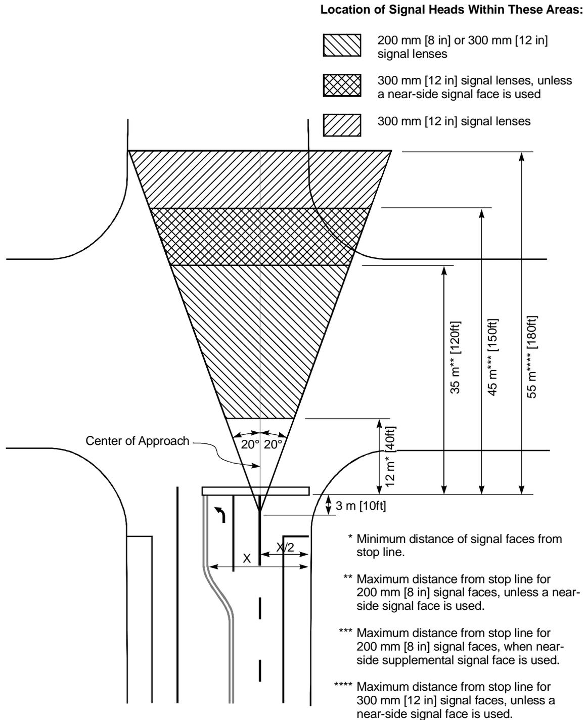
Figure 8-2. Federal MUTCD Horizontal Location of Signal Faces.<sup>6</sup>
