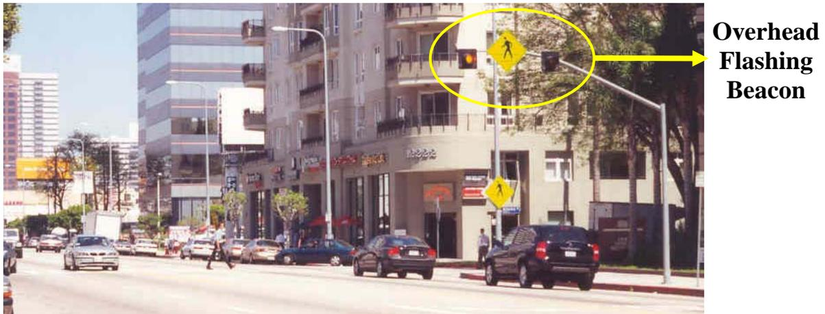
Figure 7-29. Example of Overhead Flashing Beacon.
