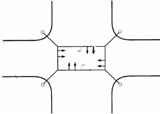
Figure 8-8. Span Wire Mounting: Cable Box.<sup>7</sup>
