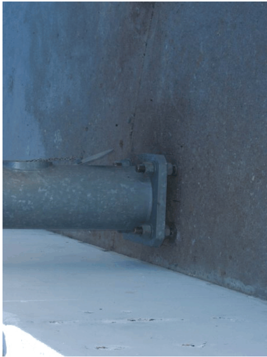
Figure 62. Luminaire Pole Mounted Behind Single-Slope Concrete Barrier, Test No. ZO1-3
