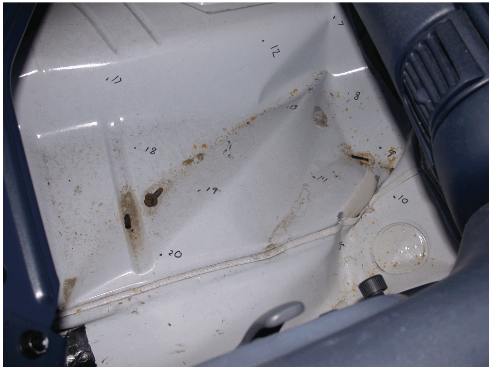
Figure 55. Occupant Compartment Deformation, Test No. ZOI-2
