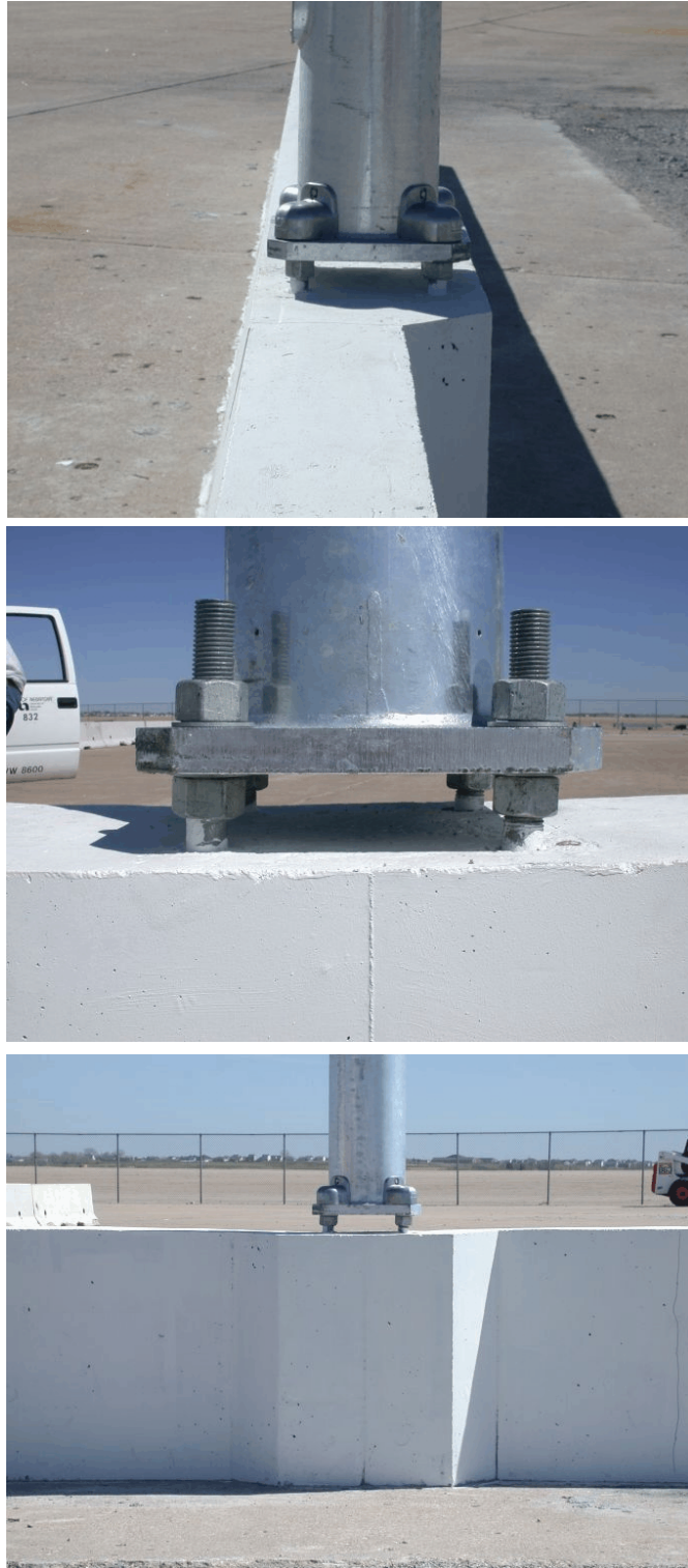
Figure 11. Luminaire Pole Attached to Single-Slope Concrete Barrier, Connection Details for Test Nos. ZOI-1 and ZOI-2
