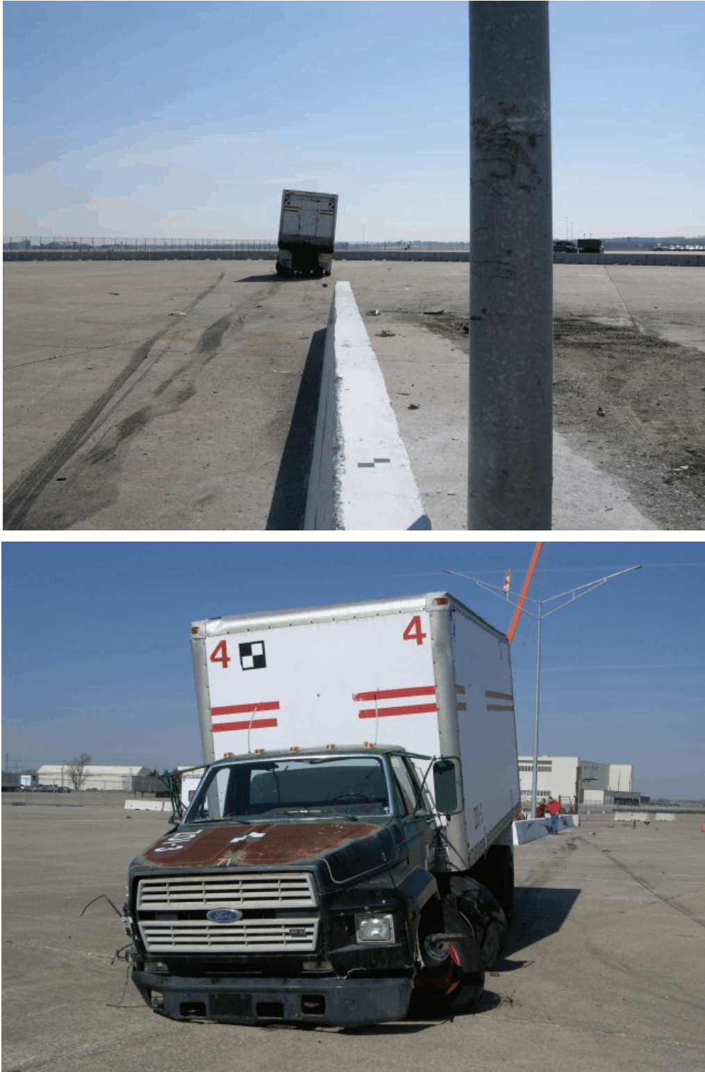
Figure 71. Vehicle Final Position and Trajectory Marks, Test ZOI-3
