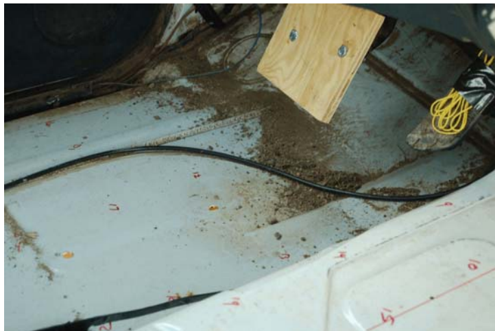
Figure 38. Occupant Compartment Deformation, Test CS-2
