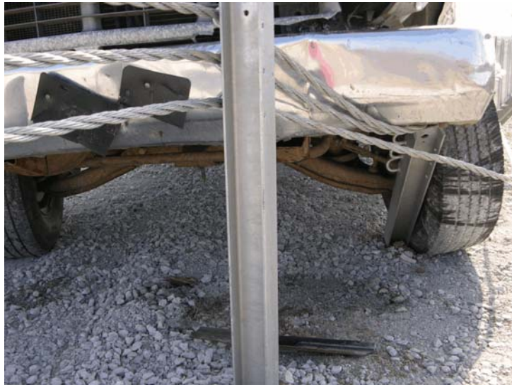
Figure 36. Vehicle Damage, Test CS-2
