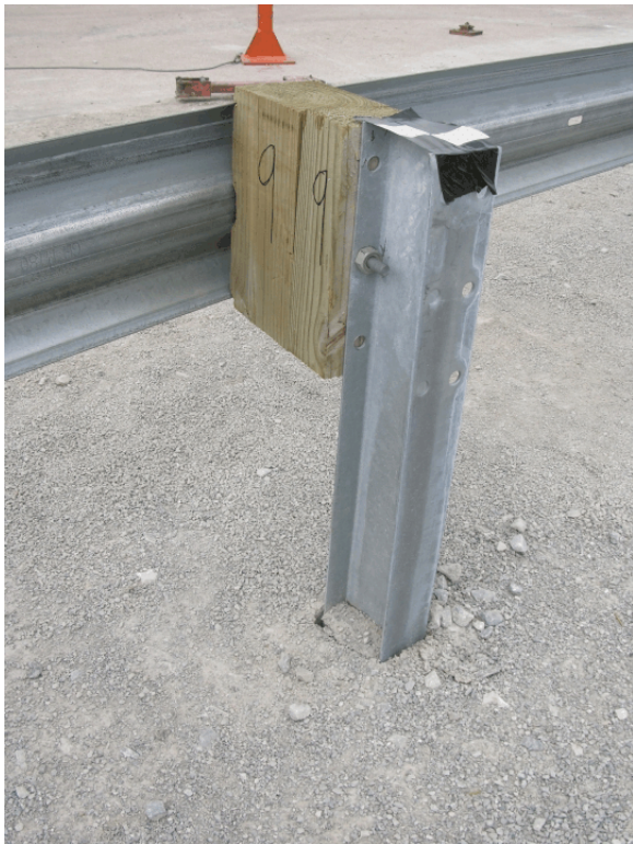
Figure 63. Post Nos. 9 and 10 Damage, Test FR-2
