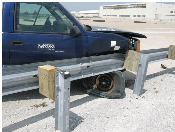
Figure 60. Vehicle Trajectory and Final Position, Test FR-2
