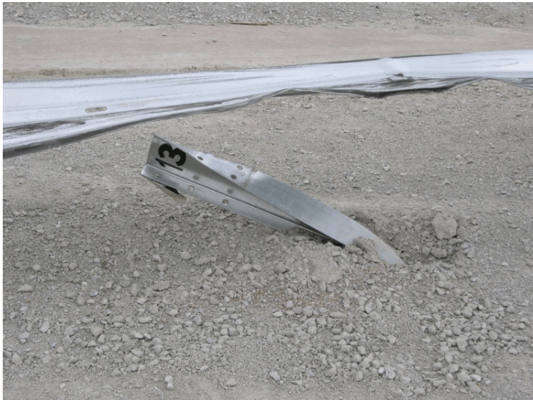
Figure 114. Post Nos. 13 and 14 Damage, Test FR-4
