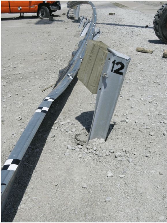
Figure 41. Post Nos. 11 and 12 Damage, Test No. FR-1
