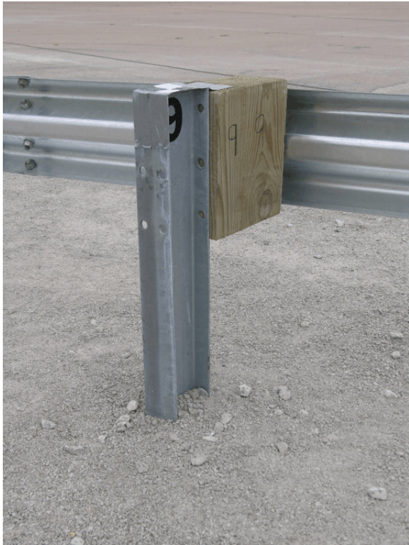
Figure 84. Post Nos. 9 and 10 Damage, Test FR-3
