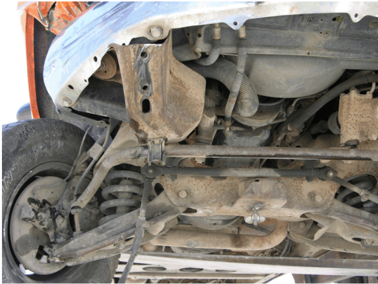
Figure 49. Vehicle Undercarriage Damage, Test FR-1
