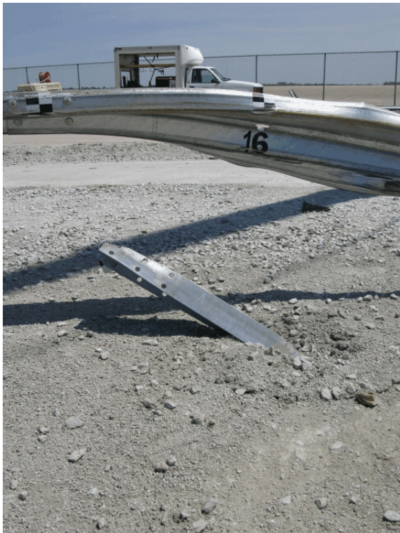
Figure 43. Post Nos. 15 and 16 Damage, Test No. FR-1
