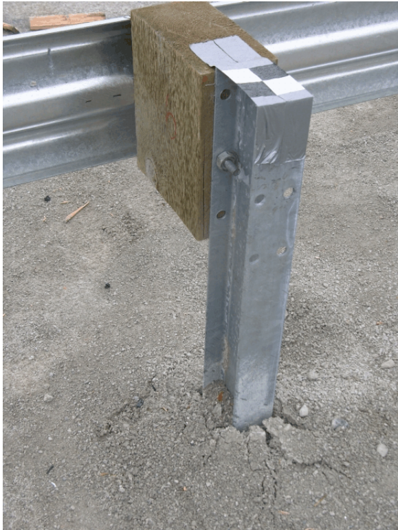
Figure 88. Post Nos. 16 and 17 Damage, Test FR-3
