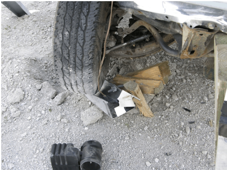
Figure 116. Post Nos. 17 and 18 Damage, Test FR-4
