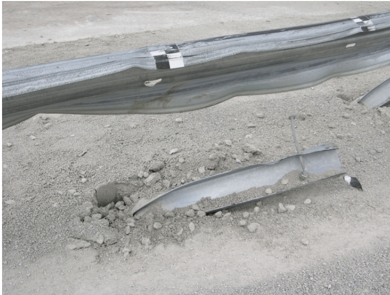
Figure 66. Post Nos. 13 and 14 Damage, Test FR-2
