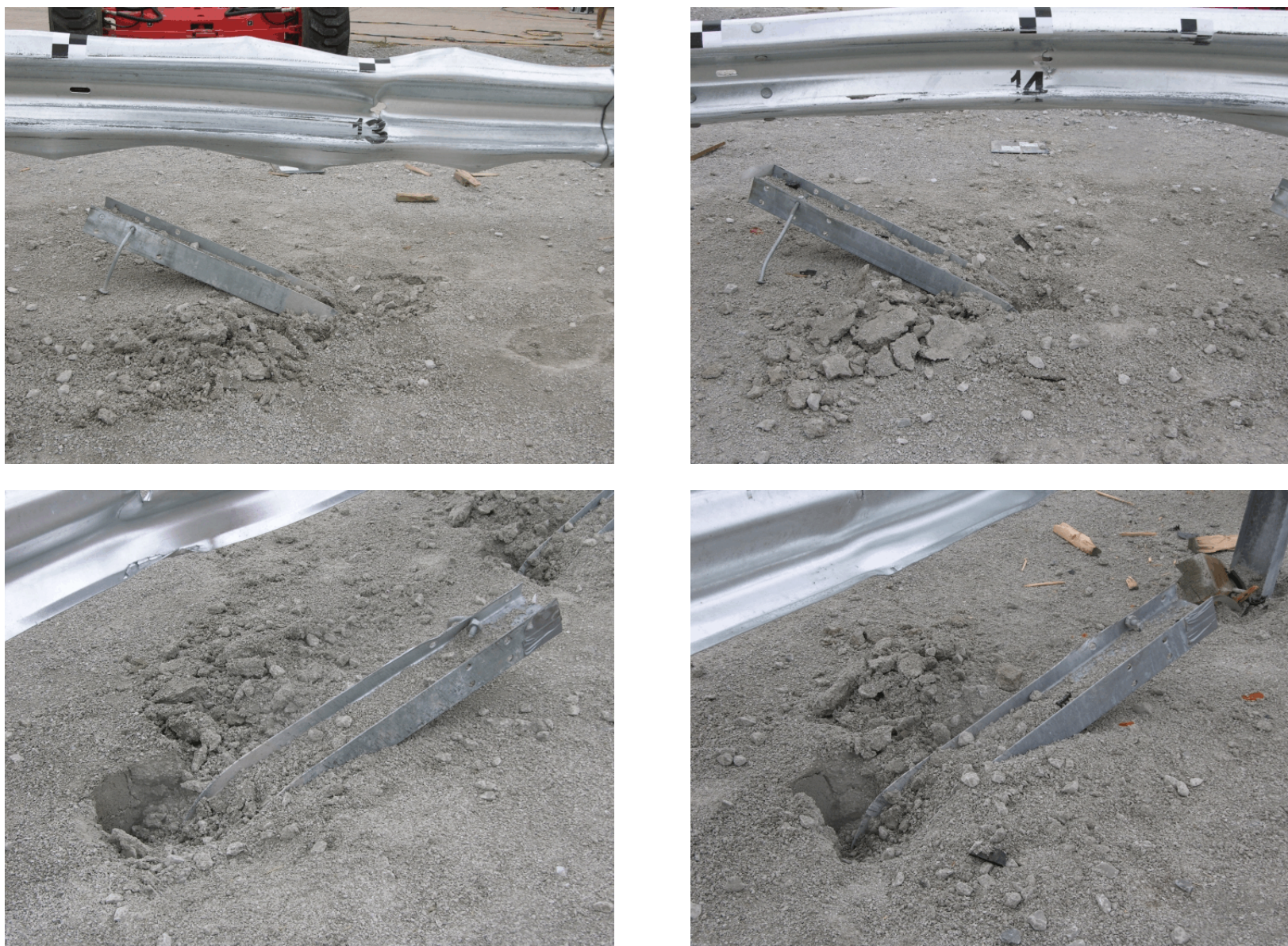
Figure 86. Post Nos. 13 and 14 Damage, Test FR-3
