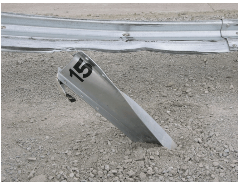
Figure 115. Post Nos. 15 and 16 Damage, Test FR-4
