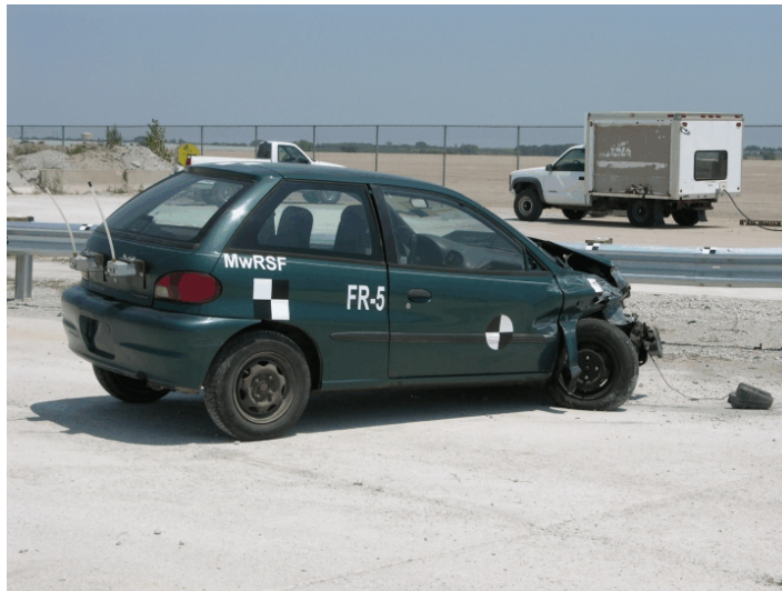
Figure 141. Vehicle Damage, Test FR-5
