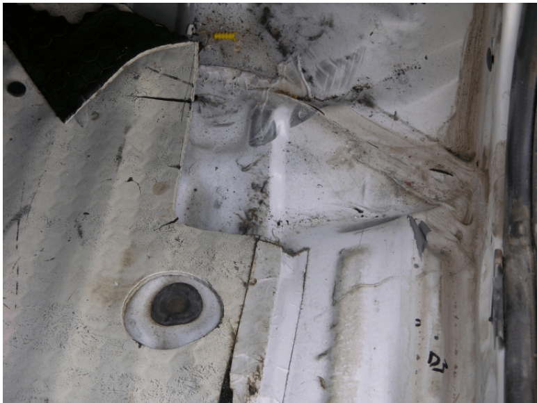
Figure 96. Occupant Compartment Damage, Test FR-3
