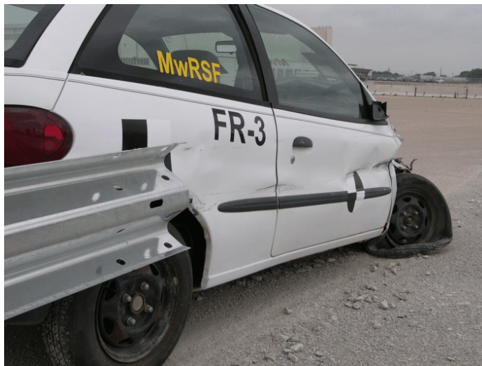
Figure 92. Vehicle Damage, Test FR-3
