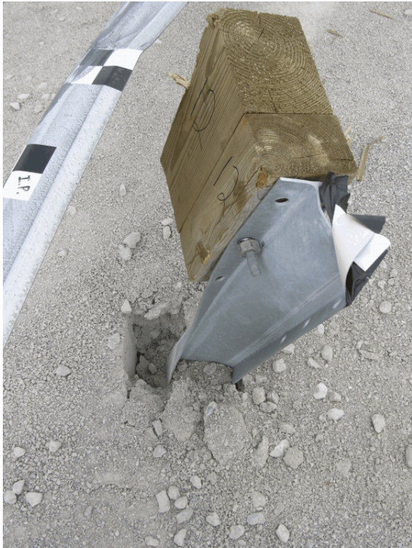
Figure 65. Post No. 12 Damage, Test FR-2
