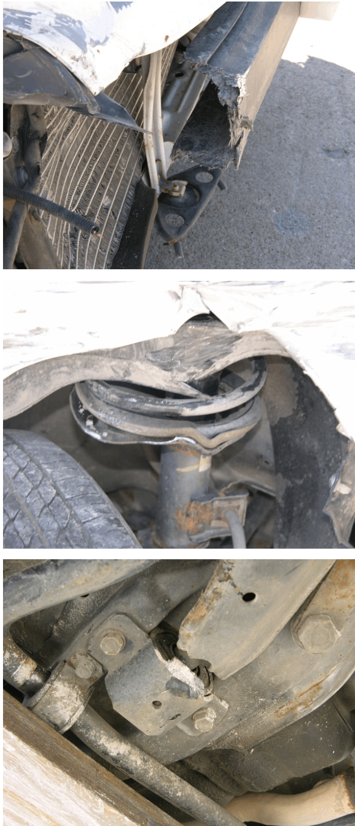
Figure 94. Vehicle Damage, Test FR-3
