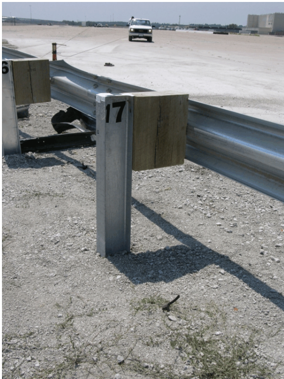
Figure 139. Post Nos. 17 and 18 Damage, Test FR-5
