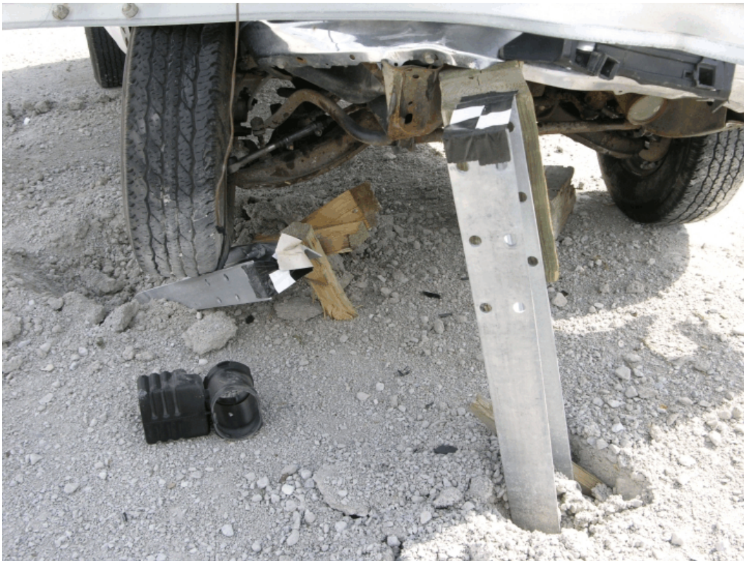
Figure 117. Post Nos. 19 and 20 Damage, Test FR-4
