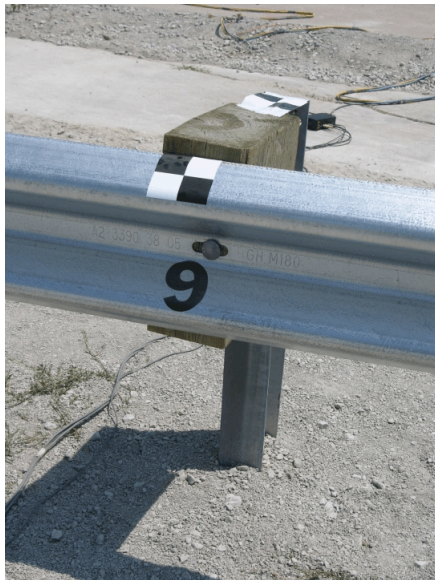
Figure 135. Post Nos. 9 and 10 Damage, Test FR-5
