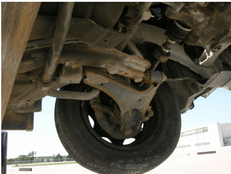
Figure 95. Suspension Damage, Test FR-3
