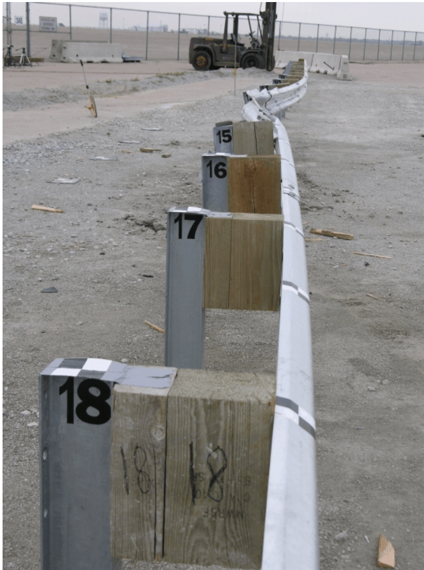
Figure 83. System Damage, Test FR-3
