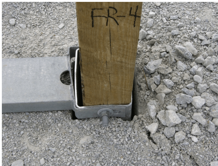
Figure 118. Upstream Anchorage Damage, Test FR-4
