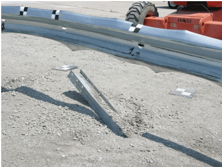
Figure 137. Post Nos. 13 and 14 Damage, Test FR-5
