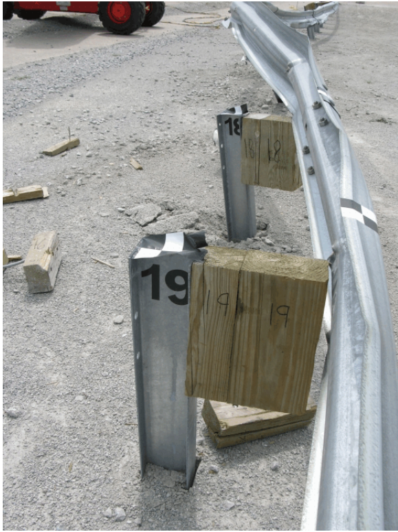
Figure 69. Post Nos. 18 and 19 Damage, Test FR-2
