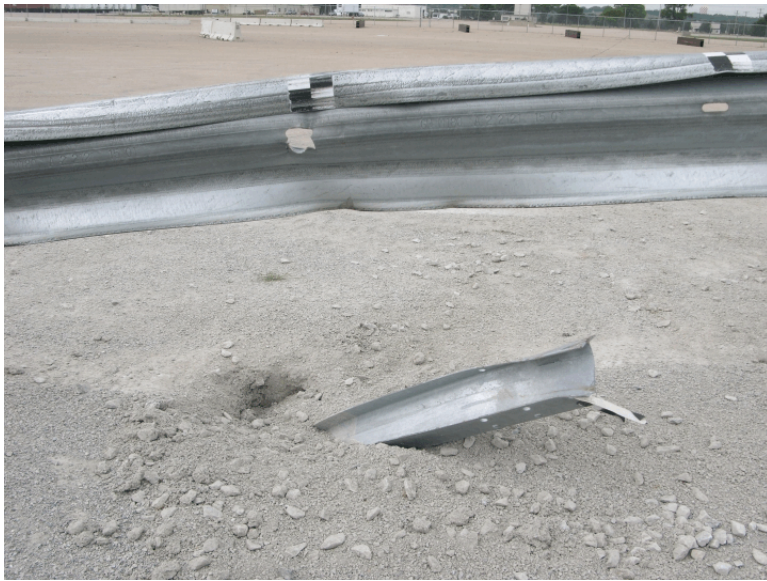
Figure 67. Post Nos. 15 and 16 Damage, Test FR-2
