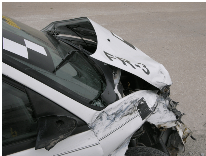
Figure 93. Vehicle Damage, Test FR-3
