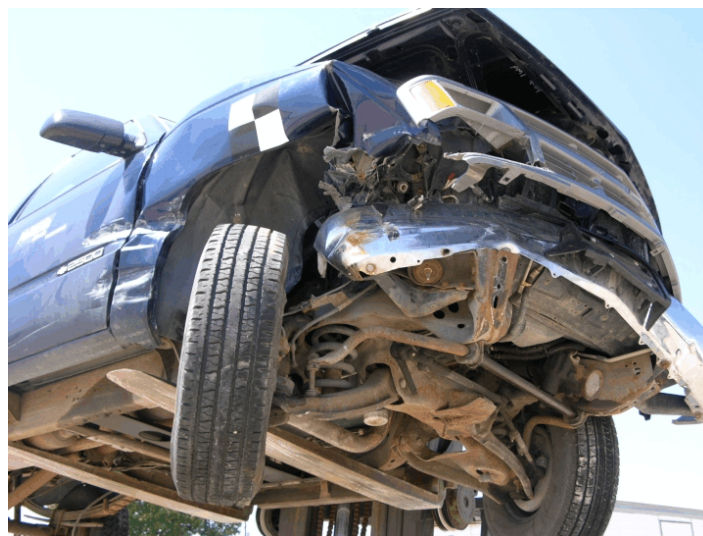
Figure 72. Vehicle Damage, Test FR-2
