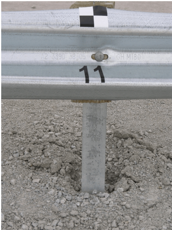
Figure 113. Post Nos. 11 and 12 Damage, Test FR-4
