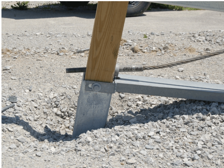
Figure 119. Downstream Anchorage Damage, Test FR-4
