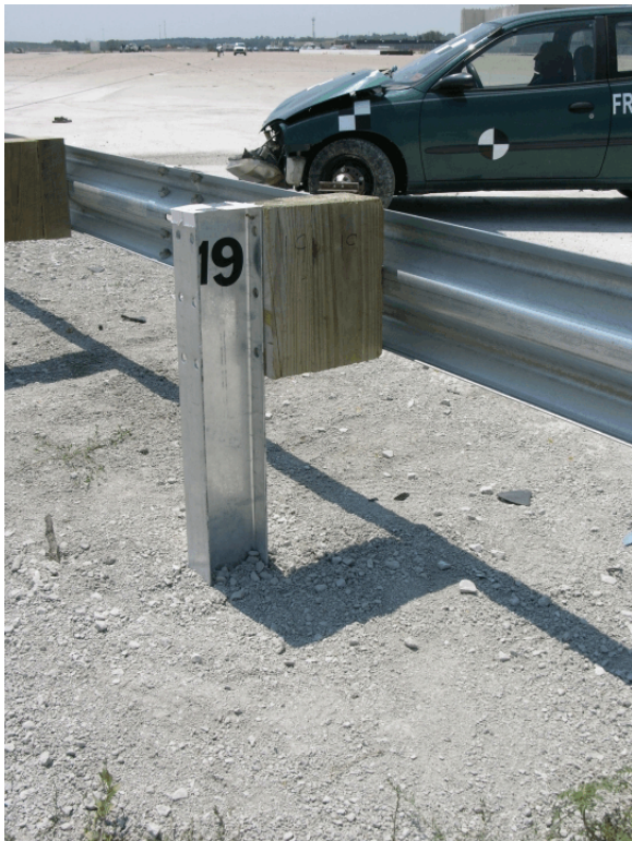
Figure 140. Post Nos. 19 and 20 Damage, Test FR-5
