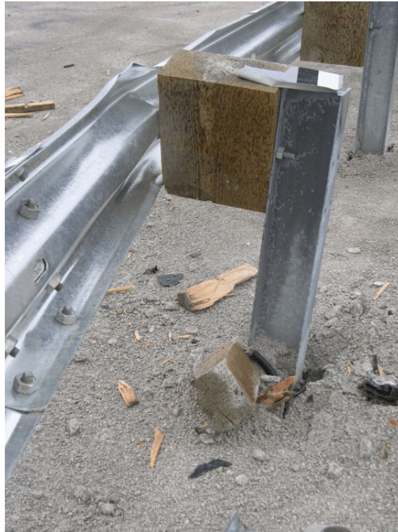
Figure 87. Post No. 15 Damage, Test FR-3
