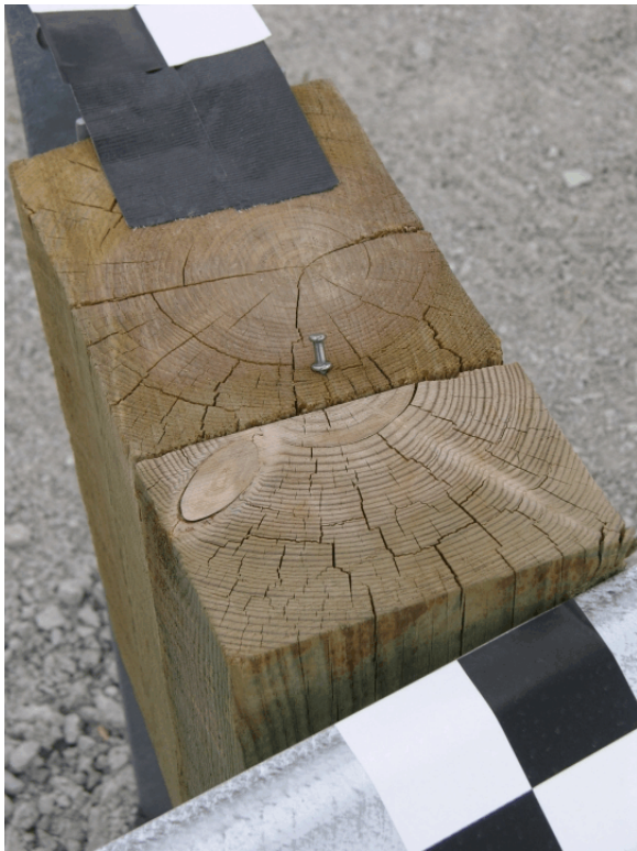
Figure 112. Post Nos. 9 and 10 Damage, Test FR-4
