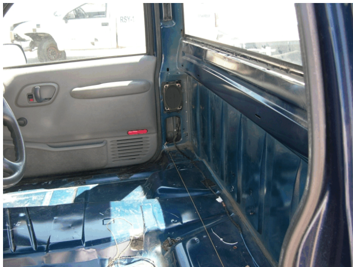
Figure 74. Occupant Compartment Deformation, Test FR-2
