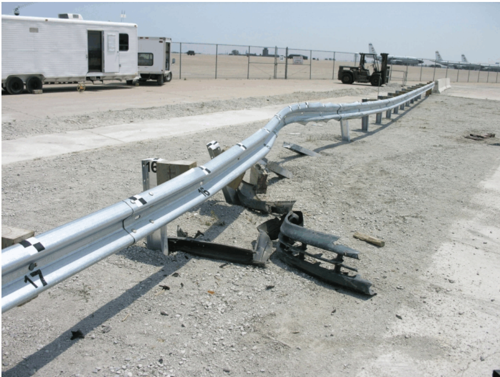
Figure 132. System Damage, Test FR-5
