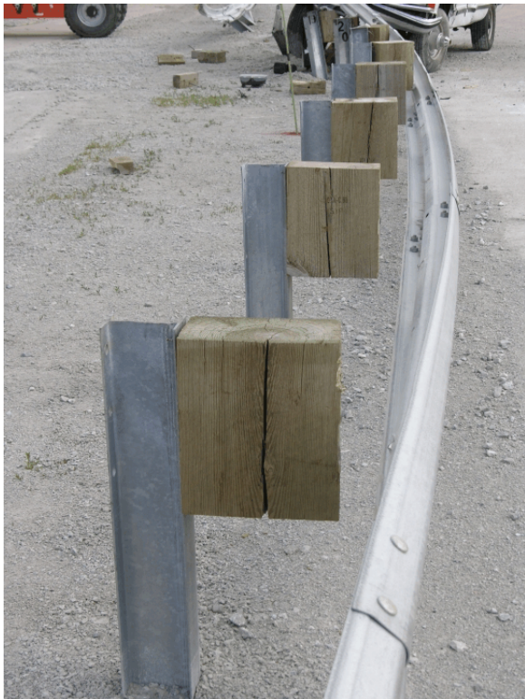
Figure 109. System Damage, Test FR-4
