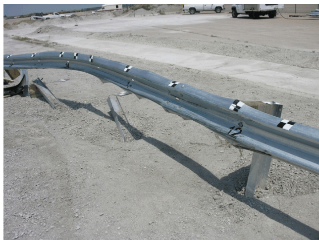
Figure 133. System Damage, Test FR-5
