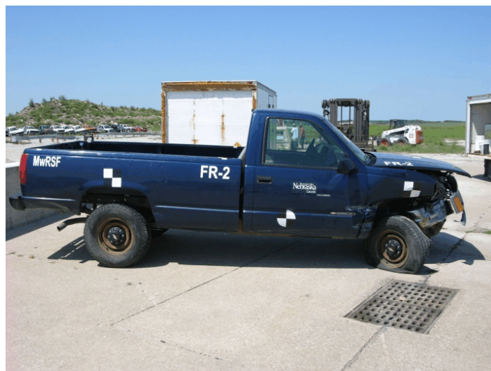
Figure 71. Vehicle Damage, Test FR-2
