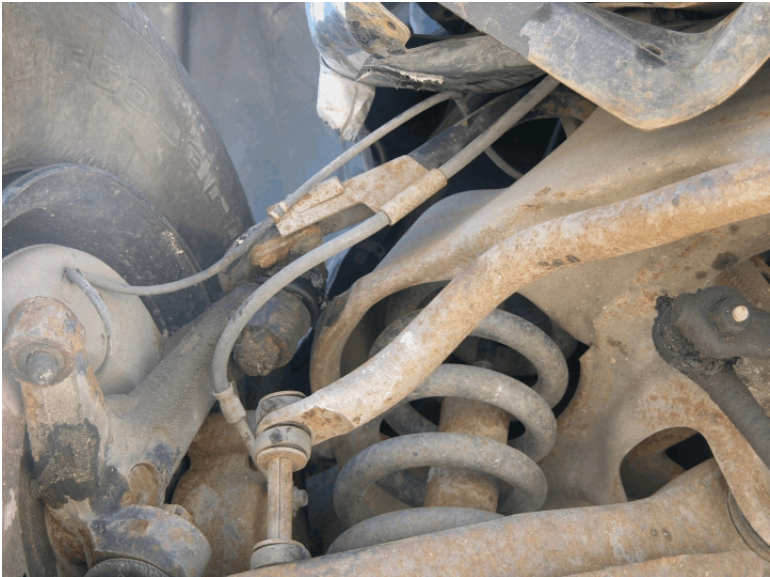
Figure 73. Undercarriage Damage, Test FR-2
