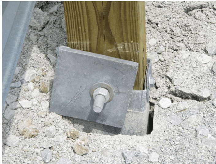
Figure 70. Anchorage Damage, Test FR-2
