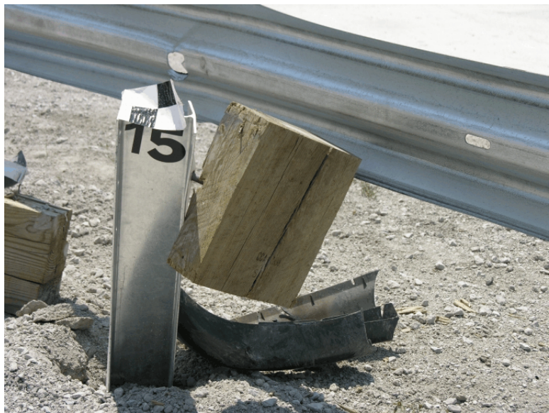
Figure 138. Post Nos. 15 and 16 Damage, Test FR-5
