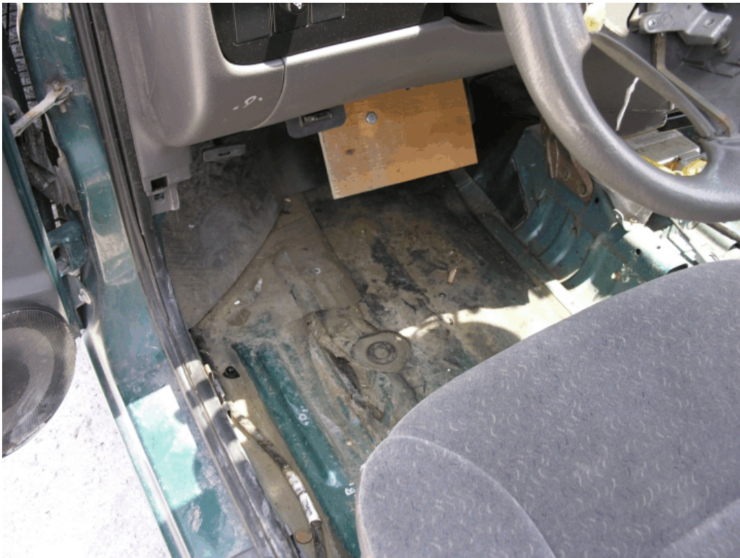
Figure 145. Occupant Compartment Deformation, Test FR-5
