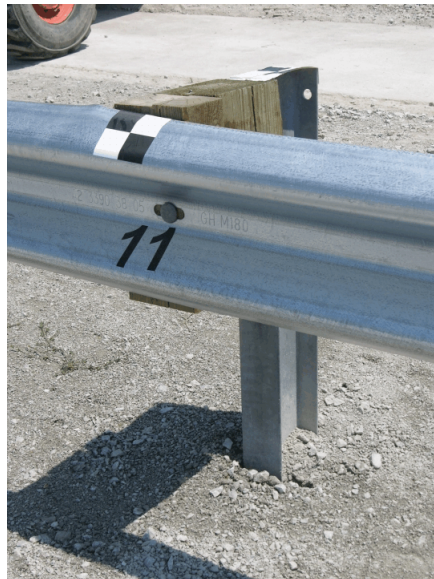
Figure 136. Post Nos. 11 and 12 Damage, Test FR-5
