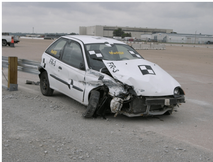
Figure 91. Vehicle Damage, Test FR-3
