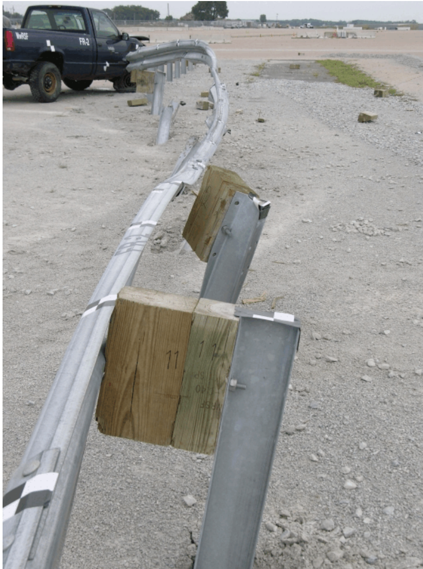
Figure 62. System Damage, Test FR-2
