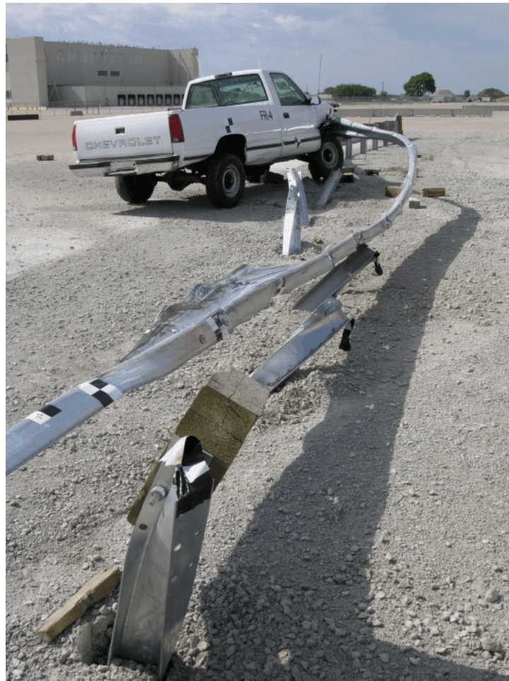
Figure 111. System Damage, Test FR-4
