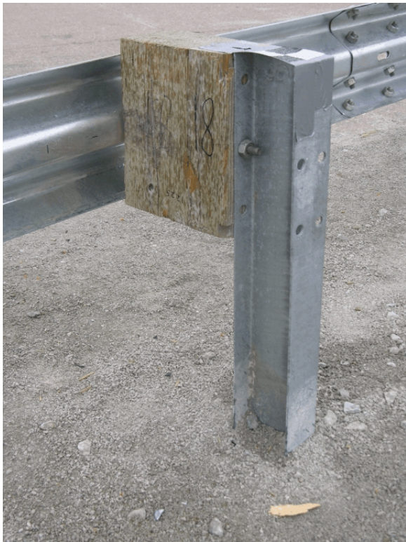
Figure 89. Post Nos. 18 and 19 Damage, Test FR-3
