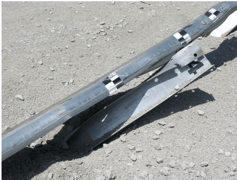
Figure 42. Post Nos. 13 and 14 Damage, Test No. FR-1
