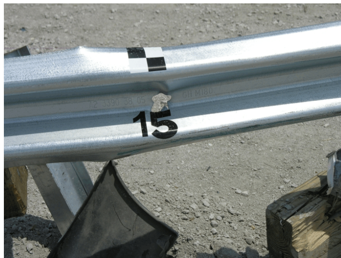
Figure 134. Rail Damage, Test FR-5
