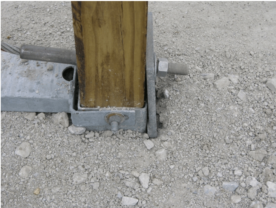
Figure 90. Downstream Anchorage Damage, Test FR-3
