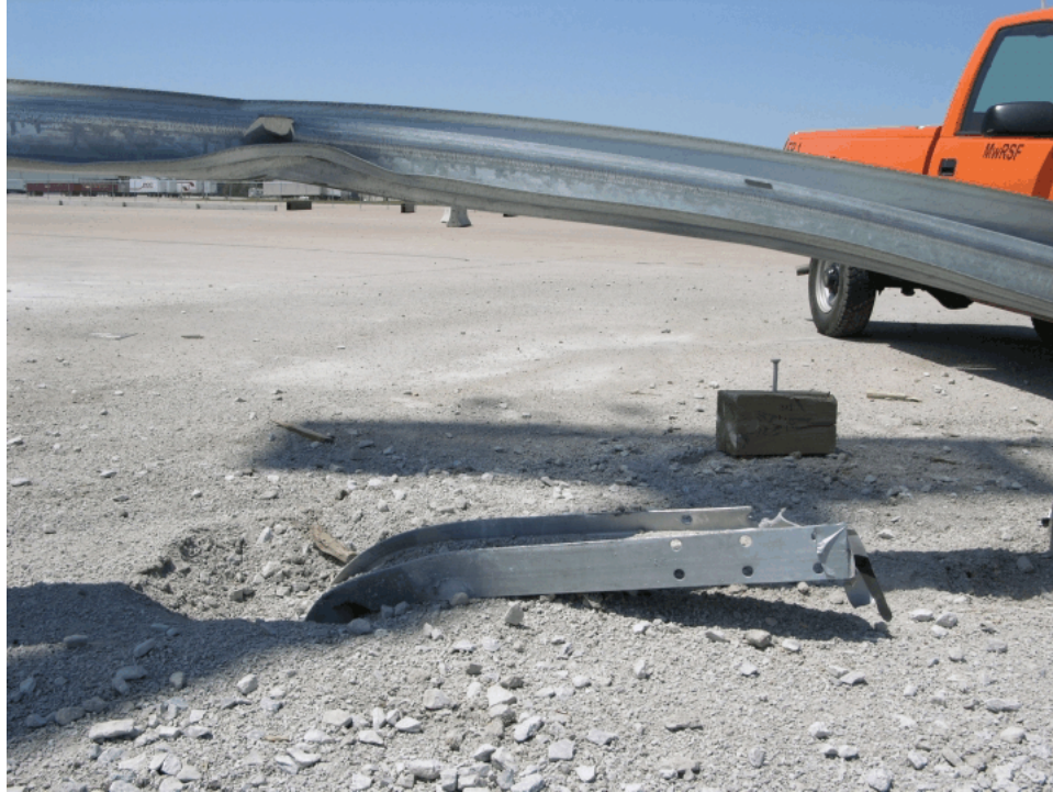
Figure 44. Post Nos. 17 and 18 Damage, Test FR-1
