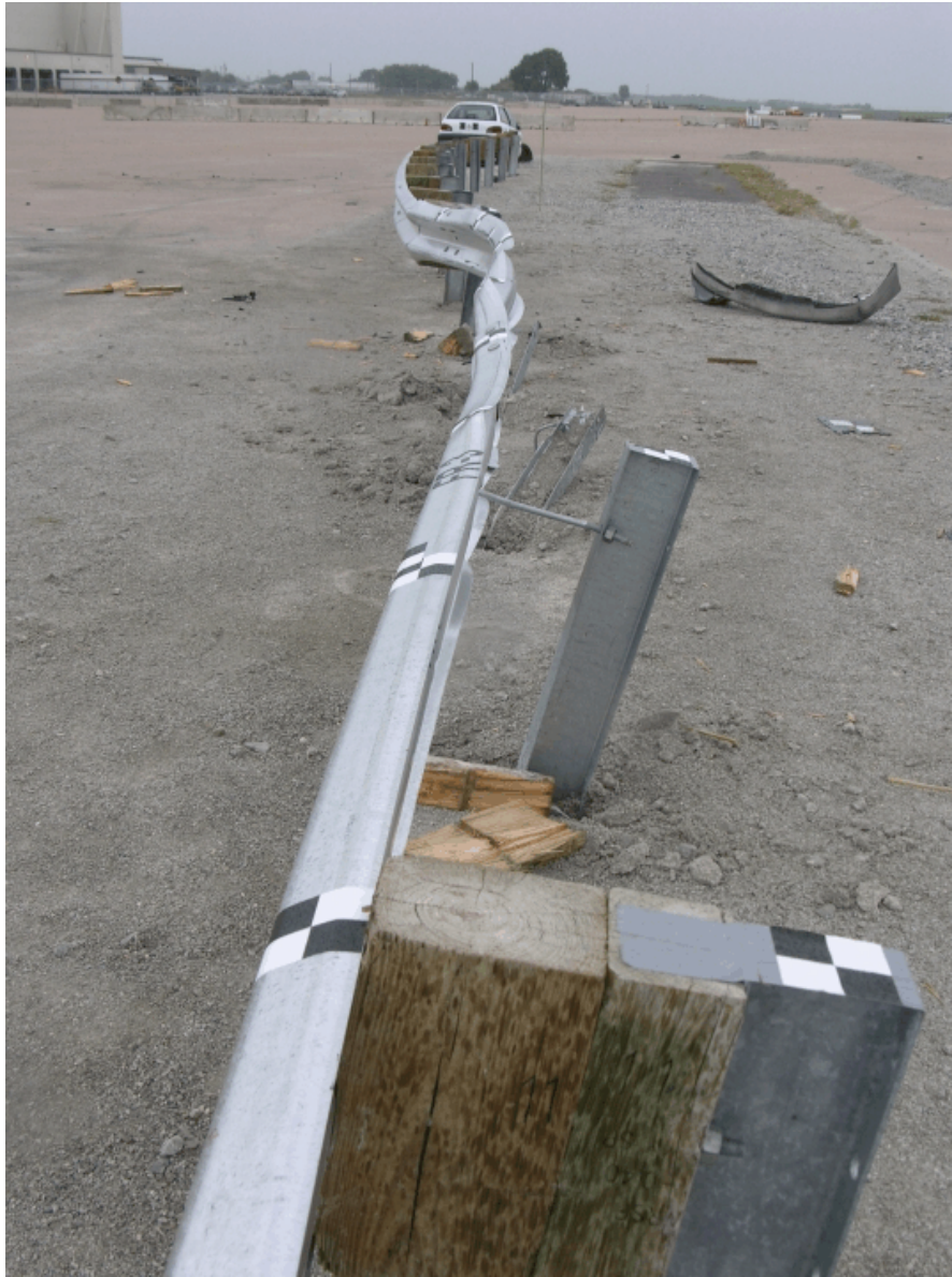
Figure 82. Vehicle Trajectory and Final Position, Test FR-3
