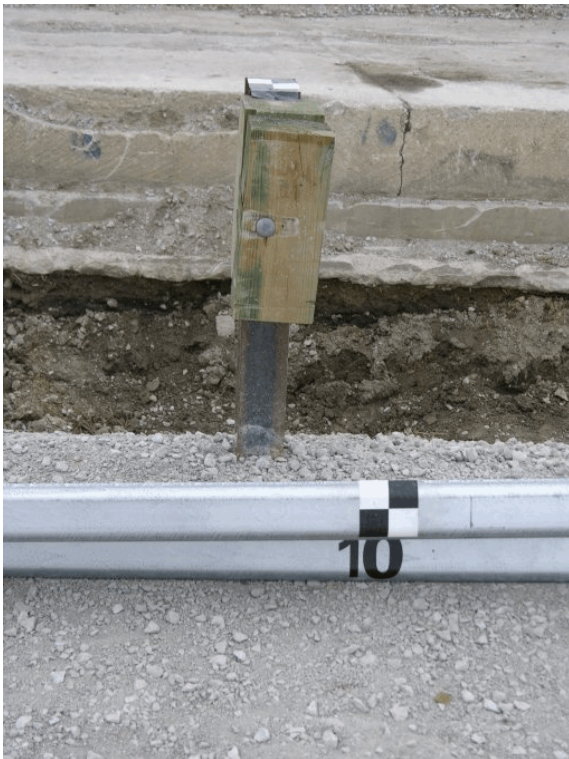
Figure 60. Post Nos. 9 through 12 Damage, Test No. MGS221-2
