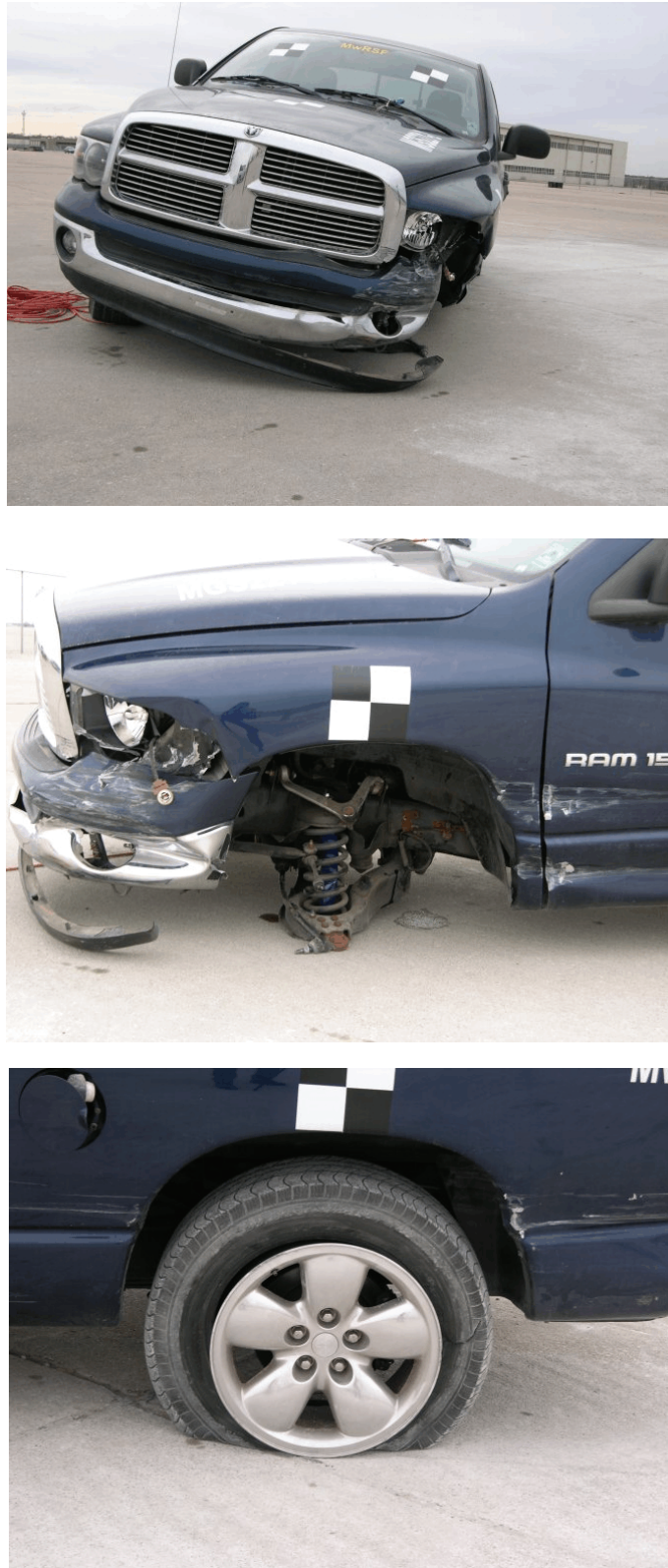
Figure 66. Vehicle Damage, Test No. MGS221-2
