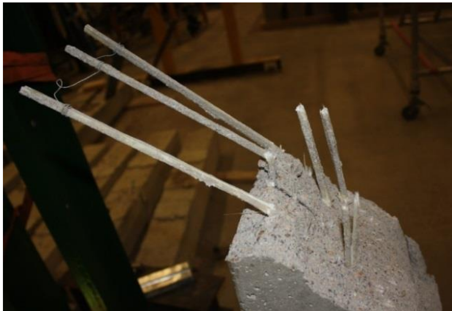
Figure 4.17 Debonding failure of Ib-2
