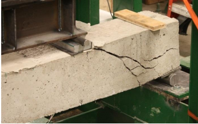
Figure 4.21 I Ib-2 failure patterns before collapse
