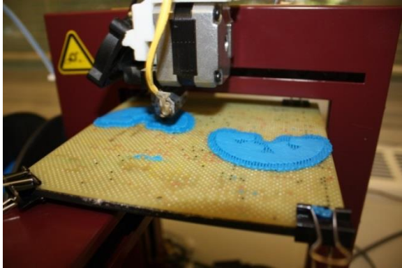
Figure 3.12 3D printing in progress of type II form molds
