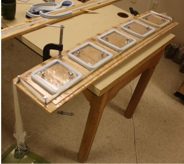
Figure 3.31 GFRP lay-up of stirrups
