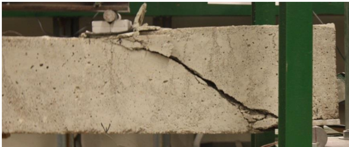
Figure 4.14 Ib-1 shear crack (rear view)
