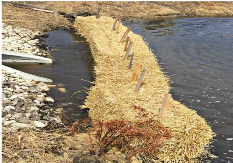
Figure 4.14 Unfiltered sediment passing through product.
