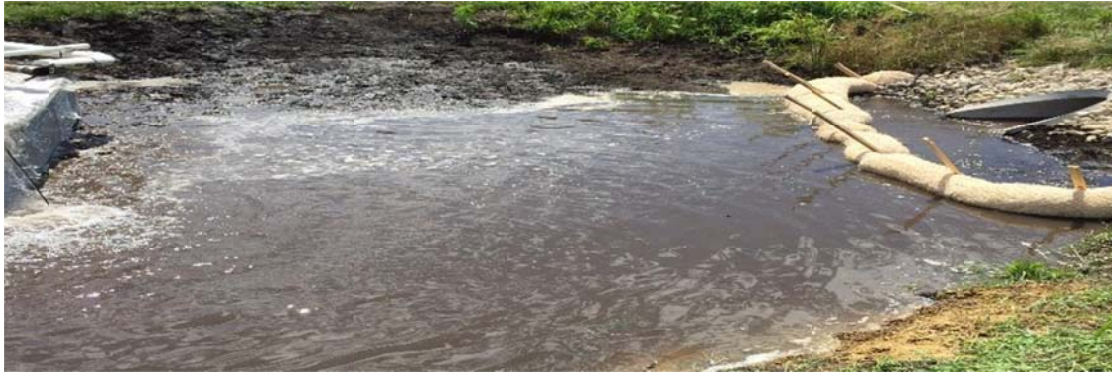
Figure 4.1 Sediment log at 158 gpm (10 L/s) flow rate.
