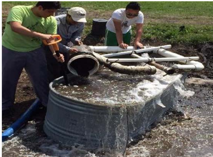
Figure 3.9 Adding clay soil.
