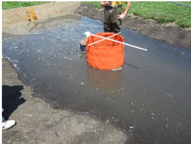
Figure 4.2 Channel ponding during the welded-wire woven monofilament lid test at 79 gpm (5 L/s).
