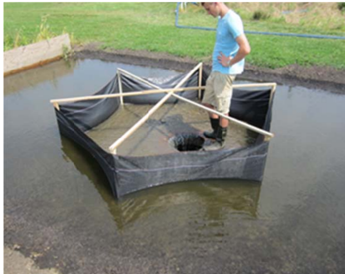
Figure 4.15 Silt fence at 79 gpm (5 L/s) flow rate, inside.
