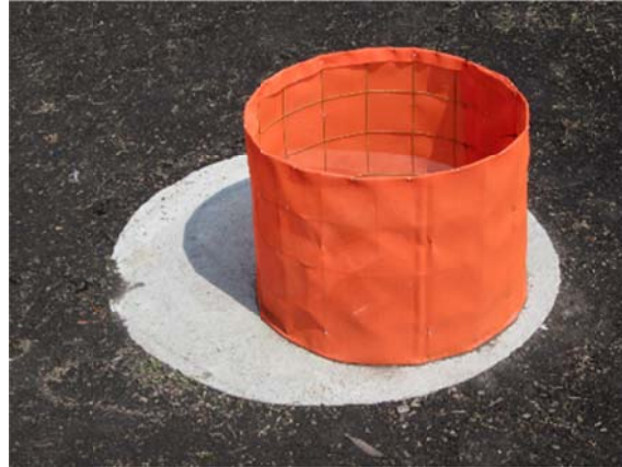
Figure 3.1 Welded-wire woven monofilament around the lid.
