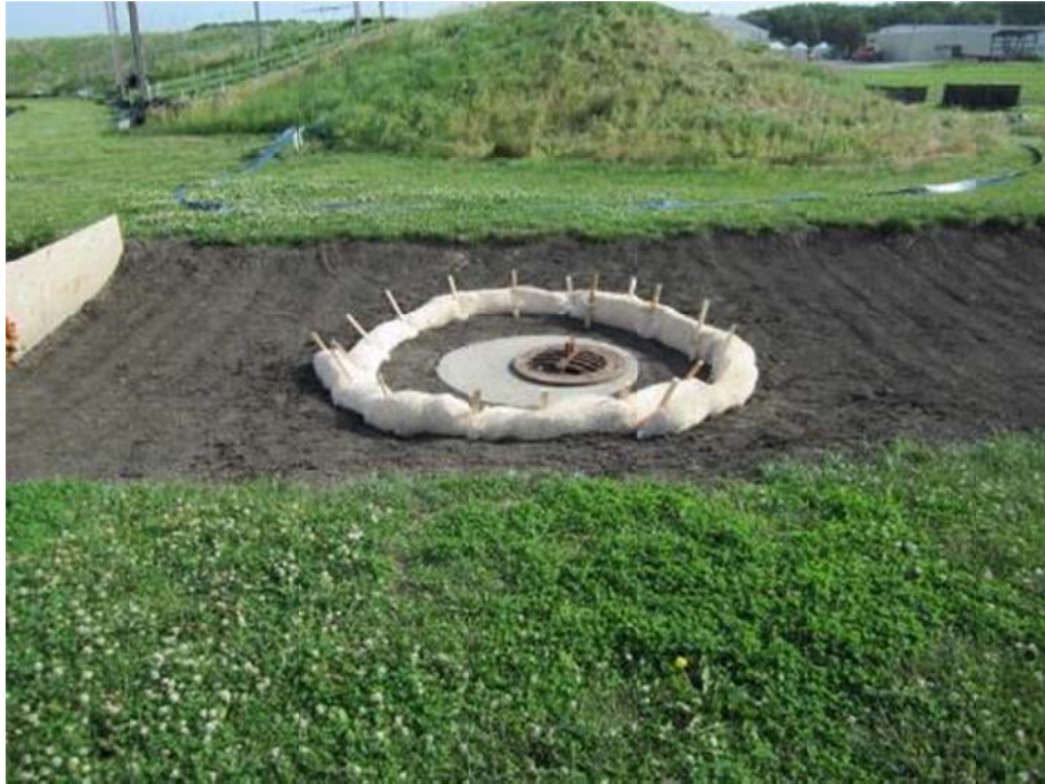
Figure A.5 Sediment log, pre-testing.
