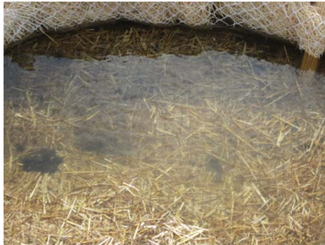
Figure 4.7 Sediment log with erosion control blanket, at 79 gpm (5 L/s) flow rate and showing sediment settling on the blanket.
