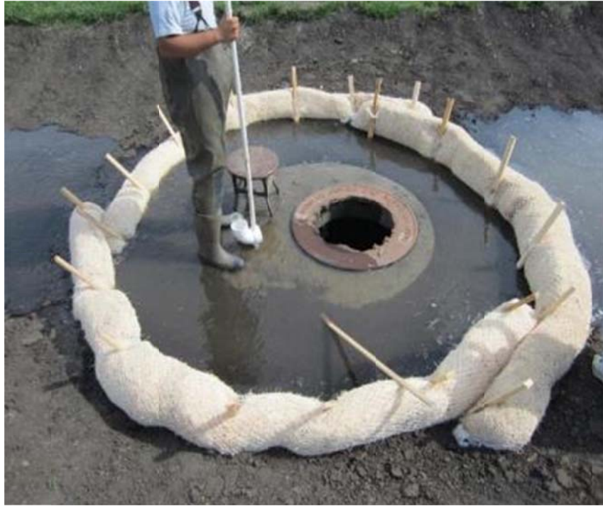
Figure A.7 Sediment log during testing.
