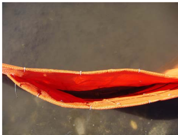
Figure 4.4 Welded-wire woven monofilament with 2 foot gap under 79 gpm (5 L/s) flow rate, with overlap failure.
