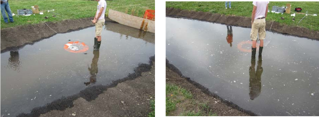
Figure 4.11 Dandy Bag at 79 gpm (5 L/s) flow rate.
