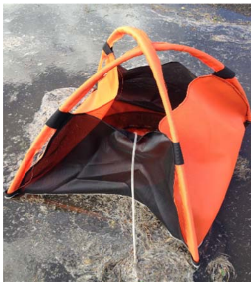
Figure 4.10 Dandy Pop at 79 gpm (5 L/s) flow rate, inside.
