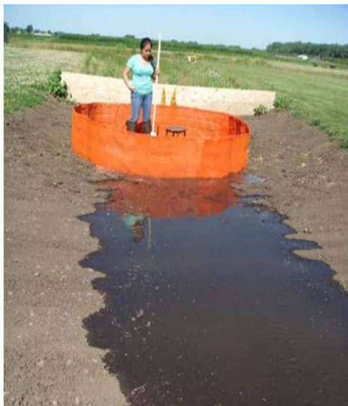
Figure A.2 Welded-wire woven monofilament fabric after testing started.
