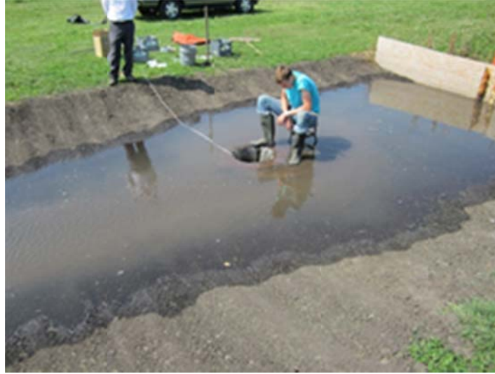
Figure 4.14 Filter bag at 158 gpm (10 L/s) flow rate.
