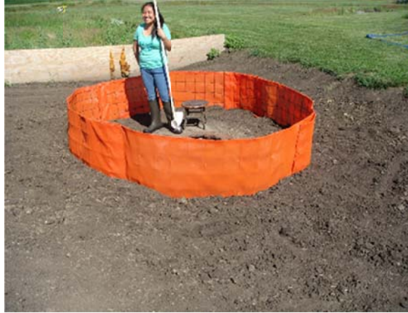
Figure 3.2 Welded-wire woven monofilament with 2 foot gap.
