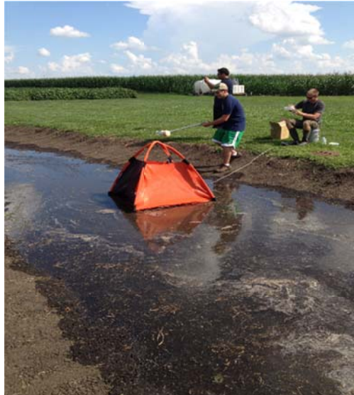
Figure 4.9 Dandy Pop testing at 79 gpm (5 L/s) flow rate.
