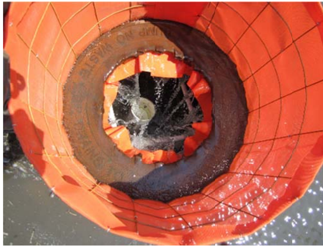
Figure 4.1 Inside of the welded-wire woven monofilament at 79 gpm (5 L/s).
