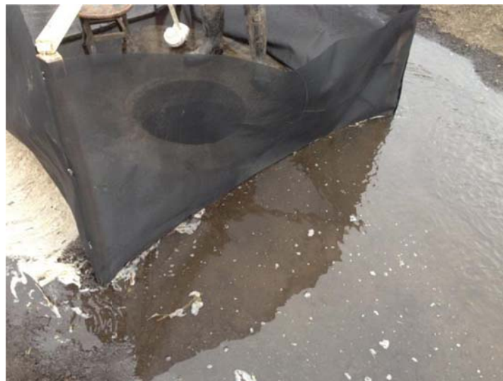
Figure 4.20 Front of the silt fence (monofilament fabric) during testing.
