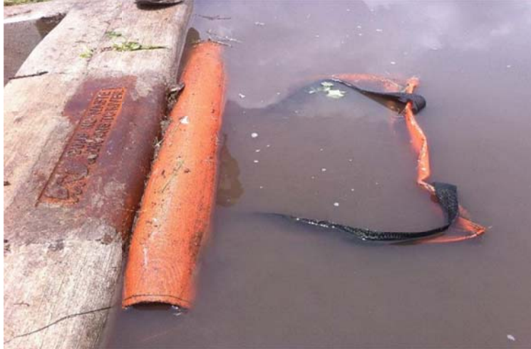
Figure 4.7 Dandy curb bag at 119 gpm (7.5 L/s) flow rate.
