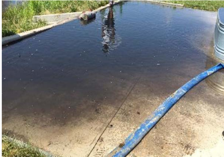
Figure 4.10 GeoHay at 119 gpm (7.5 L/s).
