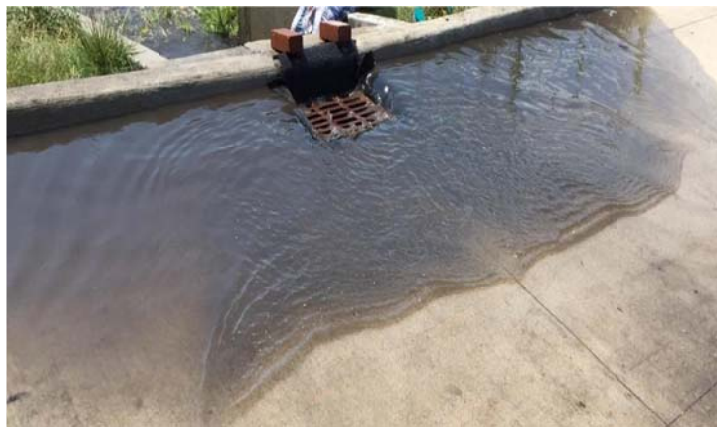
Figure 4.18 Inlet Pro at 119 gpm (7.5 L/s) flow rate.
