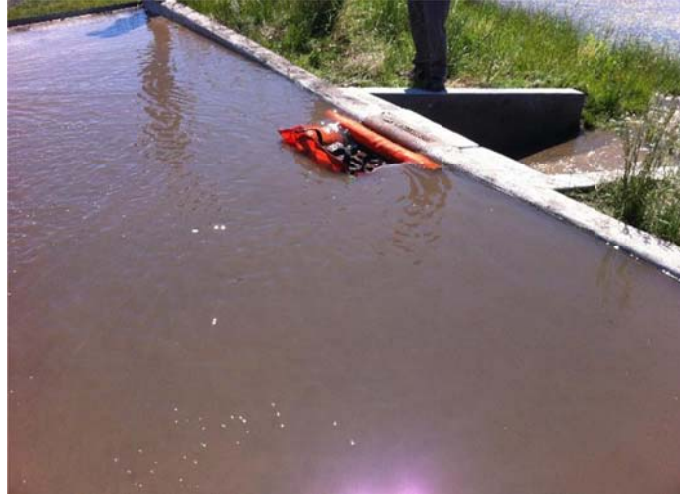
Figure 4.5 Dandy curb sack at 119 gpm (7.5 L/s) flow rate.
