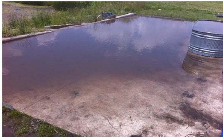
Figure 4.8 Dandy curb bag at 119 gpm (7.5 L/s) flow rate, concrete slab.
