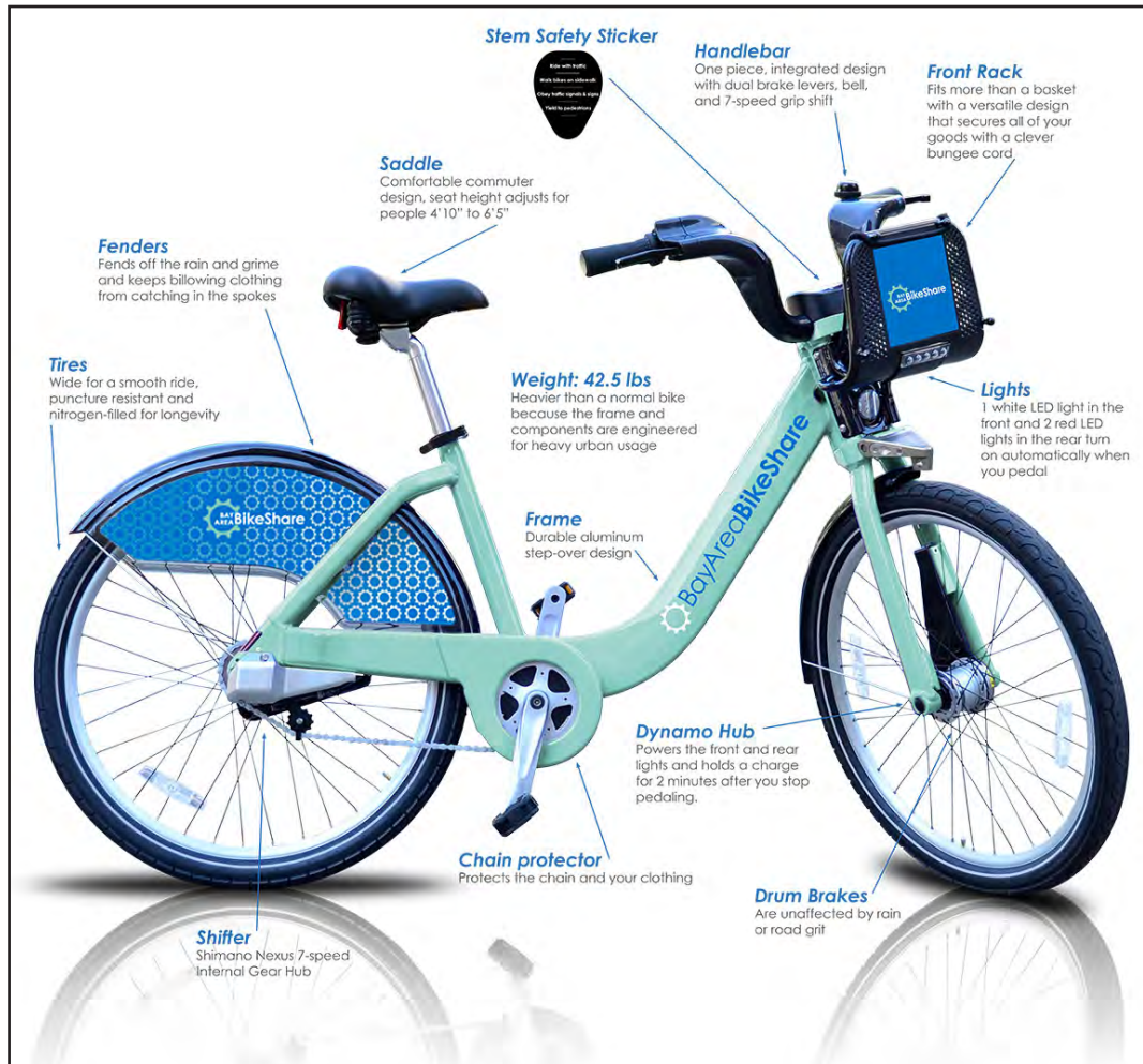
Figure 1. Common Safety Features of Public Bikesharing Bicycles
