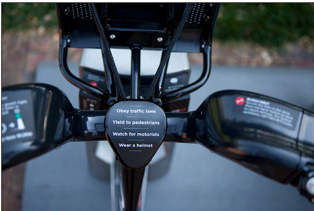
Figure 2. Handlebar Safety Reminders
