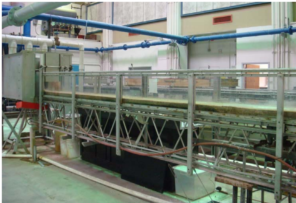
Figure 4.1. Flume apparatus for the erosion test: system layout (upper) and photo (lower).
