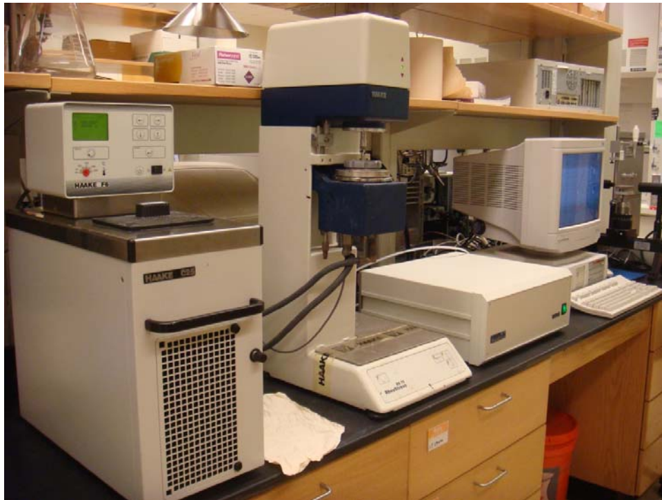
Figure 4.2. Stress-controlled rheometer apparatus: system layout (upper) and photo (lower).
