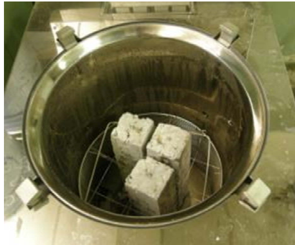
Figure 19. ACPT specimens in autoclave.
