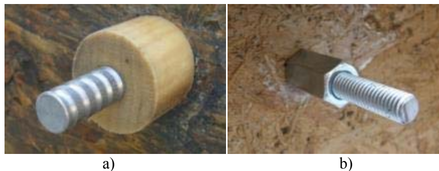
Figure 71. Insert assembly on a) the inside of the form and b) the outside of the form.
