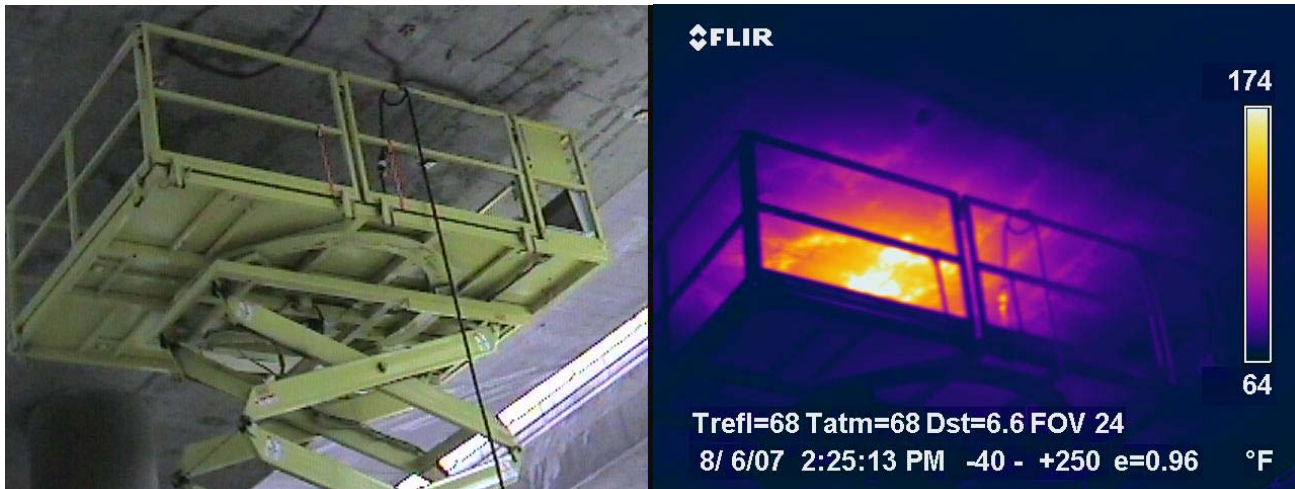
Figure 19 – Typical orientation of lift truck and heater to heated surface (Method 2)
