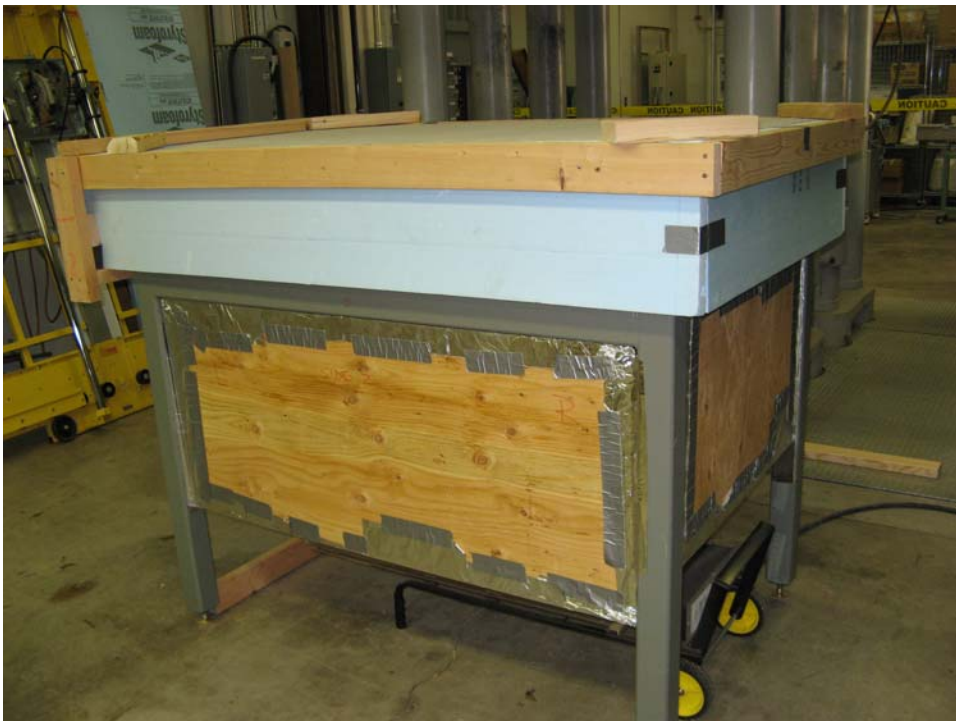
Figure 8 – Test set-up showing aluminum-covered plywood sides and insulation on edges/ends of a concrete specimen
