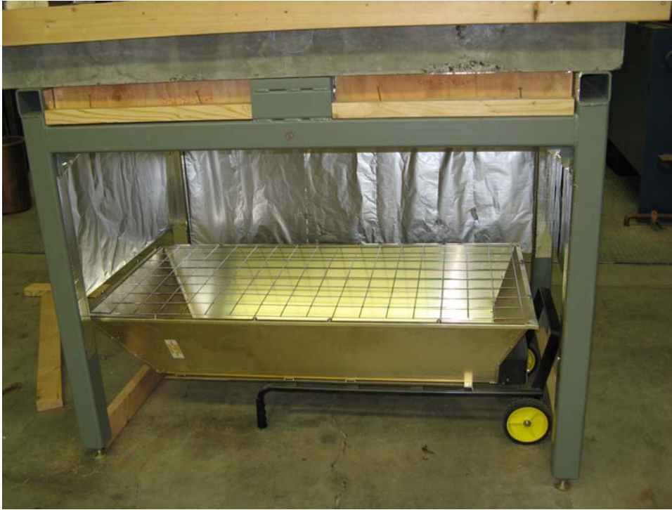
Figure 7 – Test set-up showing infrared heater and test frame supporting a concrete specimen
