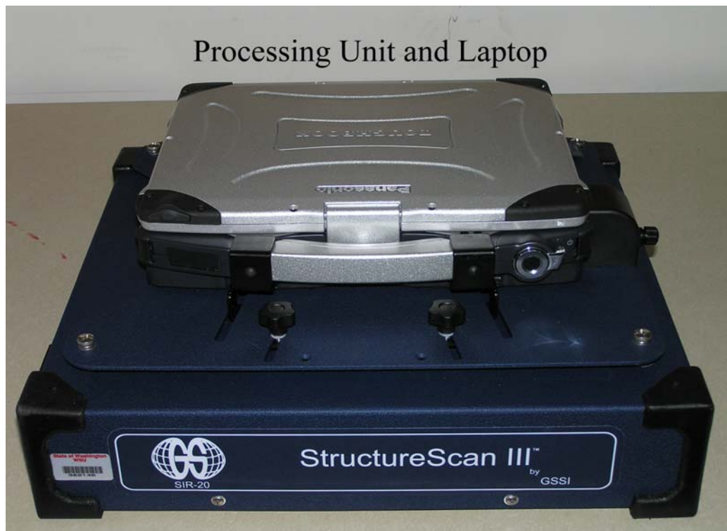
Figure 12 – StructureScan processing unit and laptop computer.
