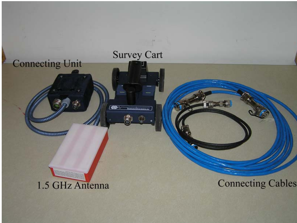
Figure 11 – GPR antenna, survey cart, connecting unit, and cables.
