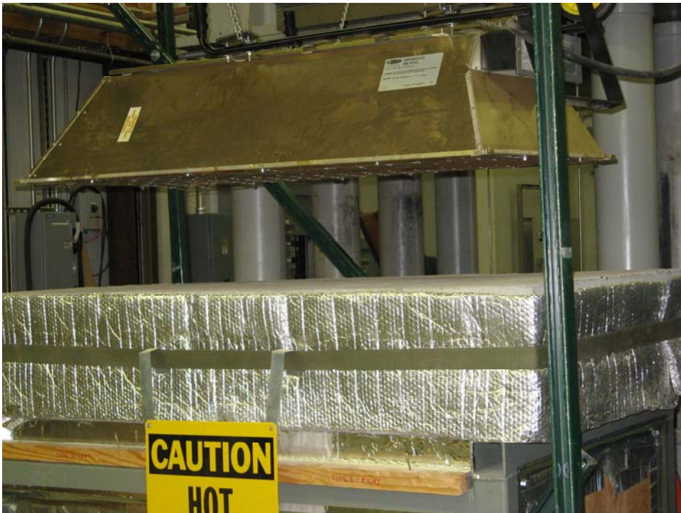
Figure 9 – Test set-up with heater suspended above a concrete specimen
