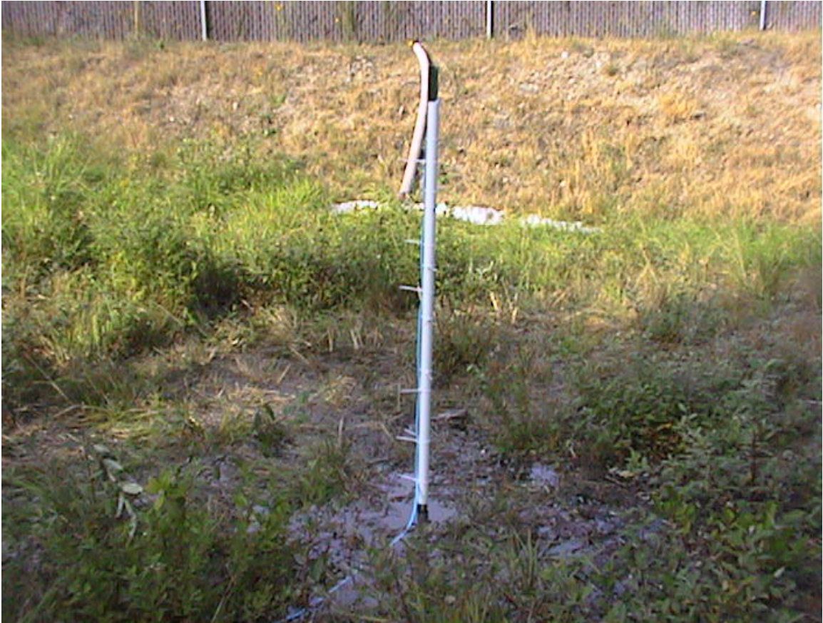
Figure 4.1 - Pressure transducer installed at Krista Firs, Kitsap County.
