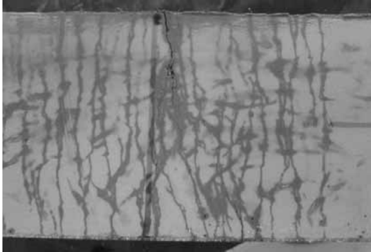
Figure 2.27. Micro-cracking during a flexural prism test (Acker and Behloul 2004)
