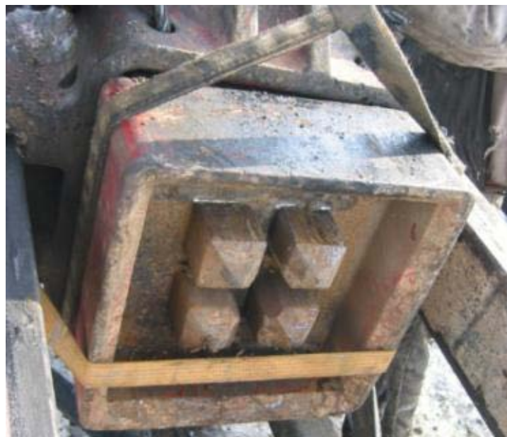
Figure 5.5. Driving helmet with guiding spikes used for steel piles
