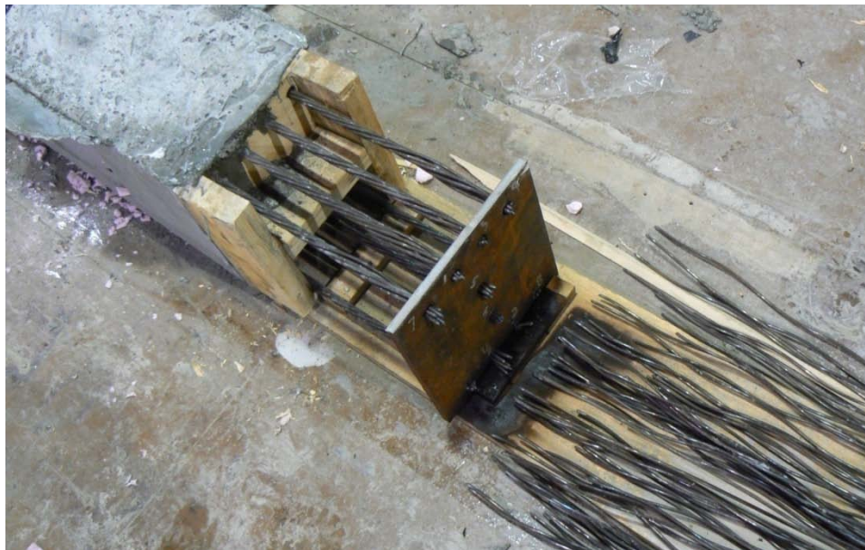
Figure 4.15. Strands released at end of UHPC pile P2
