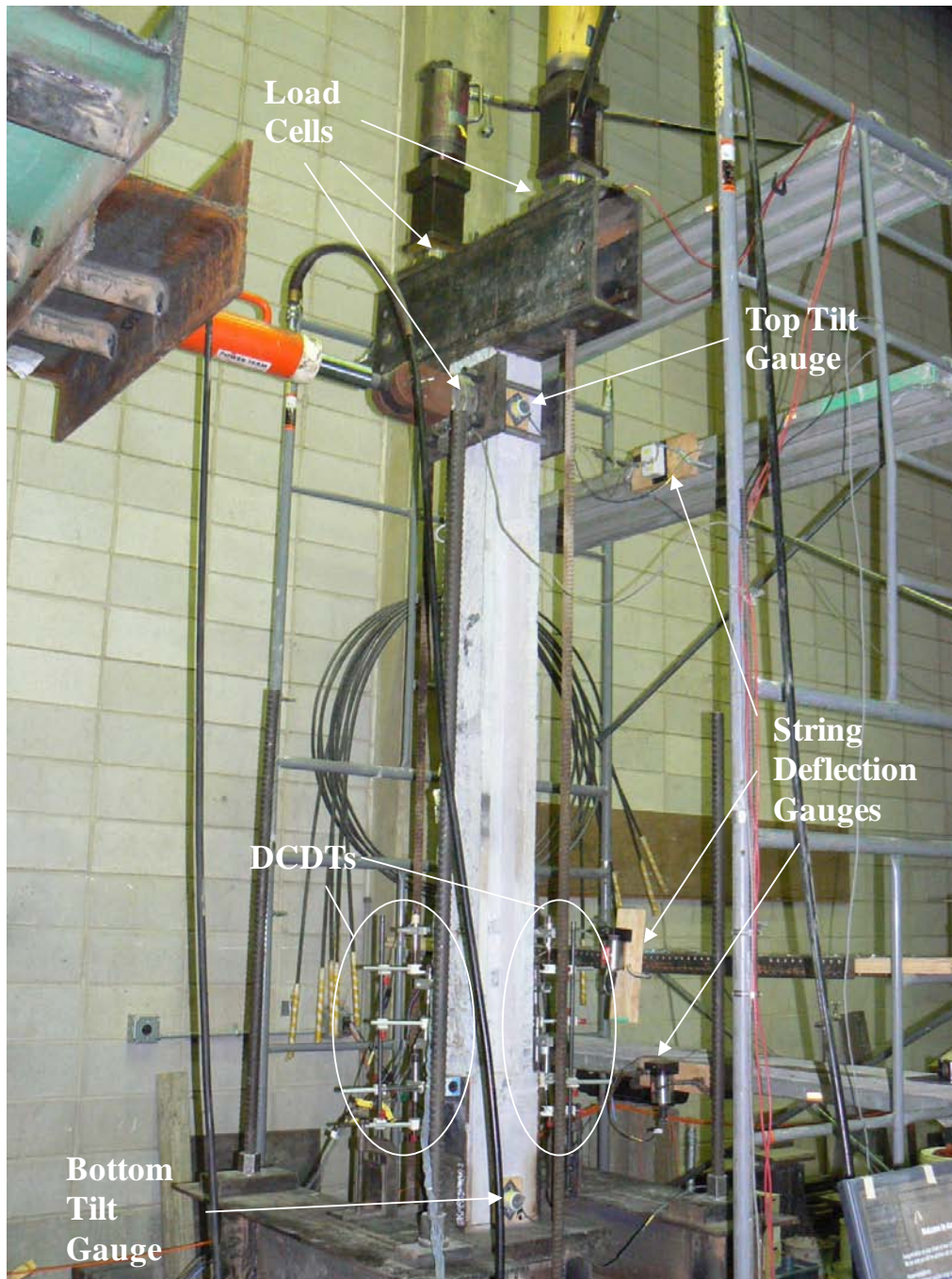
Figure 4.29. Test setup of UHPC test unit L1 and the location of external instruments
