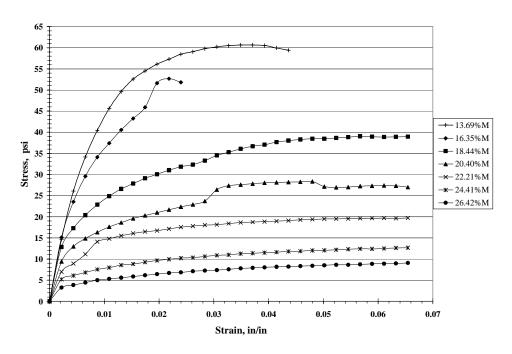
Figure B.2. Stress-strain response of Argyle paleosol at various moisture contents
