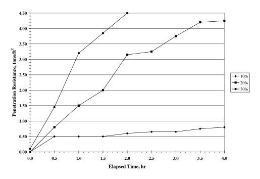
Figure 55. Strength gain of Turin loess dried with PN4 fly ash
