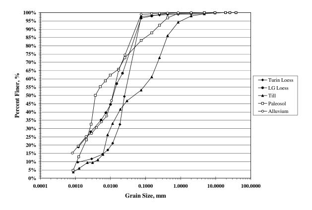
Figure 2. Soil particle size distribution
