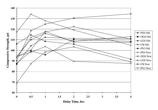
Figure 30. Influence of compaction delay on strength gain of Class C fly ash and Turin loess
