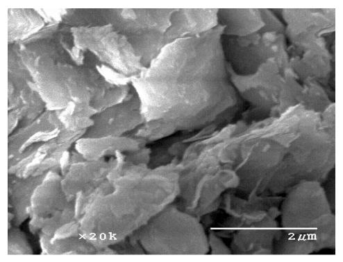
Figure 5. SEM image at 20,000x of Glacial Till clay fraction (<2 microns)
