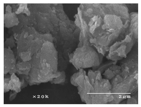
Figure 3. SEM image at 20,000x of Le Grand Loess clay fraction (<2 microns)
