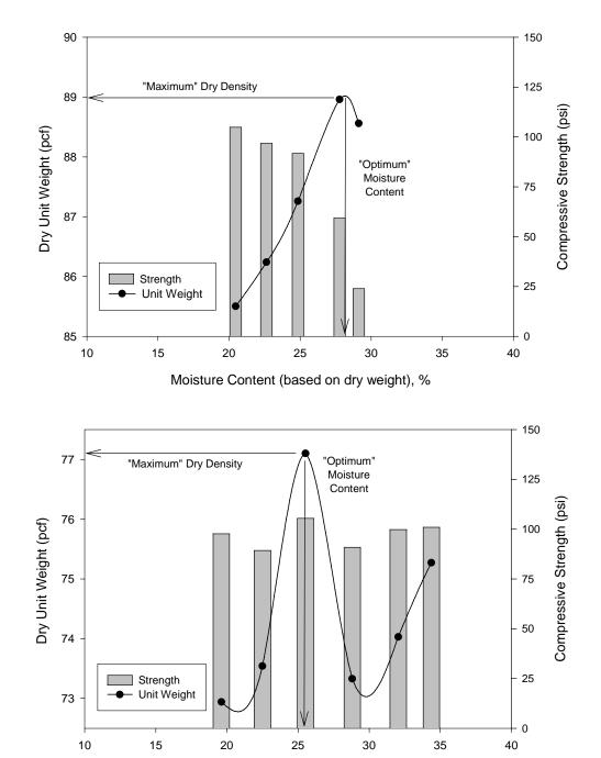
Figure E.1. Typical moisture-density and moisture-strength relationships for CFA materials
