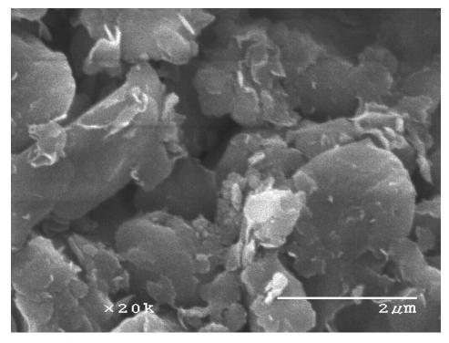
Figure 4. SEM image at 20,000x of Alluvium clay fraction (<2 microns)
