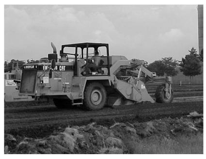
Figure 1. Pulvamixer used for on-site mixing
