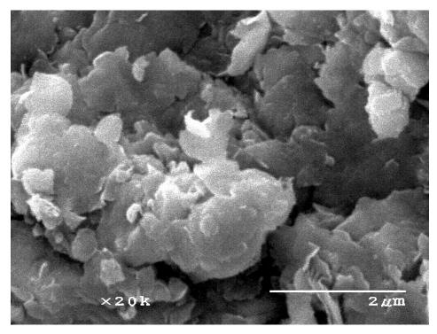
Figure 6. SEM image at 20,000x of Paleosol clay fraction (<2 microns)
