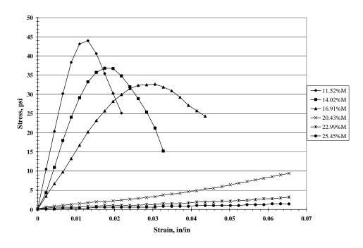
Figure B.4. Stress-strain response of Turin loess at various moisture contents
