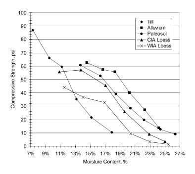
Figure 14. Moisture-strength relationships of soils used in the study
