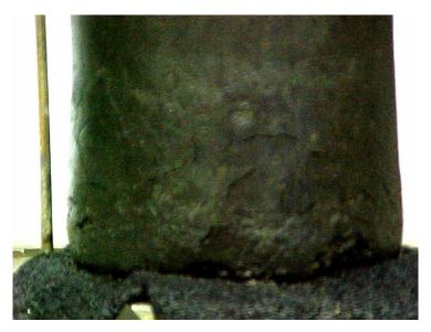
Figure 72. SGS CFA after one freeze-thaw cycle
