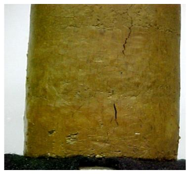
Figure 73. Le Grand loess after one freeze-thaw cycle
