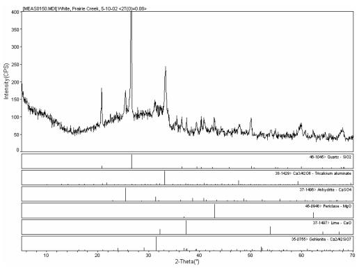
Figure A.12. X-Ray diffractogram for PC3+4 fly ash
