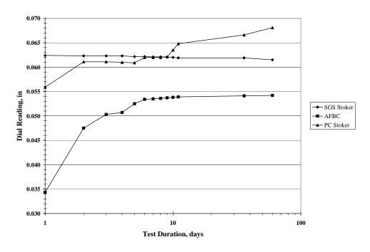
Figure 56. Swell of paleosol-high sulfur fly ash mixtures
