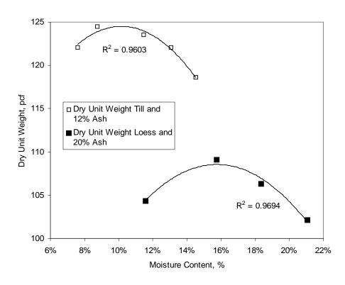
Figure C.1. Typical moisture-density relationships of stabilized soil
