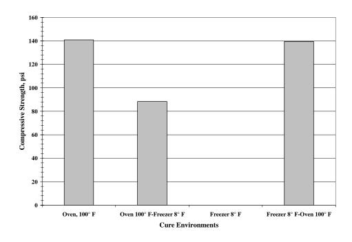
Figure 65. Influence of cure environment on strength gain of self-cementing fly ash-soil mixtures
