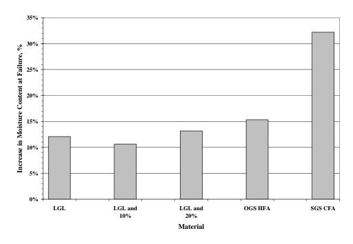
Figure 76. Moisture content increase of ASTM D560 volumetric stability samples
