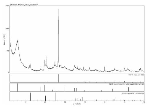
Figure A.3. X-Ray diffractogram for Argyle paleosol clay fraction (<2 microns)
