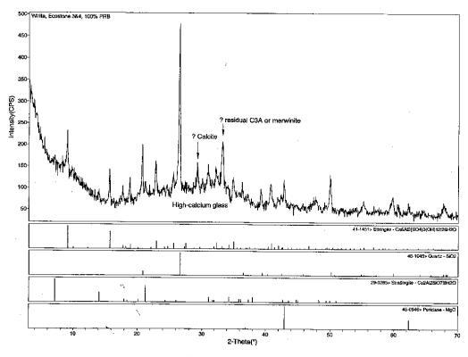
Figure A.18. X-Ray diffractogram for PC conditioned fly ash
