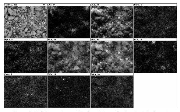
Figure 7. EDS elemental map of Le Grand Loess clay fraction (<2 microns)
