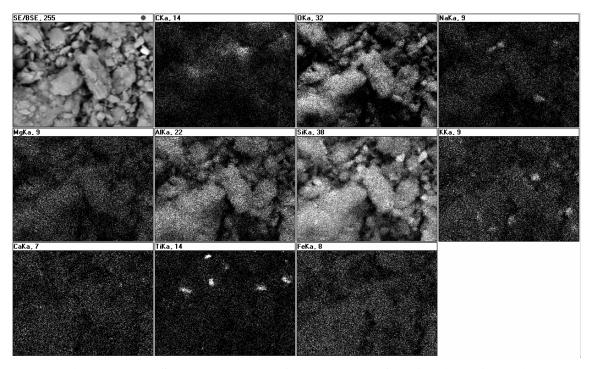
Figure 10. EDS elemental map of Paleosol clay fraction (<2 microns)
