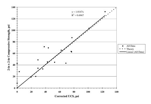
Figure 45. Correlation between two-inch  ${\bf x}$  two-inch compressive strength and corrected UCS
