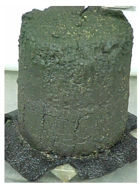
Figure 79. SGS CFA prior to second cycle brushing
