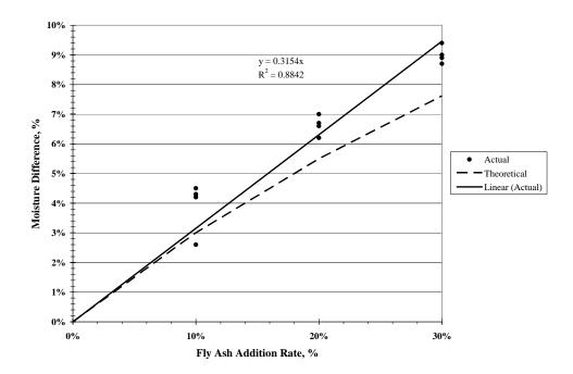
Figure 51. Soil moisture loss as a function of fly ash content
