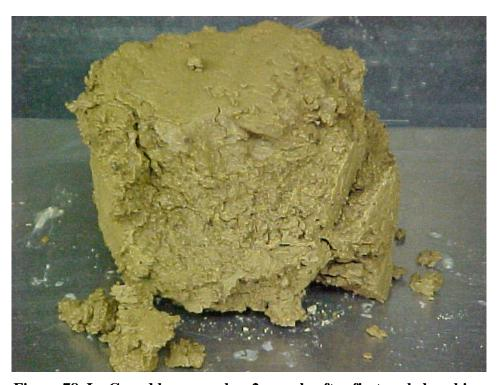
Figure 78. Le Grand loess number 2 sample after first cycle brushing
