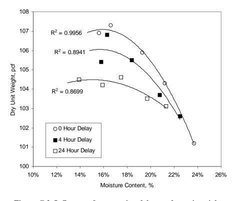
Figure C.2. Influence of compaction delay on dry unit weight
