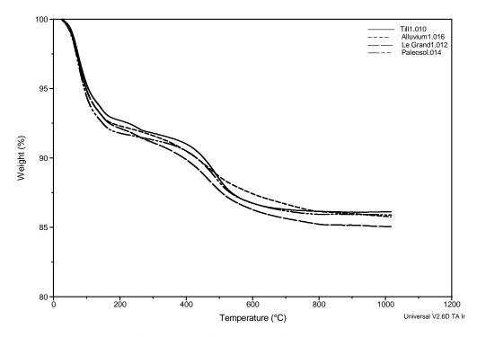
Figure 11. TGA results for soil clay fractions (<2 microns)
