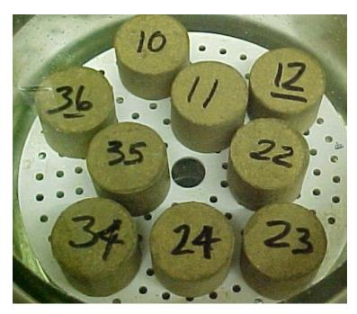
Figure 69. Vacuum saturated paleosol and fly ash after curing at 100° F
