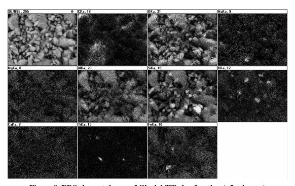
Figure 9. EDS elemental map of Glacial Till clay fraction (<2 microns)
