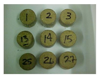
Figure 63. Paleosol and fly ash cured at 70° F after soaking
