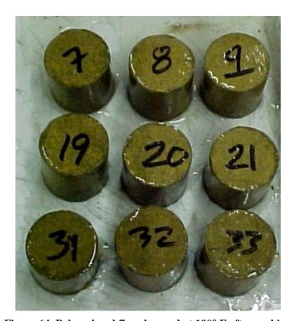
Figure 64. Paleosol and fly ash cured at  $100^{\circ}$  F after soaking
