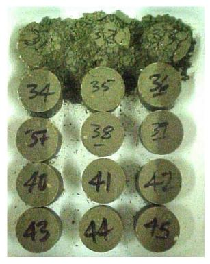
Figure 33. 24-hour compaction delay samples after soaking (molded moisture content increases from top to bottom)
