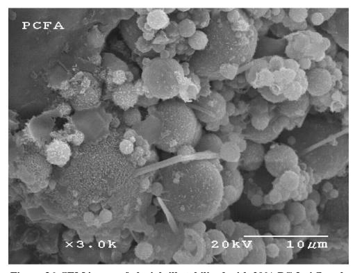
Figure 36. SEM image of glacial till stabilized with 20% PC 3+4 fly ash
