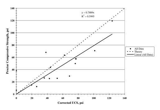
Figure 46. Correlation between Proctor compressive strength and corrected UCS
