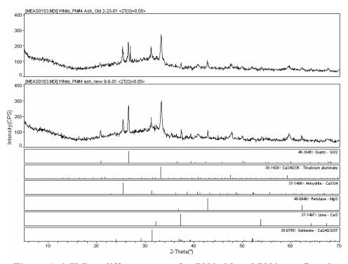
Figure A.6. X-Ray diffractograms for PN4 old and PN4 new fly ash
