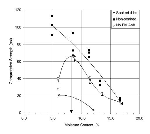
Figure C.3. Typical moisture-strength relationships for soaked and unsoaked fly ash modified subgrade. (For soaked samples, optimum moisture content is approximately 8.2%)
