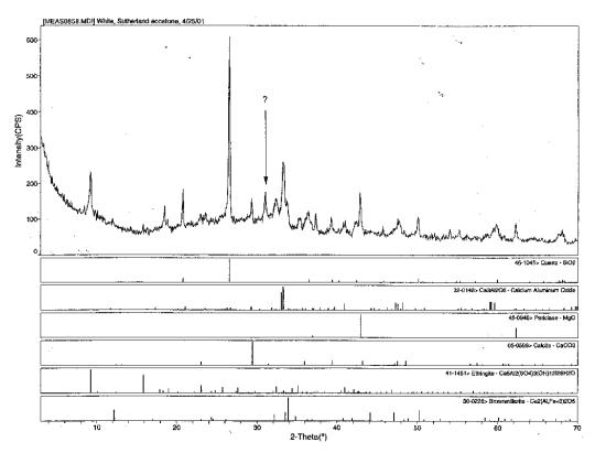
Figure A.19. X-Ray diffractogram for SGS conditioned fly ash
