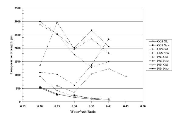
Figure 17. Class C fly ash paste strength
