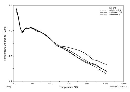
Figure 12. DTA results for soil clay fractions (<2 microns)
