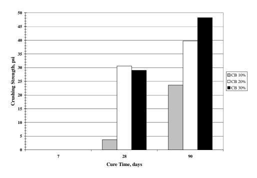
Figure 89. Strength gain of Le Grand loess stabilized with CB HFA
