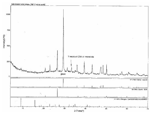
Figure A.16. X-Ray diffractogram for CB hydrated fly ash
