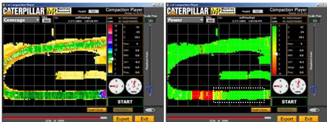
Figure 20. Topsoil, strip 4 compaction monitor views (30 x 24 m viewing area)
