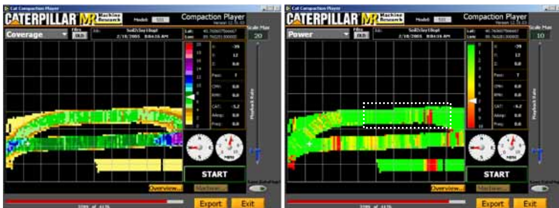
Figure 25. Fill clay, strip 3 compaction monitor views (30 x 24 m viewing area)
