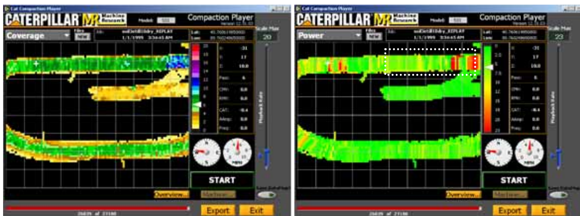
Figure 27. Edwards till, strip 2 compaction monitor views (30 x 24 m viewing area)
