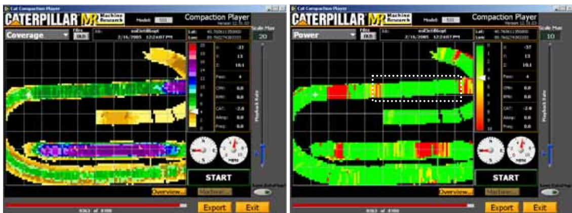
Figure 30. Edwards till, strip 6 compaction monitor views (30 x 24 m viewing area)
