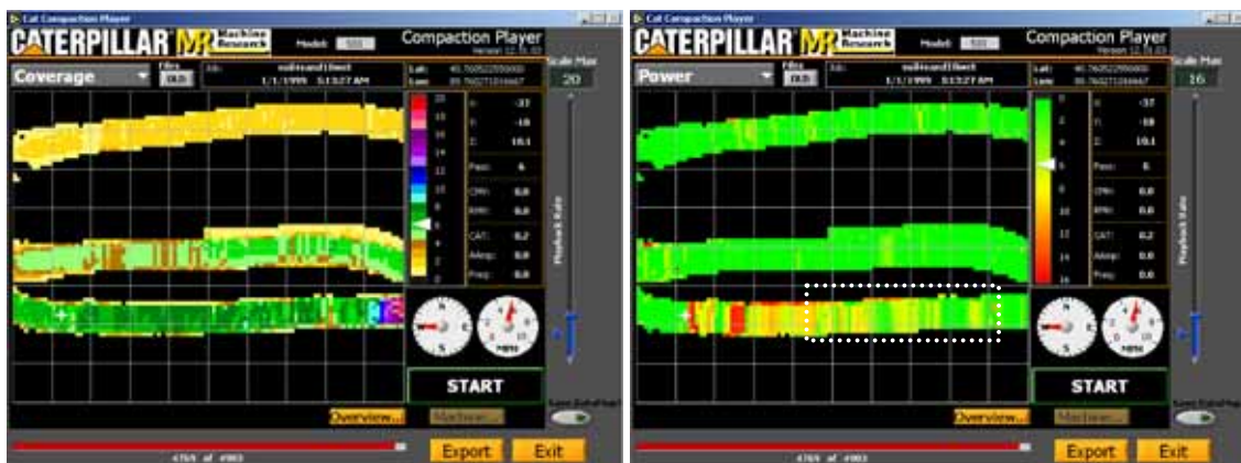
Figure 34. Sand, strip 4 compaction monitor views (30 x 24 m viewing area)
