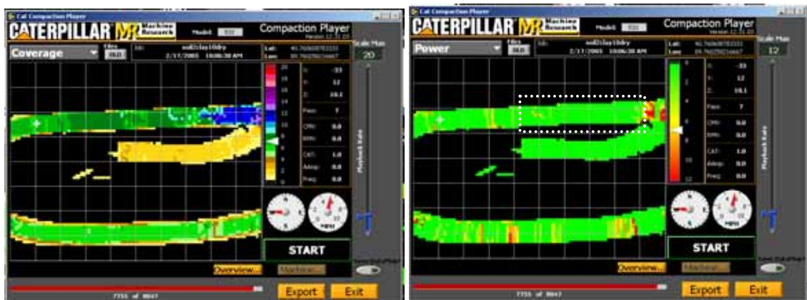
Figure 24. Fill clay, strip 2 compaction monitor views (30 x 24 m viewing area)
