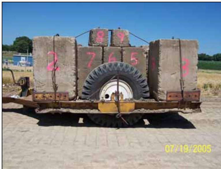
Figure 172. Test roller used for quality assurance
