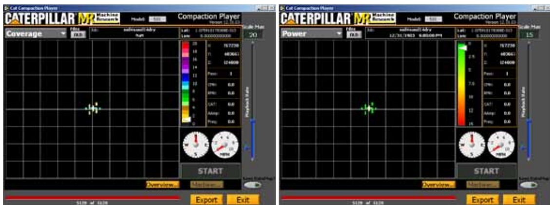
Figure 32. Sand, strip 2 compaction monitor views (30 x 24 m viewing area)
