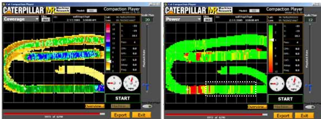
Figure 19. Topsoil, strip 3 compaction monitor views (30 x 24 m viewing area)
