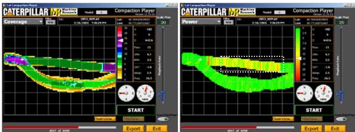
Figure 158. CA6, strip 2 compaction monitor views (30 x 24 m viewing area)
