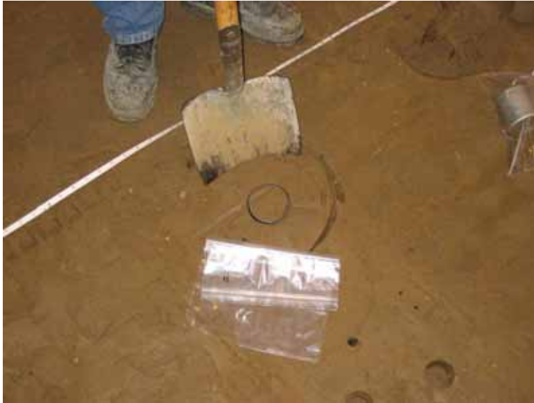
Figure 12. Excavation of drive core for density and moisture determination
