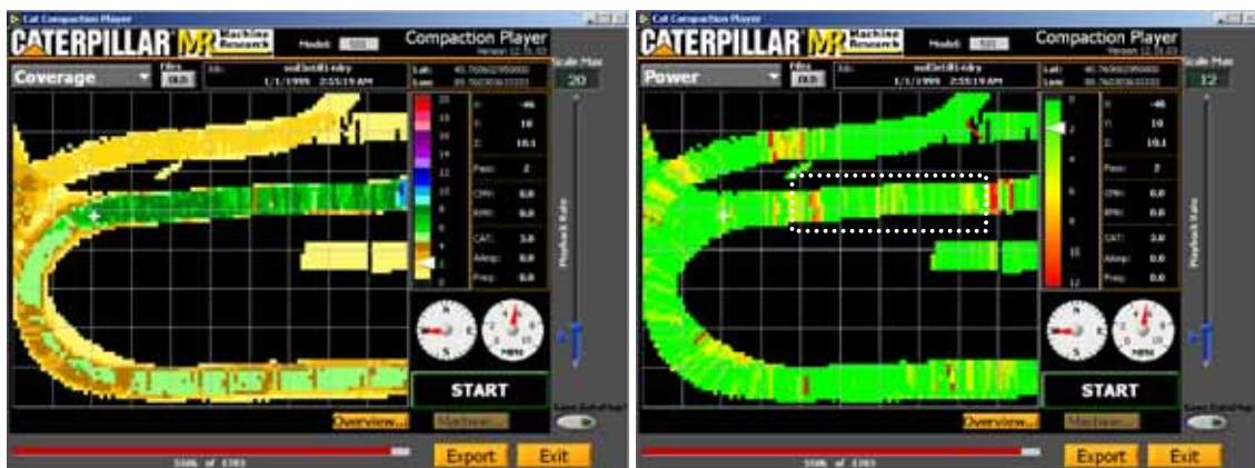
Figure 26. Edwards till, strip 1 compaction monitor views (30 x 24 m viewing area)
