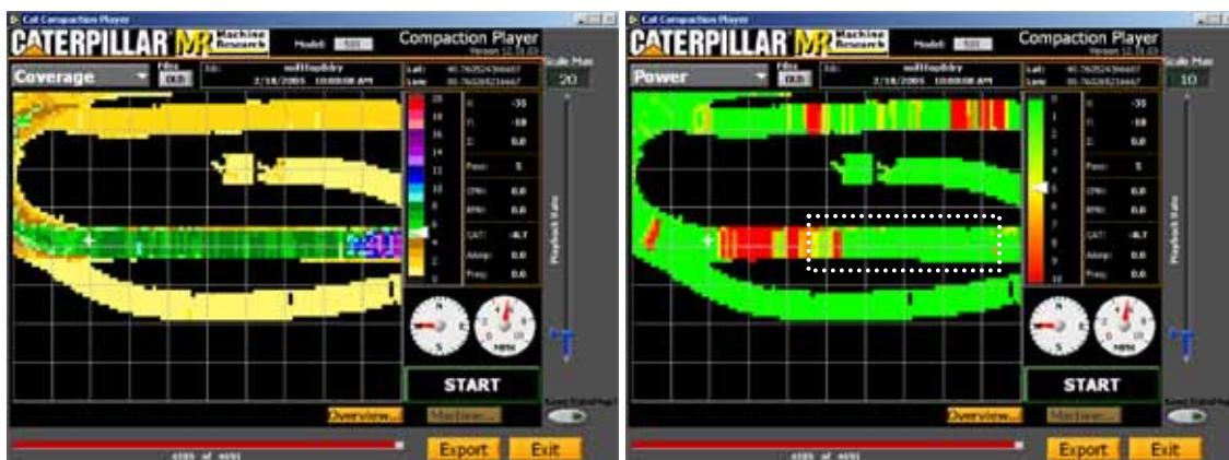
Figure 22. Topsoil, strip 6 compaction monitor views (30 x 24 m viewing area)
