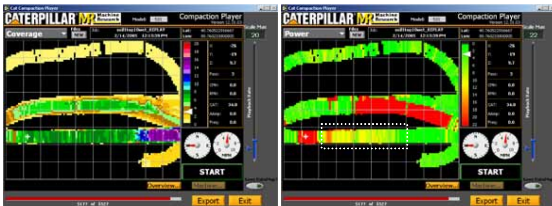
Figure 18. Topsoil, strip 2 compaction monitor views (30 x 24 m viewing area)
